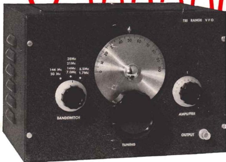
The slogan to remember when building oscillator tank circuits is "Keep 'em cool and solid, OM!" By placing the tubes outside the box, W2RMM does just that with this versatile VFO which covers three ranges to multiply into all popular amateur bands.
