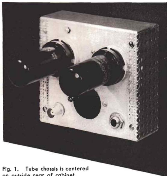
Fig. 1. Tube chassis is centered on outside rear of cabinet.
