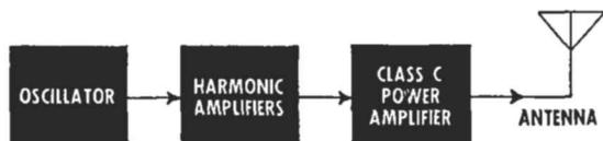
Fig. 1. Block diagram of a typical multi-stage transmitter to which a CW or AM system may be connected.
