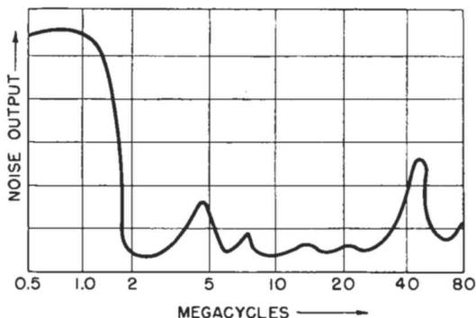
This particular curve represents the noise spectrum of a typical 40-watt fluorescent lamp. Lamps having different wattage ratings usually will have peaks of noise output at other frequencies.
