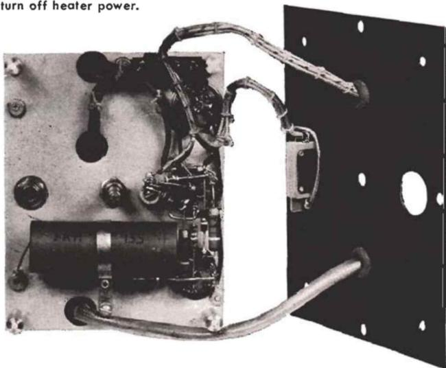
Fig. 10. Layout and construction details of the Mobile Modulator. The 12AT7 voltage amplifier is the shielded tube at the bottom next to the microphone transformer, T<sub>1</sub>.
