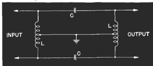
Fig. 7. Schematic diagram for the TVR High-Pass Filter. Capacitors C are 12-mmf general-purpose ceramics. Coils L are 1.08  $\mu$ h, 23 turns, No. 30 enameled wire on a  $\frac{1}{8}$ -inch diameter form. (See text for coil winding details.)
