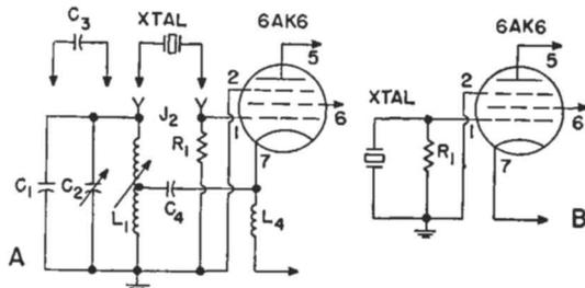
Fig. 4. Alternate oscillator grid circuits for (A) both crystal controlled and VFO operation, and (B) crystal controlled operation only, eliminating  $C_1$ ,  $C_2$ ,  $C_3$ ,  $C_4$ ,  $L_1$  and  $L_4$ .
