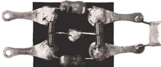
Fig. 8. Construction details of the TVR filter.
