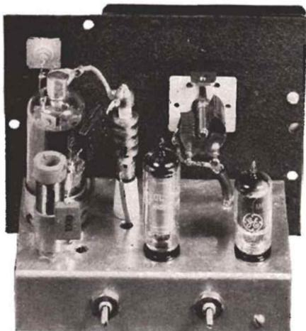
Fig. 5. Back view of the E-P Rig. Coils  $L_1$  (right) and  $L_2$  (left) are tuned through holes in the cabinet rear plate. The GL-2E26 plate coil,  $L_3$ , mounts directly behind this tube.
