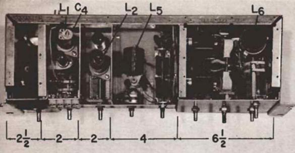
**TOP VIEW** of the r.f. unit with shield covers removed. Note shielding partitions between stages and horizontal mounting of 6146 tubes on shield to isolate grid and plate circuits in the balanced modulator output stage. Main chassis is a 5/4-inch high panel chassis designed for relay rack mounting (Bud CB-1372, or equivalent).
