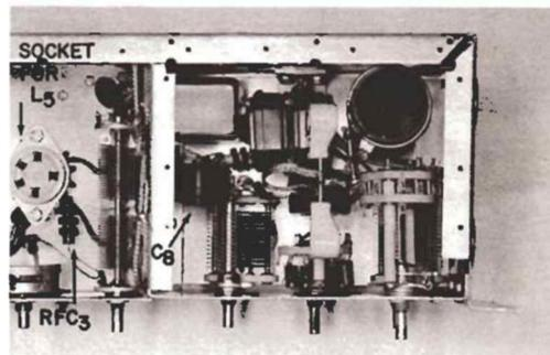
**TOP VIEW** of the 6146 compartment showing the positions of smaller components near the switches, capacitors and coils. The bandswitch,  $S_2$ , was modified by adding longer side rods and spacers to shorten the connections to  $L_6$ . This compartment was assembled before being fastened to the main r.f. chassis.
