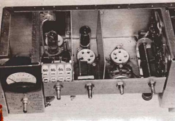
**DETAIL VIEW** of the wiring around the 6146 balanced modulator tube sockets. The standard technique of bypassing the ends of shielded wire has been used. The 6146 plate caps were joined with No. 12 tinned wire, then connected with thin copper strips to the circuit components shown in the schematic diagram, FIG. 1.
