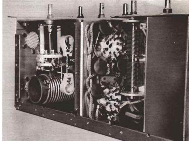
**EXCITER COMPARTMENTS** in the r.f. unit. Plug-in coils have been removed to show the coil sockets mounted on metal pillars  $\frac{3}{4}$  of an inch high. All partitions and shelves were fabricated from 1/16-inch thick soft sheet aluminum. The crystal sockets were mounted on a bracket drilled to match the socket holes.
