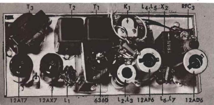
**REAR VIEW** of the center chassis. Note the r.f. shield between the 6360 tube and the 12AT7 oscillator tube. The cabled leads at the top of the picture run to the parts and controls on the front panel. Power connections to  $P_1$  on the cabinet are included in this cable. The antenna lead runs directly from relay contacts  $K_{1A}$  to  $J_2$  on the rear panel.
