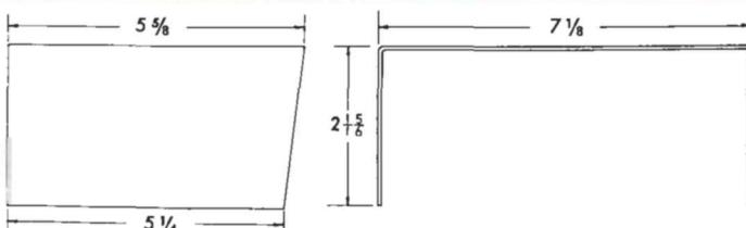
**FIG. 5. HOODED COVER** which can either be installed on the commercially made cabinet, or on a home-made cabinet. A piece of  $\frac{1}{8}$ -inch thick sheet aluminum,  $13\frac{1}{4} \times 5\frac{5}{8}$  inches over-all, is required.
