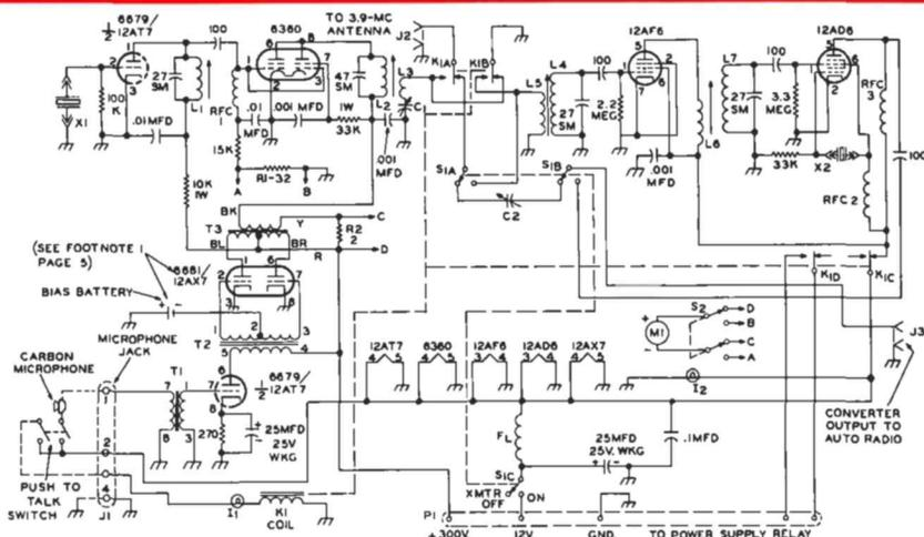
**FIG. 1. SCHEMATIC DIAGRAM** of the TC-75 transmitter/converter. The transmitter and modulator are at the left; and the crystal-controlled converter is at the right. Capacitors are in mmf, unless otherwise noted; silvered micas are marked "SM." Resistances are in ohms (K = 1000), 1/2 watt rating if not marked 1 watt, or 2 watts.
