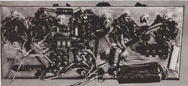
FRONT VIEW of the center chassis, showing the wiring and placement of small parts around the tube sockets. The nine terminals on T<sub>1</sub> and T<sub>2</sub> can be seen through the 3/4 x 3/4-inch square cutouts in the chassis for these components.
