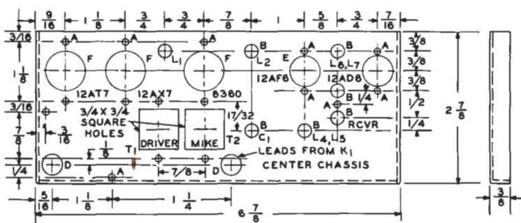
**FIG. 2. DRILLING DIAGRAM** for the center chassis. All holes sizes identified on the diagram by letter are given in TABLE II. Over-all size of the aluminum sheet should be  $7\frac{3}{4} \times 3\frac{5}{16}$  inches, to allow for the  $\frac{3}{8}$ -inch wide lips, plus bends.
