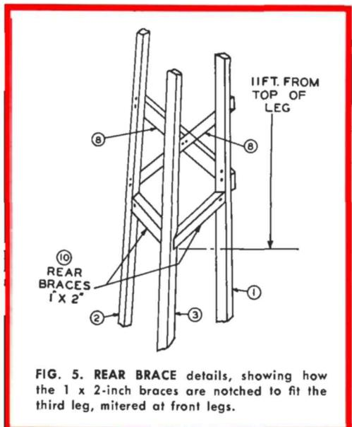
FIG. 5. REAR BRACE details, showing how the 1 x 2-inch braces are notched to fit the third leg, mitered at front legs.
