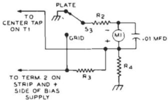
The plate current metering circuit for the GL-813 KILOWATT GROUNDED-GRID LINEAR AMPLIFIER (See G-E HAM NEWS, November-December, 1959, Fig. 1, page 4) should be connected as shown above. Complete details are available in a bulletin, which also has additional construction and component information.
