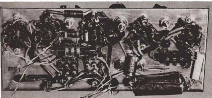
**FRONT VIEW** of the center chassis, showing the wiring and placement of small parts around the tube sockets. The nine terminals on  $T_1$  and  $T_2$  can be seen through the  $\frac{3}{4} \times \frac{3}{4}$ -inch square cutouts in the chassis for these components.
