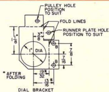
FIG. 10. DIAGRAM showing how the brackets on which C<sub>1</sub> is suspended below the chassis are formed and drilled, using 1/16-inch sheet stock. The dimensions and holes fit the Hammarlund MCD-100-S RF tuning capacitor used on this model.
