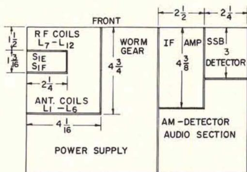
FIG. 6. SHIELD PARTITION locations inside the main chassis. An "L" shaped shield encloses the entire RF coil section, with a small "U" shaped shield in the middle of the bandswitch. A straight shield runs from the front to the back of the chassis alongside the IF amplifier, and a small straight shield runs from this to the side of the main chassis.
