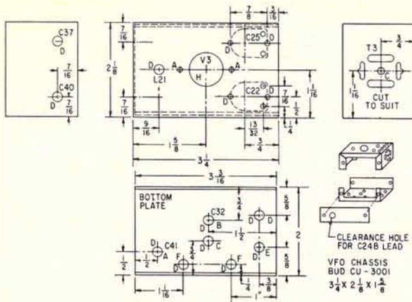
FIG. 4. VFO SUBCHASSIS layout diagram. Holes in bottom plate marked "A" through "F" are for small feedthru bushings (National TPD), and C<sub>32</sub> and C<sub>41</sub>. They should be drilled through the main chassis to allow connections to be made below the chassis.
