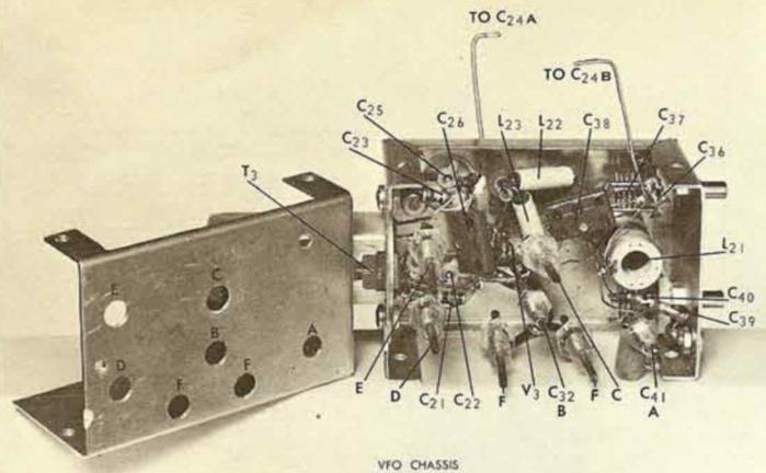
INSIDE VIEW of VFO-second mixer (V<sub>3</sub>) subchassis with bottom cover plate (at left) removed. Machine screws on both sides of first IF transformer (T<sub>3</sub>) are for grounding lugs on inside of box to which grounded ends of C<sub>22</sub> and C<sub>25</sub> are connected. Note that opening is cut in one side of bottom cover for cover plate which provides access to inside of VFO box after it is installed on chassis of receiver.
