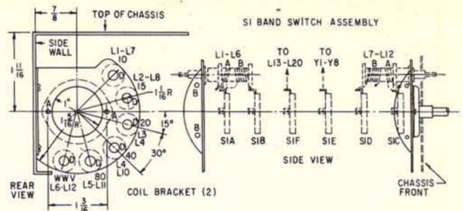
FIG. 8. BANDSWITCH ASSEMBLY, showing the positions of the switch wafers and coils. The brackets on which the RF coils (L1 to L6, and L7 to L12) are mounted are cut as 2 5/8-inch diameter circles from 1/16-inch thick sheet aluminum, then drilled, trimmed and bent as shown.
