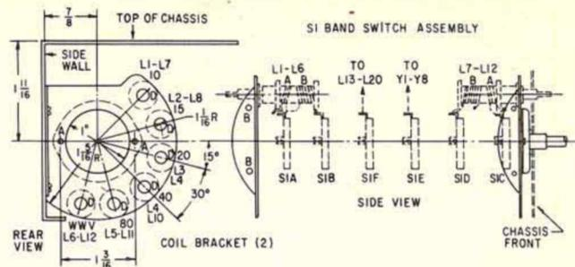
FIG. 8. BANDSWITCH ASSEMBLY, showing the positions of the switch wafers and coils. The brackets on which the RF coils (L<sub>1</sub> to L<sub>6</sub>, and L<sub>7</sub> to L<sub>12</sub>) are mounted are cut as 2 5/8-inch diameter circles from 1/16-inch thick sheet aluminum, then drilled, trimmed and bent as shown.
