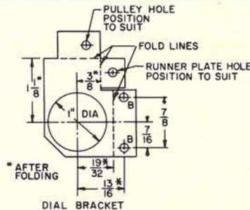
FIG. 10. DIAGRAM showing how the brackets on which C1 is suspended below the chassis are formed and drilled, using 1/16-inch sheet stock. The dimensions and holes fit the Hammarlund MCD-100-S RF tuning capacitor used on this model.
