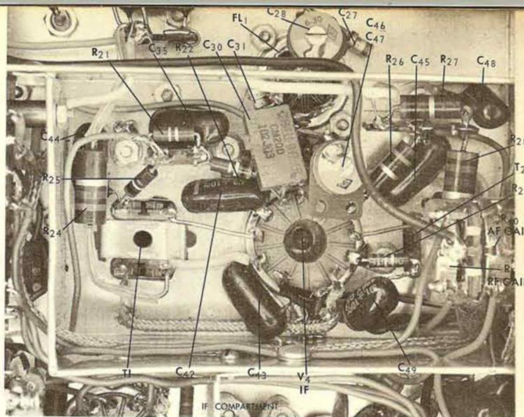
CLOSEUP VIEW OF the 455-kilocycle second IF amplifier ( $V_4$ ) compartment. The neutralizing capacitor ( $C_{46}$ ) which assures stable operation is on the 12-pin compactron tube socket. Note the shield partition running across the 9-pin miniature tube socket for  $FL_1$ .
