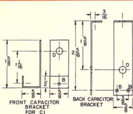
FIG. 9. BRACKETS supporting the dial scale tubing are formed using this diagram as a guide.
