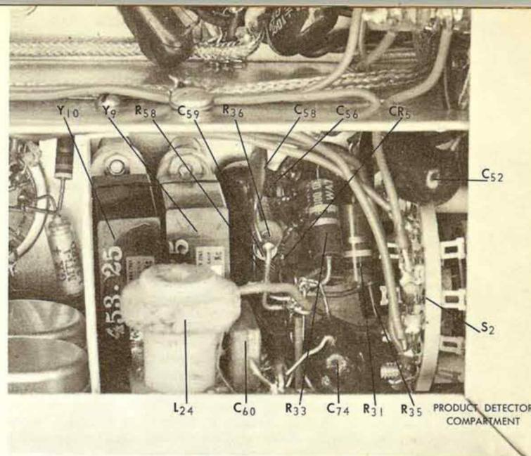
PRODUCT DETECTOR section (V<sub>8</sub>) is detailed in this view of the front right-hand corner of the receiver.
