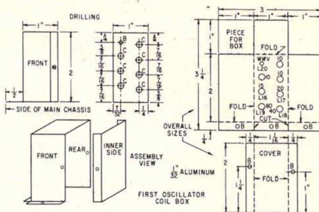
FIG. 5. FORMING AND DRILLING diagrams for the first oscillator coil box which houses L<sub>13</sub> to L<sub>20</sub> on the chassis of the receiver. Holes for the coils are drilled after folding the main piece. Matching holes for No. 6-32 machine screws are drilled into the main chassis.
