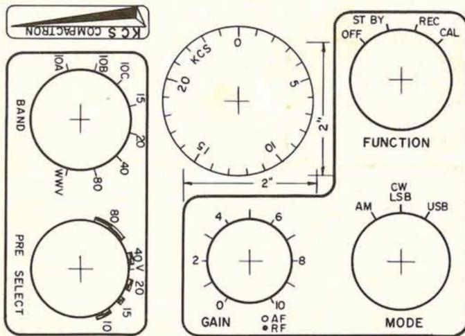
FIG. 16. CONTROL MARKINGS used on the KCS receiver, shown half size. Halmar Electro-Kit name plate process<sup>2</sup> was used to make up marking plates on the model receiver.
