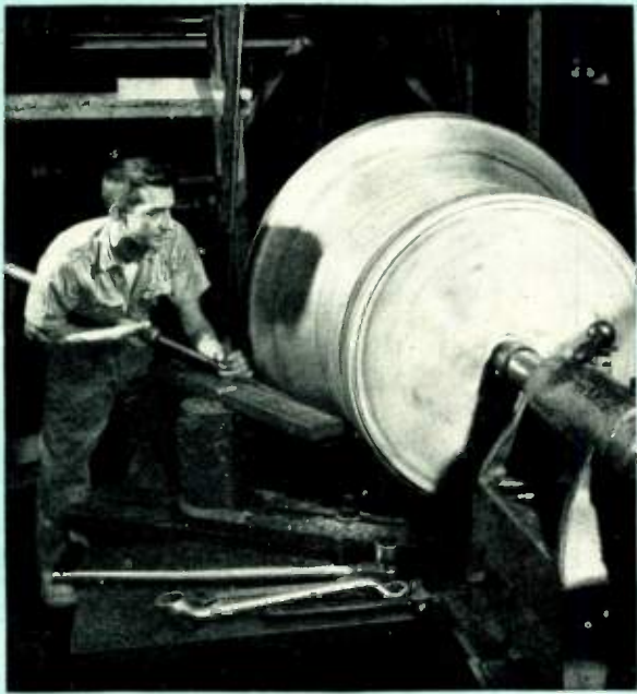
Building jet engines requires special skills, like spinning stainless steel parts. Jobs like this are expertly done by the Roland Teiner Co., in Everett, Mass.
