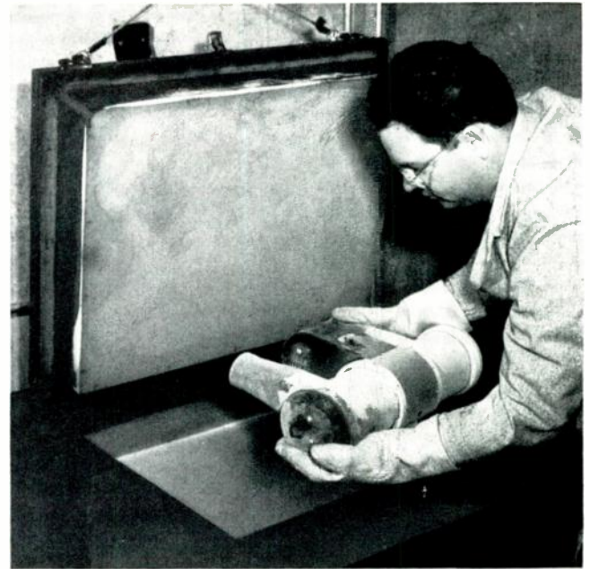
Frost covers the casing of the military x-ray unit made by the X-Ray Department as engineer Reimann Stroble lifts it from a refrigerator where it has withstood temperatures as low as -50^{\circ} F. Following a thawing-out process the tube was operated to determine whether the extreme cold had had any effect on its operating efficiency. This climatic test is only one which the tube must undergo in order to be sure that it will withstand the rugged transportation and storage conditions of military service. It is also given a "heat test" during which it operates at temperatures up to 125^{\circ} F.
