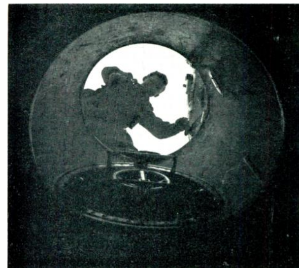
In groups of three the crew can escape through this hatch. They seal themselves in, partially flood the chamber, open the outer door and escape.
