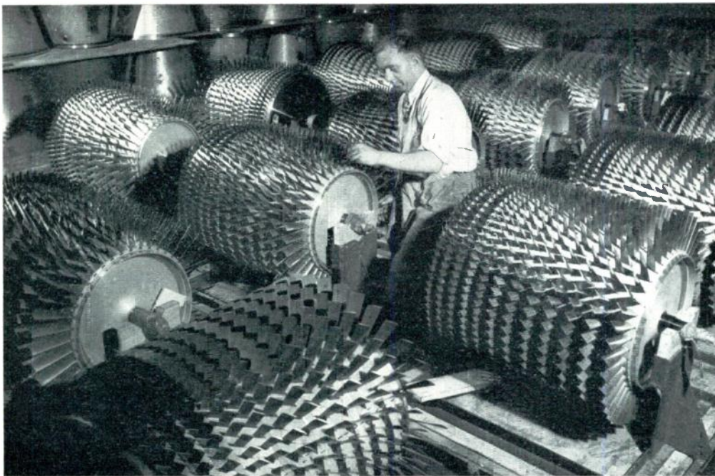
The first chapter in the jet story was written long before the first jet flight. Without years of research and development on rotors for steam turbines, these rotors for aircraft jet engines might never have been built.
