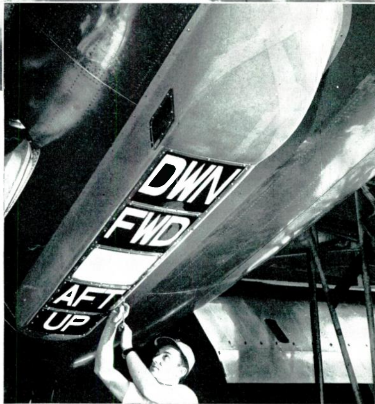
A directional lighting system is installed on a Boeing B-29 tanker to help in the job of refueling bombers in mid-air (top photo). Special sealed beam lamps were developed by the Lamp Division for this purpose. Red and green lights are automatically triggered by microswitches connected with the boom.
