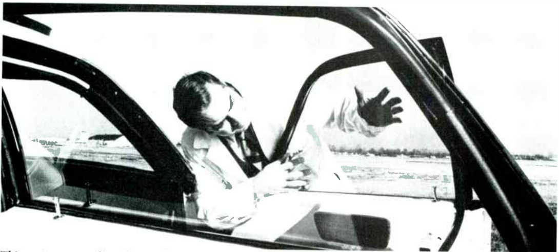
Things to come: the side windows of an experimental safety vehicle developed for the Department of Transportation by Fairchild's Republic Division are made from General Electric's Lexan® MR-4000 sheet. The plastic glazing material is strong enough to keep passengers from being thrown out should an accident occur, yet flexible enough to "give" on impact, thus reducing the chance of injury. ☐
