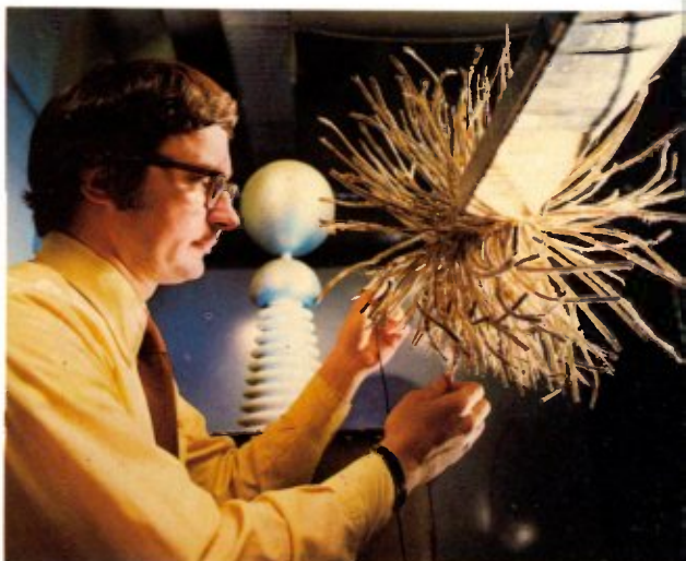
Schenectady's Materials and Processes Laboratory includes three Centers of Research, including work on high-voltage insulation systems such as this developmental strand insulation.
