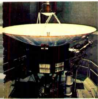
Voyager. Just starting their 12-year mission, NASA's two Voyager spacecraft are each carrying three GE Multi-Hundred Watt Radioisotope Thermoelectric Generators, which will power each craft's 10 scientific experiments.
