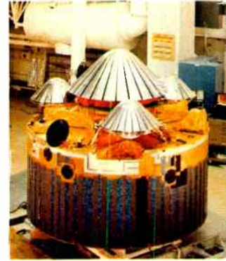
Pioneer Venus. When NASA's two Pioneer spacecraft approach Venus in late 1978, one craft will eject four GE deceleration module probes to collect information on the atmosphere.
