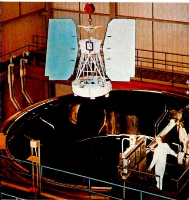
Nimbus. A GE "weather bird" undergoes space environment simulation tests. GE has built six such craft, and a seventh will be launched next year. In 1969, Nimbus spotted Hurricane Camille and is credited with saving thousands of lives.
