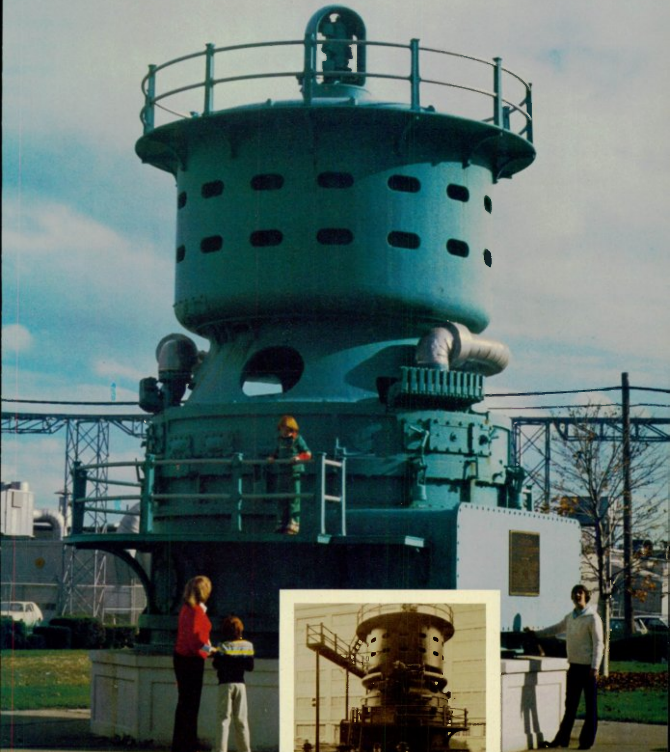
The 5,000-KW Curtis steam turbine of 1903 on display at Schenectady-GE. A national historic engineering landmark, it was viewed by Edison, Steinmetz and Rice in 1922 (inset).
