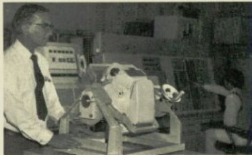
A. Trident's "brains": GE inertial measurement unit is examined by Ordnance's Roy Wiley.
