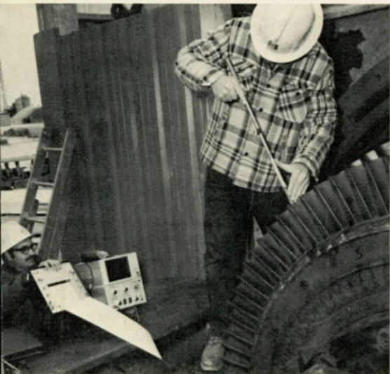
To provide customers with timely turbine maintenance, I&SE monitors turbine operations (above) using new eddy current inspection procedure. I&SE personnel (right) rebuild irradiated control rod drive units during nuclear plant refueling outage.
