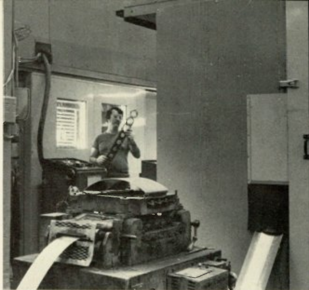
Shielding Fort Wayne GE employees from loud workplace noises are sound-dampening enclosures for automatic-feed-lamination punch presses.
