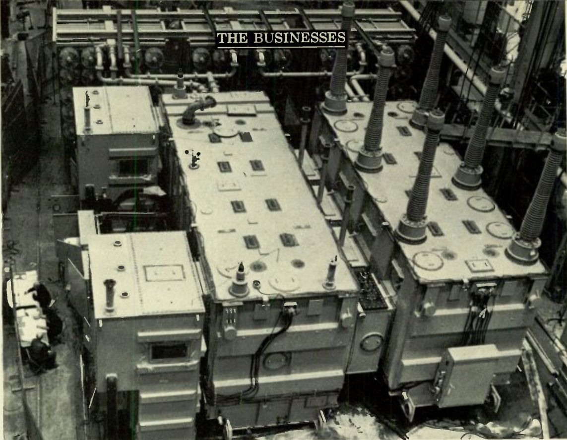
To help reduce the probability of power blackouts: a 2.1-million-pound GE phase shifter transformer.
