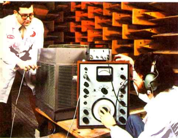
Research shaping tomorrow’s major appliances involves, left, noise measurements in anechoic room and, right, evaluation of new dishwasher tub coatings exposed to hot water vapor test.
