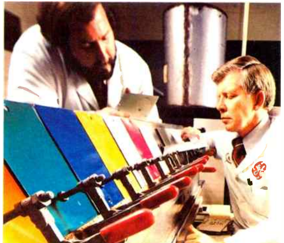
Research shaping tomorrow’s major appliances involves, left, noise measurements in anechoic room and, right, evaluation of new dishwasher tub coatings exposed to hot water vapor test.
