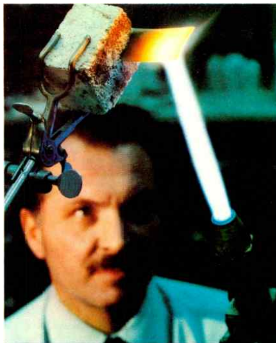
Scientists study fabrication of silicon carbide heat-resistant materials (above); large family of GE silicone products grew from 1940 research on a direct process (below).
