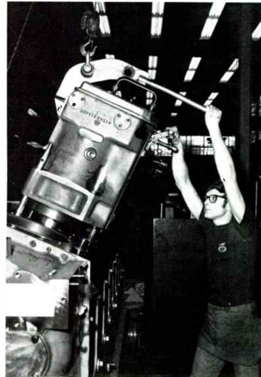
Some 5000 General Electric diesel engines are now in operation. In Erie's main assembly area, grinder Randy Strickenberger grinds an engine's main connecting rod, while assembler Rick Pheasant lowers unitized cylinder into place.
