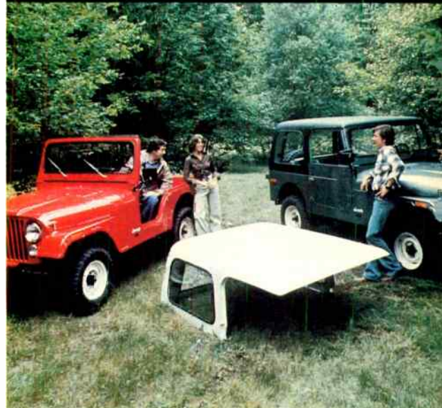
Dr. Daniel Fox (above), inventor of supertough Lexan® polycarbonate resin. Today, Lexan Structural Foam reduces jeep weight by substituting for its heavier metal top (below).
