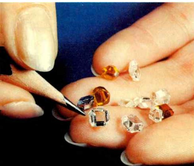
Man-Made® diamonds (1955) and synthesized gem diamonds (1970—above) by GE researchers (below) ended a centuries-long quest to duplicate nature's hardest substance.
