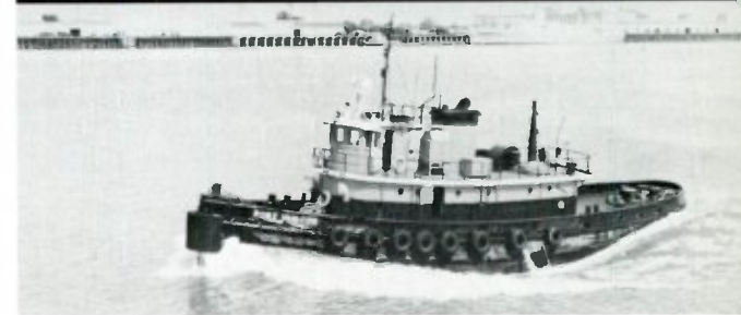
General Electric's marine diesel business began eight years ago. Among early GE projects: fishing vessel Enterprise (top), originally purchased for Del Monte tuna fleet, propelled by one diesel engine; Crescent Towing and Salvage's tugboat Port Hudson (below), also powered by one diesel engine; and Reading & Bates' drill ship Douglas Carver , with three diesel-electric power modules.
