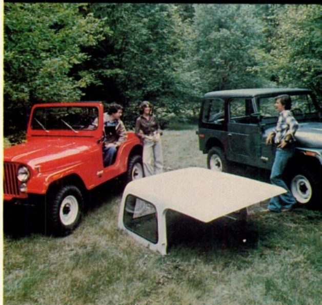
Dr. Daniel Fox (above), inventor of supertough Lexan® polycarbonate resin. Today, Lexan Structural Foam reduces jeep weight by substituting for its heavier metal top (below).
