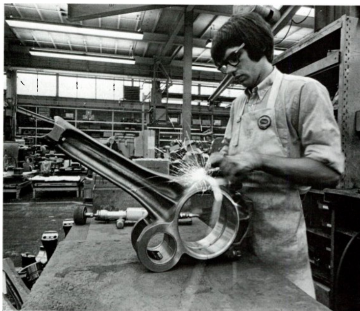
Some 5000 General Electric diesel engines are now in operation. In Erie's main assembly area, grinder Randy Strickenberger grinds an engine's main connecting rod, while assembler Rick Pheasant lowers unitized cylinder into place.
