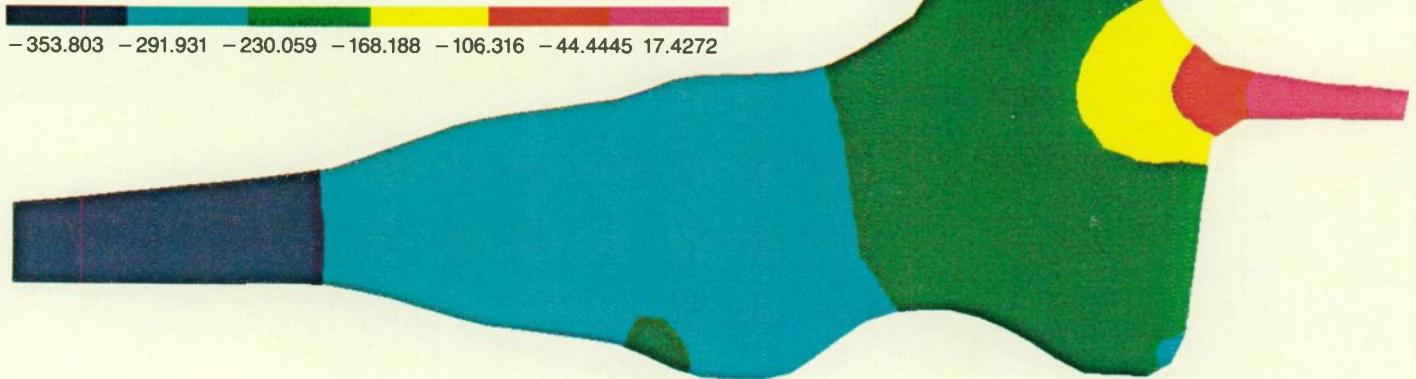
Figure 6 Ladish Stage One Disk—Finisher Element Hydrostatic Pressure Assigned To Nodes
