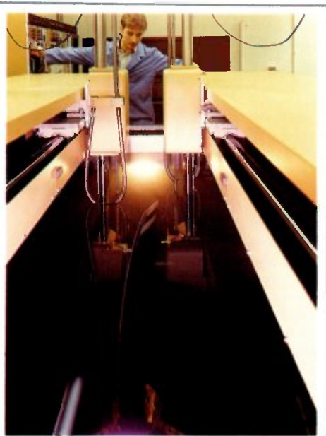
On the cover. Ultrasonic C-scan of UDF™ blade.
