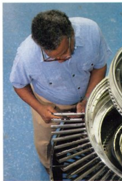
Leaman Houston assembles blades into the inner rotor of the UDF power turbine.
