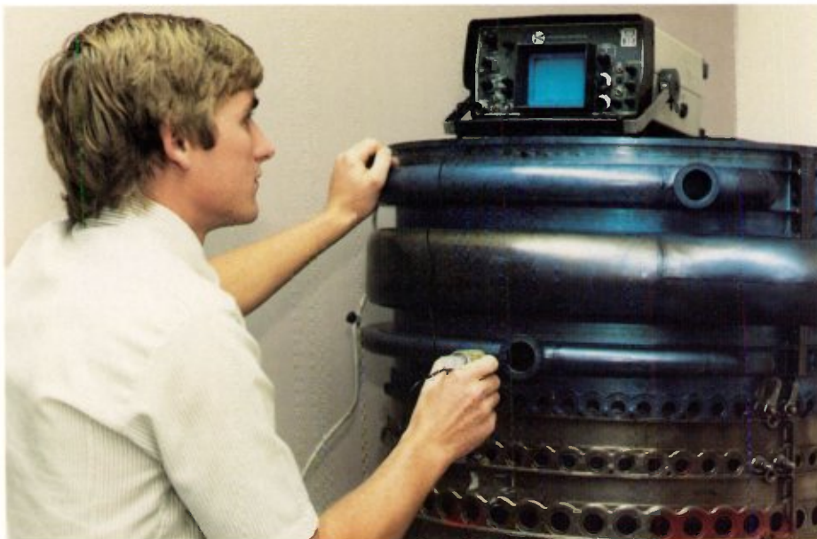
NDE Technician John Dierdorf proof-tests what will soon be an on-wing ultrasonic inspection technique.
