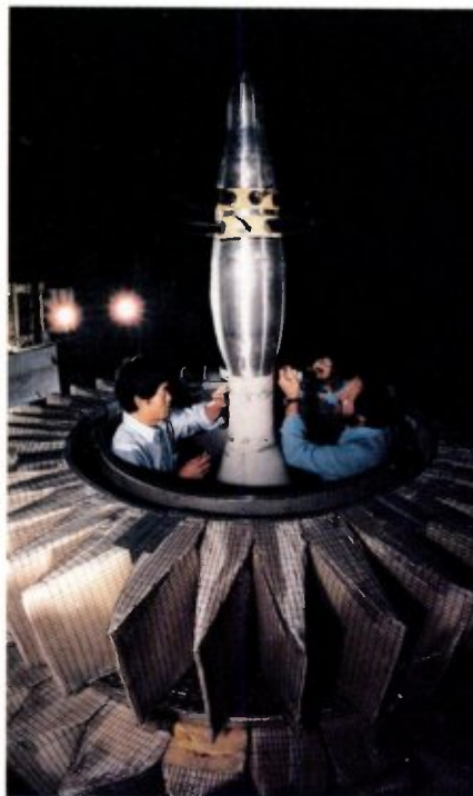
Dave Chi (left) and Dan Kavanagh make last minute adjustments to the scale model UDF rig before test in the anechoic chamber at Evendale.
