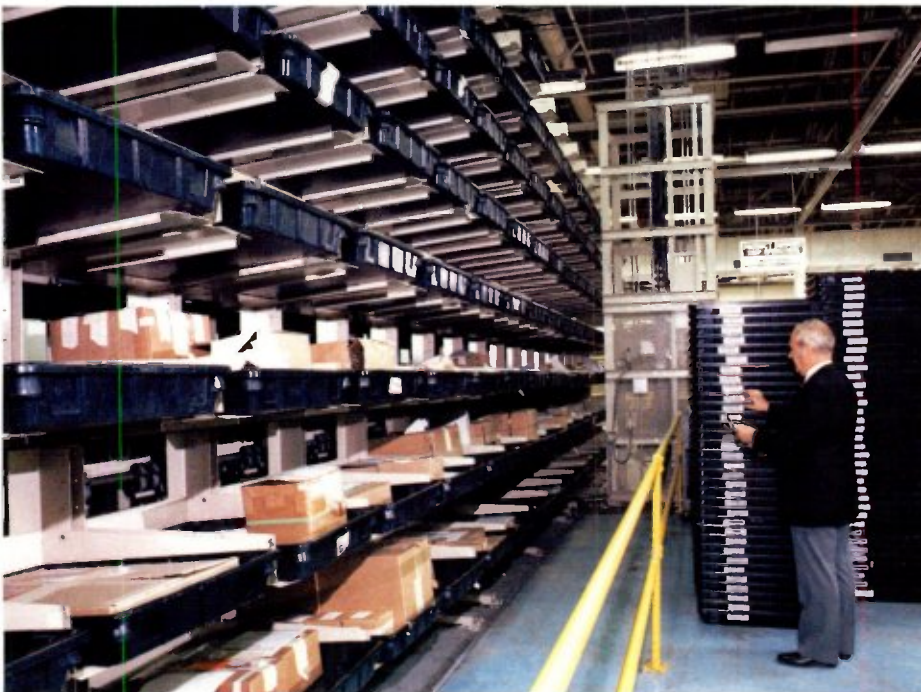
Al DesMarais verifies bar-coded labels on material handling trays as the robot in the background loads incoming parts onto the carousel for storage.
