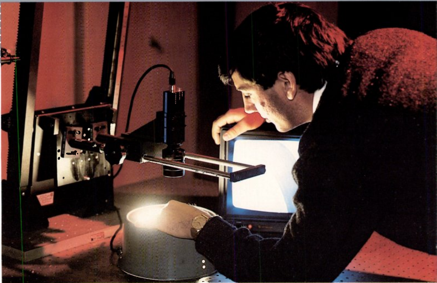
Engineering co-op Doug Beitch positions a light fixture on an optical bench for thickness measurement of a CFM-56 blade.
