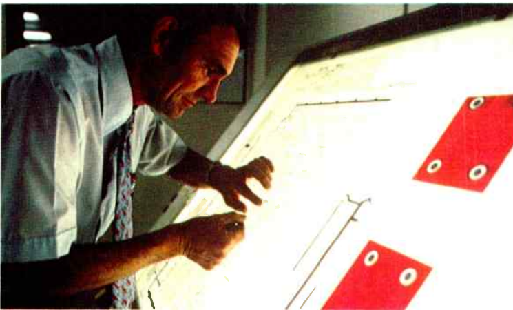
This artwork is used to make a printed circuit board at Intersil.
