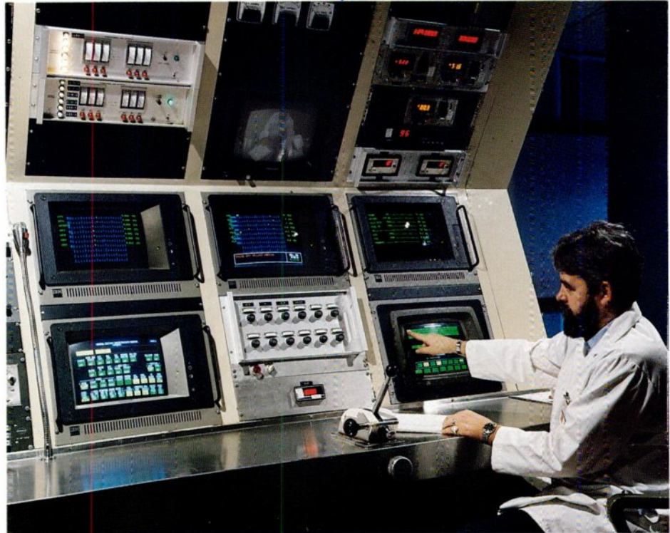
Using touch screens like this one in cell 105 is faster and less error-prone than typing
