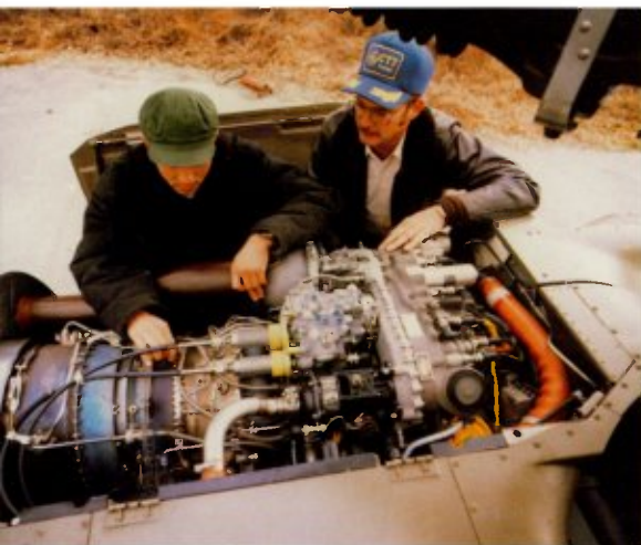
CT7, a commercial version of the T700, was developed in 1980 as an advanced turboprop. It was certified in 1983 and by the end of the decade 150 were in service.
