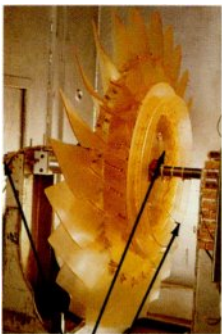
Figure 7A. Photoelastic model showing F118 slip ring assembly with embedded thick/thin location thermocouples.
