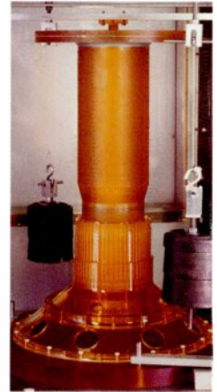
Figure 8. Loading rig for torsional stress-freezing static test of fan shaft spline coupling.
