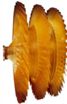
Figure 3. Using photoelastic techniques, stress magnitudes and distributions were obtained for all three stages and the rear shaft of this three-stage fan rotor assembly model of the F110.
