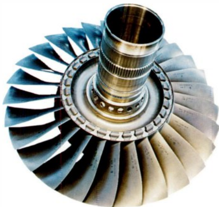
Figure 3: The high pressure compressor's stage one disk features a steel design to enhance durability
