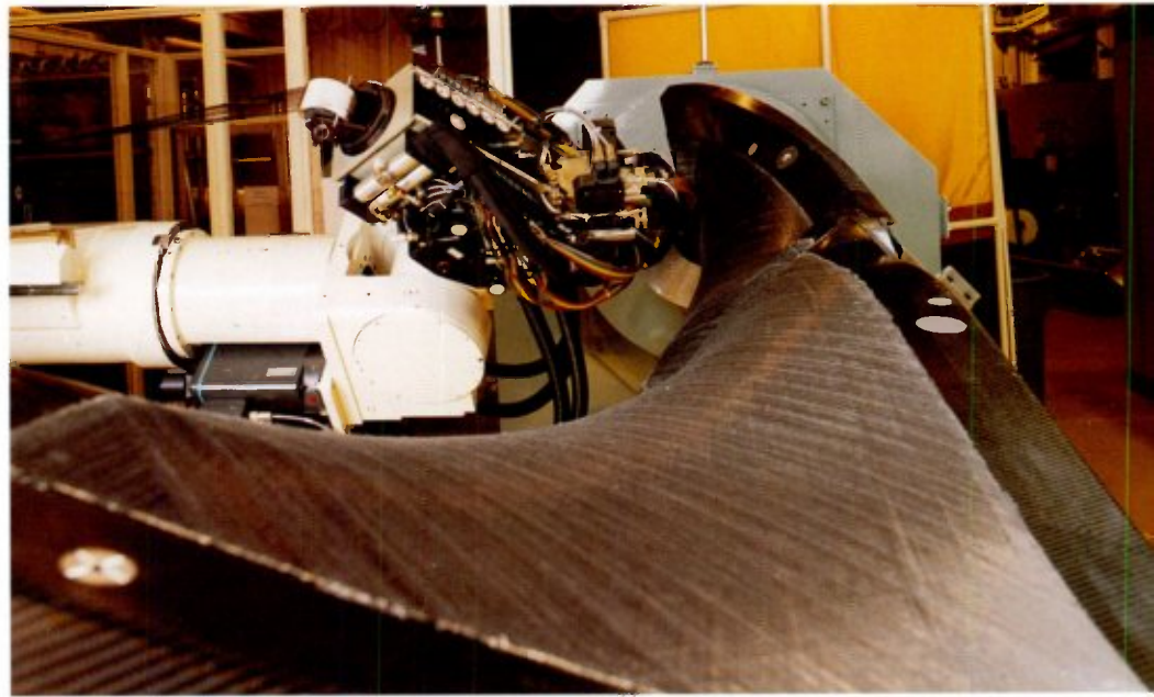
Figure 3: Robotic techniques being adapted by GE Aircraft Engines and Cincinnati Milacron will replace manual manufacturing methods for GE90 fan blades
