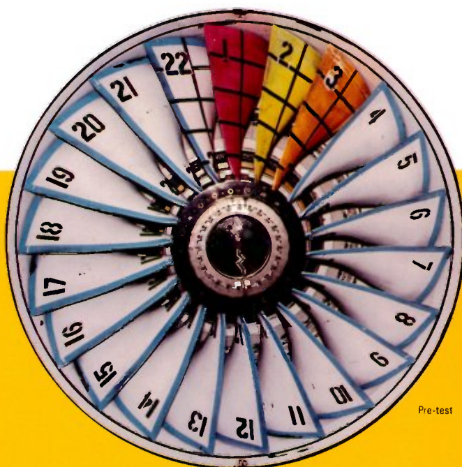
Figure 5: Fan bladeout imbalance and secondary impact forces were within predicted levels, proving blade and retention design adequacy
