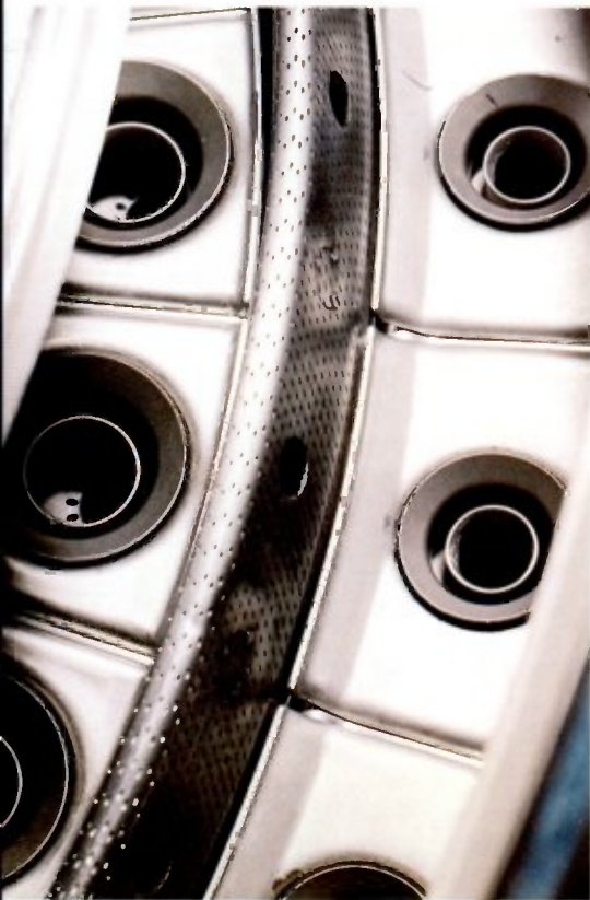
Figure 1: GE90's dual annular combustion system blends the characteristics of two different combustors, each optimized for different operating regimes
