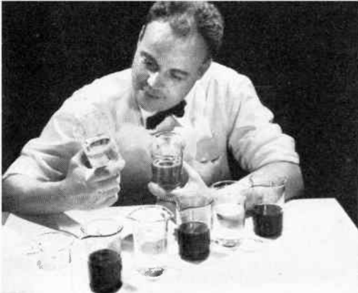
SILICONE LUBRICANT stays clear at high heat.
