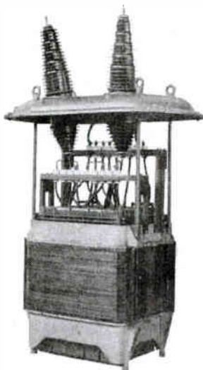
Transformer Removed from Case
