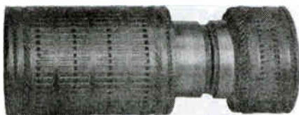
Fig. 4. Generator and Exciter Armatures Mounted on Same Shaft
