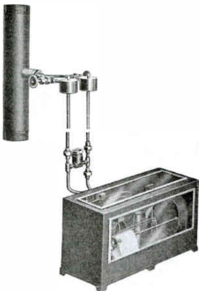
Fig. 2. Recording Steam Meter, Showing Connections to Pipe
