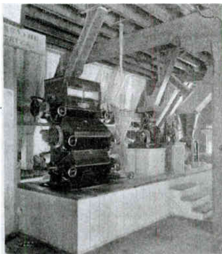
Grit Mill Machinery which is Driven by a 25 H. P. Motor Housed in a Separate Building
