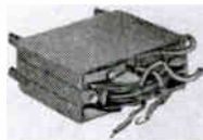
Fig. 10. Transformer of Quarter Century Ago.
