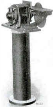
Fig. 3. 1 H.P. Induction Motor with Dowel Cutting Saw Mounted on Motor Shaft
