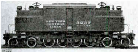
Fig. 3. Locomotive Used in the New York Central Electrification at New York
