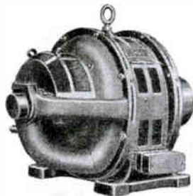
Fig. 4. 6 H.P. 500 Volt Slip Ring Induction Motor. This Motor Caused Ignition of Surrounding Gases, Owing to Large Openings Between the Feet and to Wire Gauze of too Large Mesh
