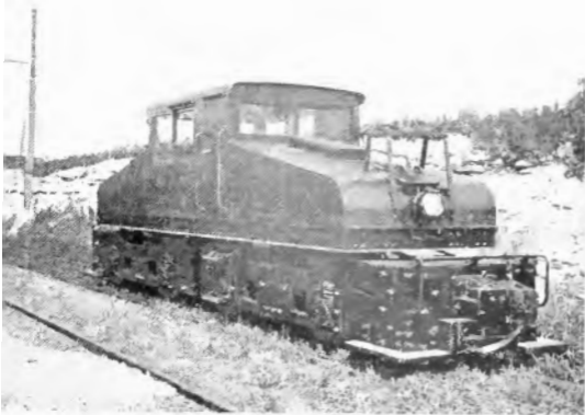
Fig. 14. 40-ton Haulage Locomotive Built for the Britannia Mining & Smelting Co.
