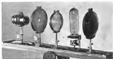
Fig. 69. Motion picture Lamp and Accessories—Experimental Equipment Showing Mazda C Lamps and Optical Train. In the commercial outfits these parts are concealed from view by the housing
