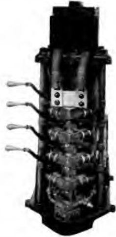
Fig. 28. Electric Rivet Heater, Front View, Showing Rivet Holding Jaws
