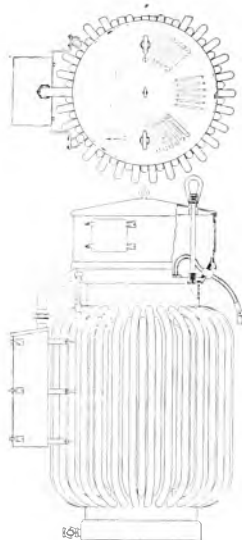
Fig. 34. Induction Regulator, Automatic, Self-control Outdoor Type
