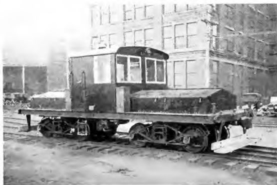
Fig. 15. 20-ton Standard Gauge Storage Battery Locomotive Built for Newport News Shipbuilding & Drydock Co.
