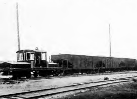
Fig. 16. 20-ton Storage Battery Locomotive Used for General Freight Car Shifting
