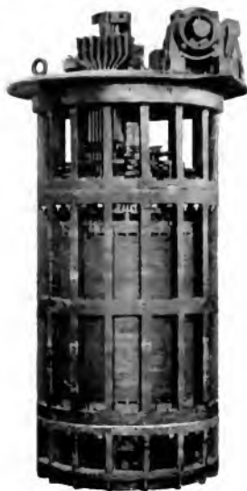
Fig. 36. 770-kv-a. Induction Voltage Regulator Showing Internal Arrangement
