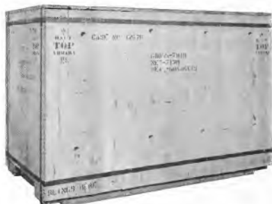
Typical Packing Case for Export Shipment. Note banding iron, breathing holes protected with wire netting to exclude mice, "Haut Top Arriba" and arrows to indicate top of box, and notched lower corners to accommodate slings
