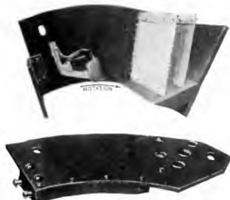
Fig. 6. Flash Barrier for Direct-current Machines
