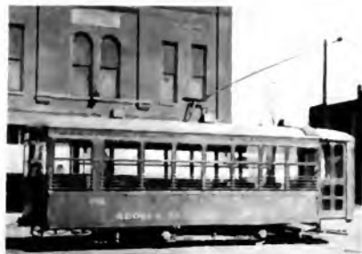
Fig. 11 Light weight Safety Car Equipped with GE-258 Motors Keokuk Electric Co
