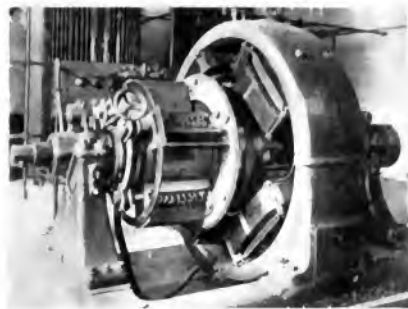
Fig. 7. 500 kv.a., 400 volt Synchronous Converter Equipped with Flash Barriers
