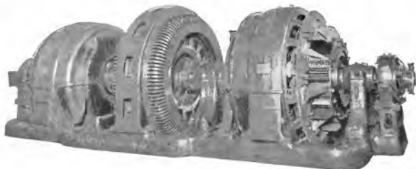
Fig. 8. One of the Eight 2000 kw., 3000-volt, Three unit Synchronous Motor generator Sets Under Construction for the Chicago, Milwaukee & St. Paul Railway, Othello, Seattle & Tacoma Division. Twenty-three similar sets are in service on the original electrification from Harlowton to Avery
