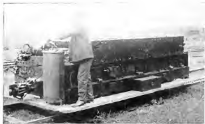
Fig. 18. 12-ton Storage Battery Locomotive Used for Yard Shifting and Provided with Special Footboard
