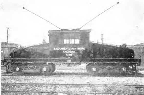
Fig. 13. 60-ton Electric Locomotive Built for Sacramento & Northern Railroad
