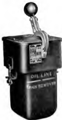
Fig. 44 Triple pole, Single throw, 600 volt, 30-ampere Oil Circuit Breaker, Type FP 15
