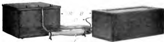
Fig. 4. Assembly of Apparatus for Measuring Crest Voltage from Volt Coil B , Instrument Case; D , Cable to Resistance; R , Resistance Box; E , Filament Current Resistance.
