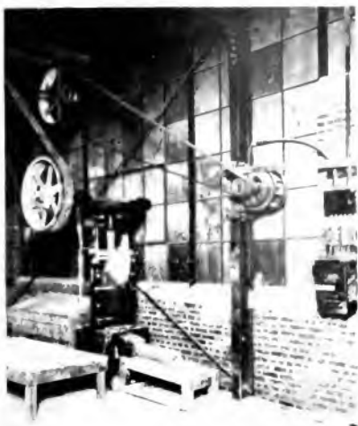
2 h.p., 900 r.p.m. Induction Motor Operating a Mueller Company's Pug Mill, Imperial Porcelain Company, Manasquan, N. J.
