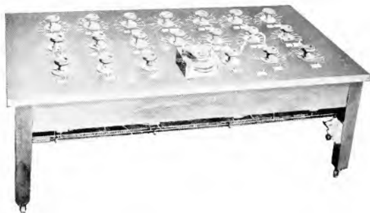
Fig. 3. Table Showing Method of Mounting Rheostats, Ammeters and Terminal Blocks
