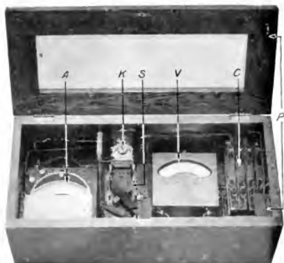
Fig. 5. Instrument and Case of Apparatus for Measuring Crest Voltage from Volt Coil
