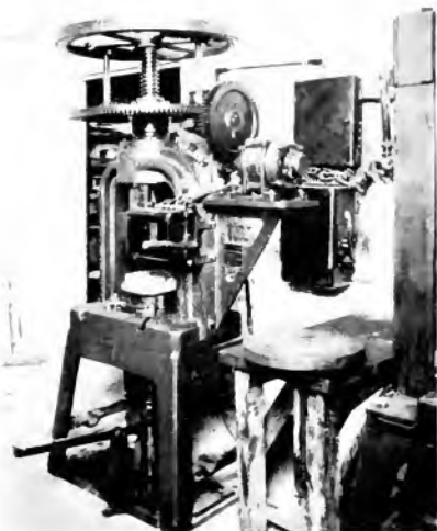
3-h.p., 1200-r.p.m., Reversible Induction Motor Operating a Mueller Machine Company's "Segger" Press, Lennox, Inc., Trenton, N. J.
