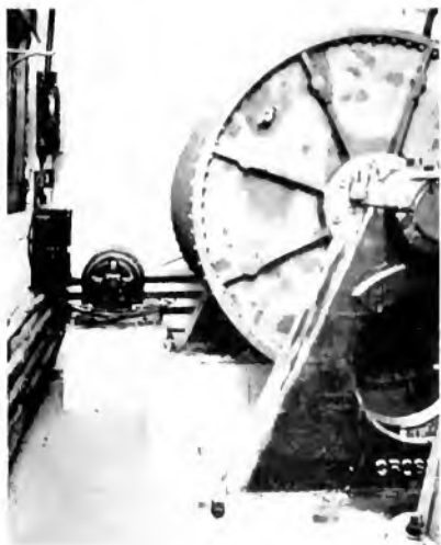
10 h.p., 1200-r.p.m. Induction Motor Operating a Crossley Machine Company's Glaze Drum, Lennox, Inc., Trenton, N. J.
