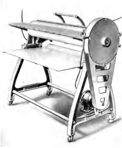
Fig. 8. The application of motor drive in the domestic laundry is no longer limited to the washing machine and wringer. The power-operated ironing machine reduces to a negligible amount the work involved in ironing.
