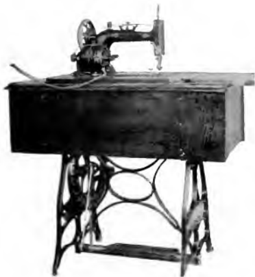
Fig. 12. Detachable type of sewing machine motor mounted in position.
