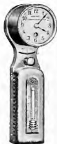
Fig. 20. A thermostat, in conjunction with the motor mechanism shown in Fig. 21, will assure the hot air furnace, steam boiler, or hot water heater maintaining the house at a constant temperature without personal attention to the dampers. The device shown can be set for any two temperatures—one for daytime, the other for nighttime—and the shifting from one to the other is accomplished by the eight-day clock
