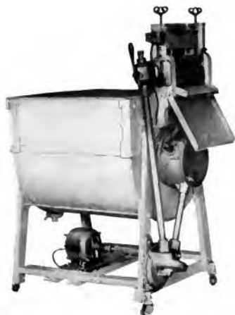
Fig. 3. Motor-driven washing machine of the cylinder type
