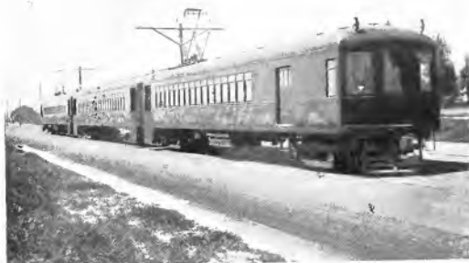
Southern Pacific Electric Train: Alameda Division. Motor Cars each equipped with four G-E. 207, 600 1200 Volt Motors with Type M Control
