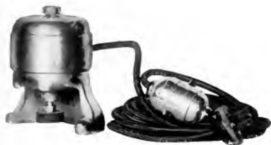
Fig. 16. Friction pulley type of phonograph motor
