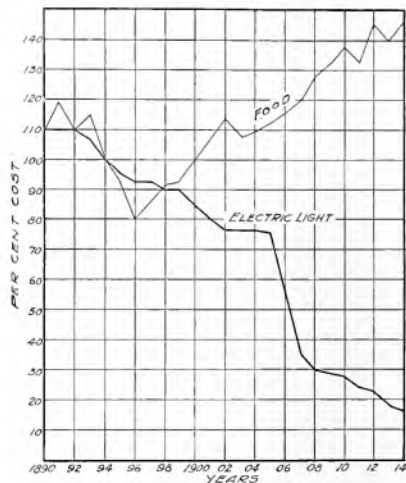
Fig. 1. Curves showing that while the cost of food commodities has been rising almost continuously, the cost of electric light has been steadily decreasing. Since the beginning of the war, the cost of food and light have both increased, but the increase in the cost of light has been very moderate.
