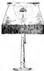
Fig. 5. Portable lamps should be designed primarily with a view to the avoidance of glare. This lamp is designed to direct the major portion of the light to the ceiling whence it is diffused throughout the room, but sufficient light penetrates the translucent reflector to light the shade to a moderate brightness. See Fig. 6
