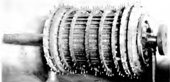
Fig. 20. Assembling the Field Coils in the Turbine generator Rotor Slots Under Heavy Pressure
