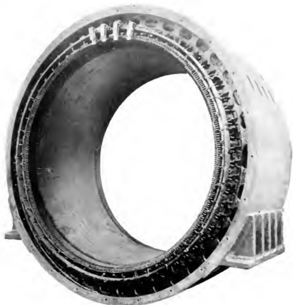
Fig. 1. Marine propulsion Induction motor Stator Completely Wound. Its rotor is shown in Fig. 2.
