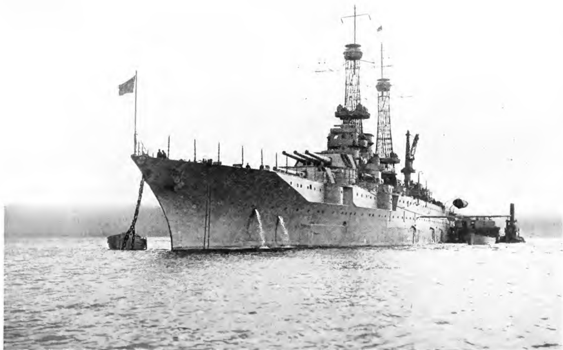
A Close-up View of the New Mexico , showing her "clipper bow," an innovation in battleship design. The main battery consists of twelve 14-inch guns, arranged three guns to each turret. She is an oil burner, and is the first battleship to be propelled by electric motors. Her trial trips have fully demonstrated the superiority of electric drive over all other methods
