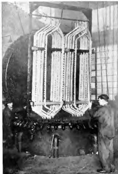
Fig. 15. After the Coils were Moulded as in Fig. 14, they were placed in this tank where all trace of moisture was removed from them and they were then impregnated with an insulating compound
