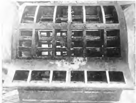
Fig. 5. Cast Type of Generator Frame Construction
