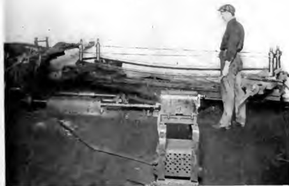
Fig. 21. Special Machine Winding Edgewise the Strip-copper Field Coils
