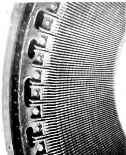
Fig. 3. Laminations Assembled and Clamped in the Induction Motor Stator Frame ready for the insertion of the winding
