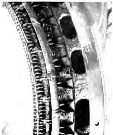
Fig. 4. A Portion of the Stator, such as shown in Fig. 3, after the winding coils have been inserted and their ends laced to the insulated steel ring
