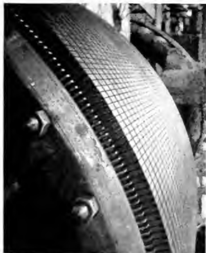
Fig. 5. Induction Motor Rotor with two sets of winding slots ready for the insertion of the bars of the double-squirrel-cage winding
