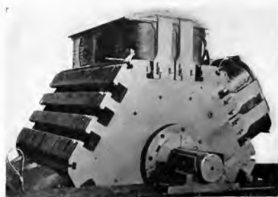
Fig. 2. An Early Salient-pole Type of Turbine-generator Rotor
