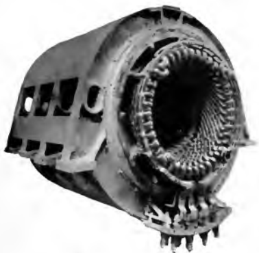
Fig. 18. The Completed Stator of one of the Maryland Propulsion Generators
