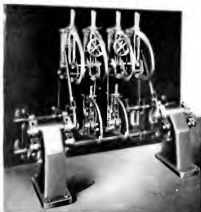
Fig. 16. Steam-limit, Speed, and Field-control Levers and Interlocks
