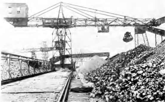
Fig. 15. Hammer Head Tower Coal Hoist at LaBelle Iron Works, Follansbee, W. Va.
