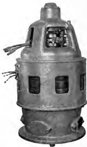
Fig. 9. Type of Motor Used for Direct Drive on Sugar Centrifugals
