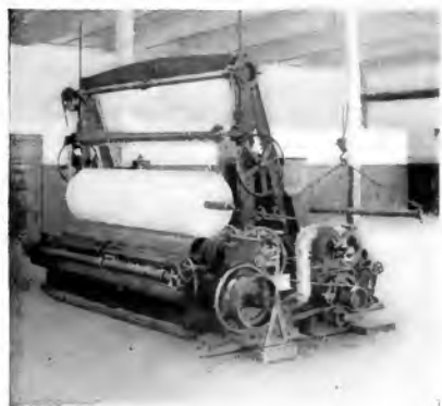
Fig. 11. 7-1/2-h.p. Induction Motor Belted to Rotary Cutter and Layby. Strathmore Paper Company, Woronoco, Mass.
