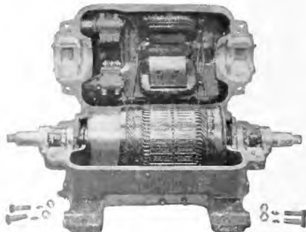
Fig. 4. MD-105, 40-h.p., 550-r.p.m., 230-volt, Series-wound, Mill-type Motor, with Upper Half Raised
