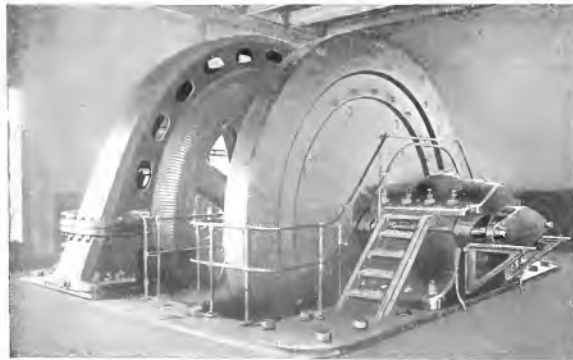
Fig. 4. 4000-h.p., 83.3-r.p.m., 6600-volt, 25 cycle, Single-speed Main-roll Motor Driving 110 in Shear Plate Mill
