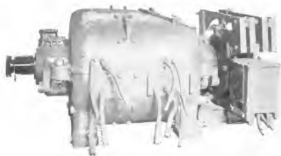
Fig. 26. 150-h.p., 230-volt, Series Wound Motor with Solenoid Brake
