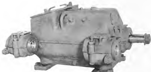
Fig. 8. MD-104 1/2, 30-h.p., 600-r.p.m., 230-volt, Series-wound, Mill-type Motor
