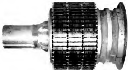
Fig. 13. Armature Core of MD-106, 60-h.p., 550-r.p.m., 230-volt, Mill-type Motor
