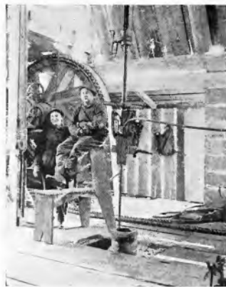
Fig. 16. The Two Handwheels on the Headache-Post at the Left Control This Motor-operated Cable-tool Drilling Rig at the Reward Oil Co., Reward, Calif.
