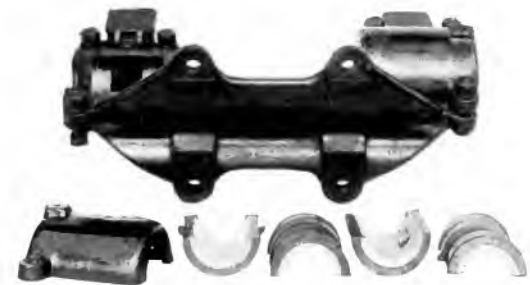
Fig. 3. Back Geared Attachment for Mine-type Induction Motor
