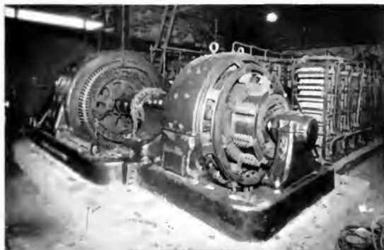
Fig. 9. 1400 950 h.p., 600 405-r.p.m., 2200-volt, Adjustable Speed Main roll Motor with Rotary Converter Speed Control Driving 21-in. Structural Mill Showing Direct-connected Direct-current Motor
