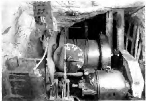
Fig. 7. Mine type, 30-h p., 900 r. p. m., 220-volt Wound-rotor Induction Motor Back Geared to a Sinking Hoist. Tennessee Coal Iron & R. R. Co., Muscoda Red Ore Division, No. 8 Mine
