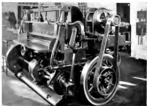
Fig. 12. Seybold Machine Company 64-in. Trimming Knife Driven by Squirrel-cage Motor. Byron Western Company, Dalton, Mass.
