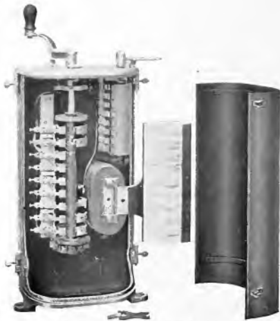
Fig. 28. Controller for Main Motors
