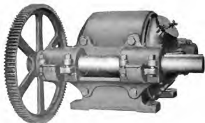
Fig. 1. Mine-type, 50-h.p., 900-r.p.m., 440-volt Back-geared Induction Motor
