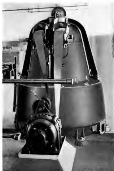
Fig. 5. 48-in. Laundry Centrifugal Extractor with Horizontal Belted Motor and Belt Tightener Head
