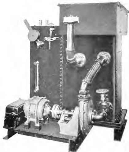
Fig. 11. Successful Type of Liquid Secondary Rheostat for Control of Mine Hoist Induction Motors. Operating Lever is on opposite side of Tank
