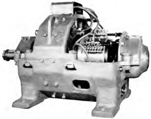
Fig. 6. MDS-110, 200-h.p., 230-volt, Series-wound, Mill-type Motor
