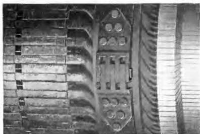
Fig. 14. Details of Binding Band and Clamp on MD and MDS Armatures
