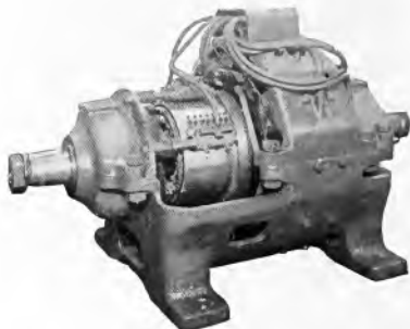
Fig. 10. Mill Motor Which is Used on Bridge Hoists
