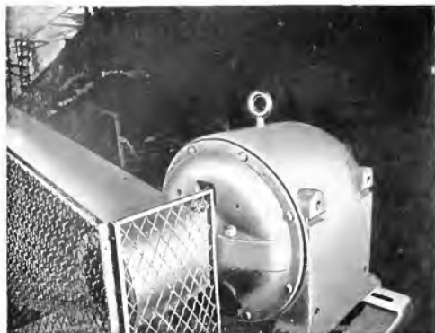
Fig. 5. Mine-type 35 h.p., 600-r.p.m., 550-volt Wound-rotor Induction Motor Driving Shaker Screen and Picking Table, Davis Coal & Coke Co., Thomas, W. Va.
