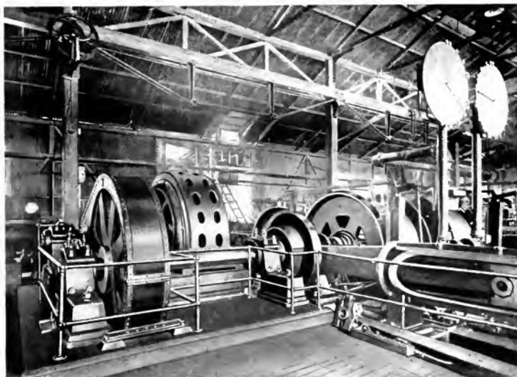
Fig. 3. First Motion Steam Hoist Converted to Electric Drive, Driven by 900 h.p. Geared Induction Motor. Bantjes Shaft, South Africa
