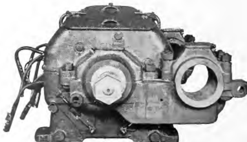
Fig. 9. MD-109, 150-h.p., 435-r.p.m., 230-volt, Compound-wound, Mill-type Motor
