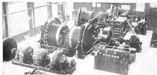
Fig. 17. Installation View of Two Automatic Mine Hoists Operating Entirely without Attention from Operator but Capable of Instant Manual Operation at Will. Inspiration Consolidated Copper Co., Miami, Arizona
