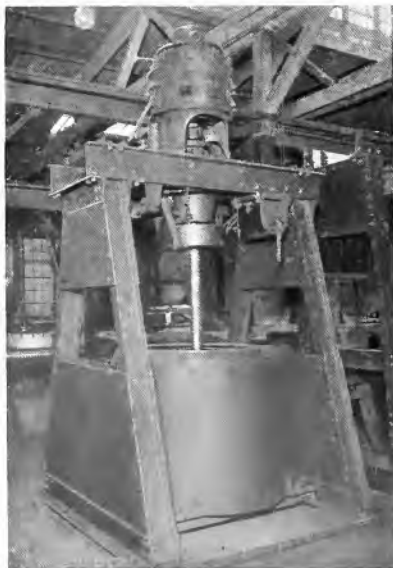
Fig. 8. 42-in. Sugar Centrifugal with Direct-connected Squirrel-cage Motor and Centrifugal Friction Clutch
