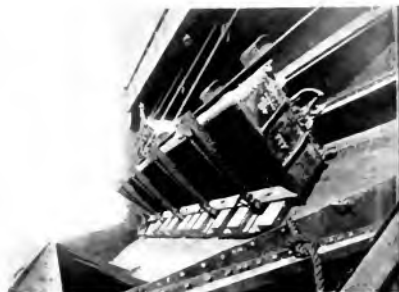
Fig. 26. High Lift Car Dumper, Car in Completely Dumped Position, Installed at Semet Solvay Coke Plant, Indiana Harbor, Ind.
