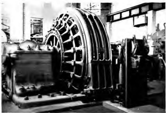
Fig. 18. 2500-h.p., 40/120-r.p.m., 500-volt, Reversing Mill Motor Driving 36-in. Blooming Mill
