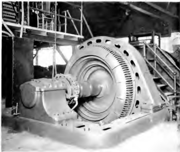
Fig. 5 1500-h.p., 450-r.p.m., 2200-volt, 30 cycle, Single-speed Main-roll Motor Driving Skelp Mill
