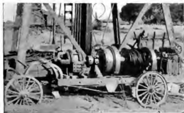
Fig. 10. Portable Electric Hoist Used for Pulling and Cleaning Jack-wells in the Kern River Field, California
