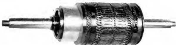
Fig. 11. Complete Armature of MD-105, 40 h.p., 550-r.p.m., 230-volt, Mill-type Motor
