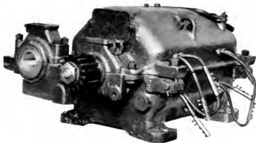
Fig. 19 MD-105, 40 h.p., 550-r.p.m., 230-volt, Series-wound, Mill-type Motor
