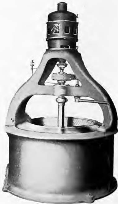
Fig. 6. Direct-driven Centrifugal Extractor with Squirrel-cage Induction Motor. A type used extensively in textile works on long duty cycles
