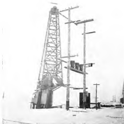
Fig. 19. A 1900 ft. Well of the Midway Pacific Oil Co. at Fellows, Calif., Drilled Entirely by Electric Power
