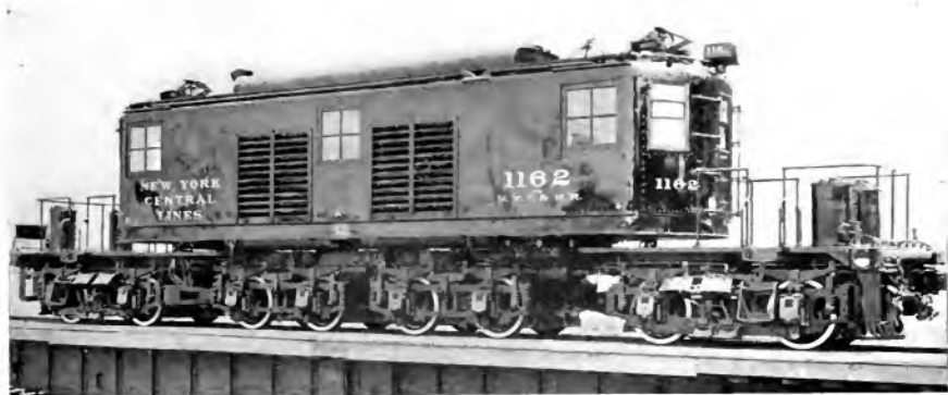
Fig. 3. Latest Type New York Central Locomotive Designed for High Speed Heavy Passenger Service Over the Electric Division Between New York and Harmon. Each unit is equipped with eight bipolar gearless motors and weighs 125 tons
