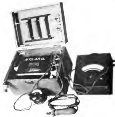
Fig. 4. Portable Outfit with Indicating Devices for Forming Films on Lightning Arrester Cones.
