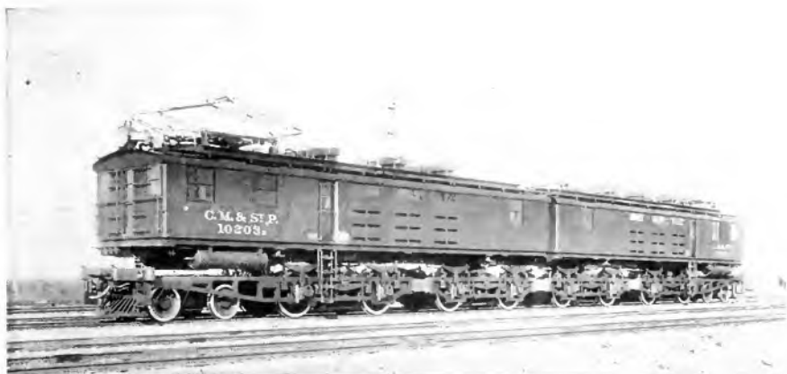
Fig. 5. 300-ton Geared Locomotive for Operation Over the Rocky Mountain Division of the Chicago, Milwaukee & St. Paul Railway. Two locomotives of this type are used to haul 2800-ton freight trains over the two per cent mountain grades.
