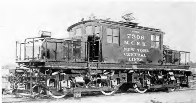
Fig. 2. 120-ton Geared Type Locomotive Operating Through the Detroit River Tunnel of the Michigan Central Railroad
