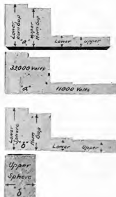
Fig. 7. Gauges used for Conveniently Setting and Checking the Setting of the Lightning Arrester Horn and Sphere Gaps
