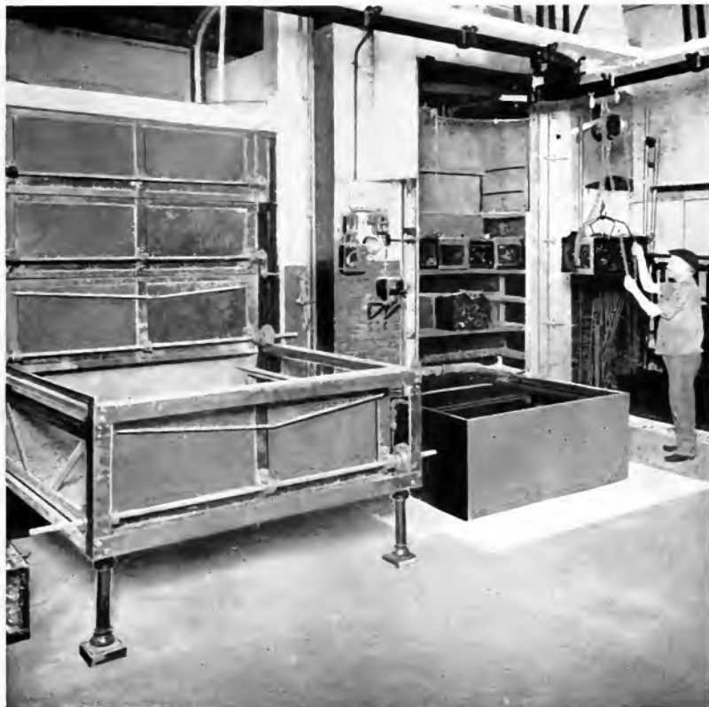
Preheating Ovens, Dip Tank, and Baking Oven for Coating Small Articles with Water Japan. This new process, which is devoid of fire risk and is cleanly, will be described in our succeeding issue
