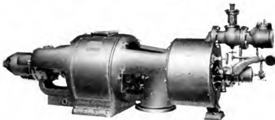
Fig. 3. Long-arc, Three-stage Turbine Direct-connected to an Alternator
