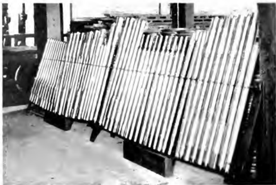
Fig. 17. Stock of Turbine Shafts
