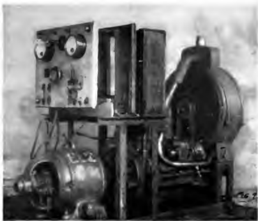
Fig. 9. "Groupe Electrogène à Essence" French 4-cylinder, 1650 r.p.m. "Ballot" gasoline engine with Constructions Electriques 29-amp., 110-volt, d.c. generator. Magneto ignition. Entirely self contained. A very popular and reliable unit much used by the French Service Electrique.
