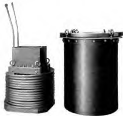
Fig. 6. Device for Amplifying Telegraphic Impulses or Telephonic Vibrations in Order that their Range of Transmission by Radio be Increased. The "magnetic amplifier," as it is called, is here shown removed from its case in which it is submerged in oil and cooled by water circulation.
