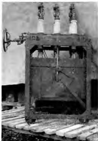
Fig. 17. Boche Portable Oil Switch. This is the same switch as in Fig. 16, but with the oil can dropped. Note the system of levers for lifting the oil can, the frame with wheels and the handwheel, which has indicating device with colored disk
