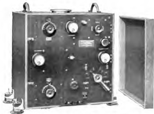
Fig. 12. 600-mile Continuous-wave Transmitter Employing Six 50-watt Photrons
