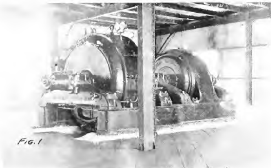
Fig. 1 Turbo-generator in Bakery Power House, Is-Sur-Tille
