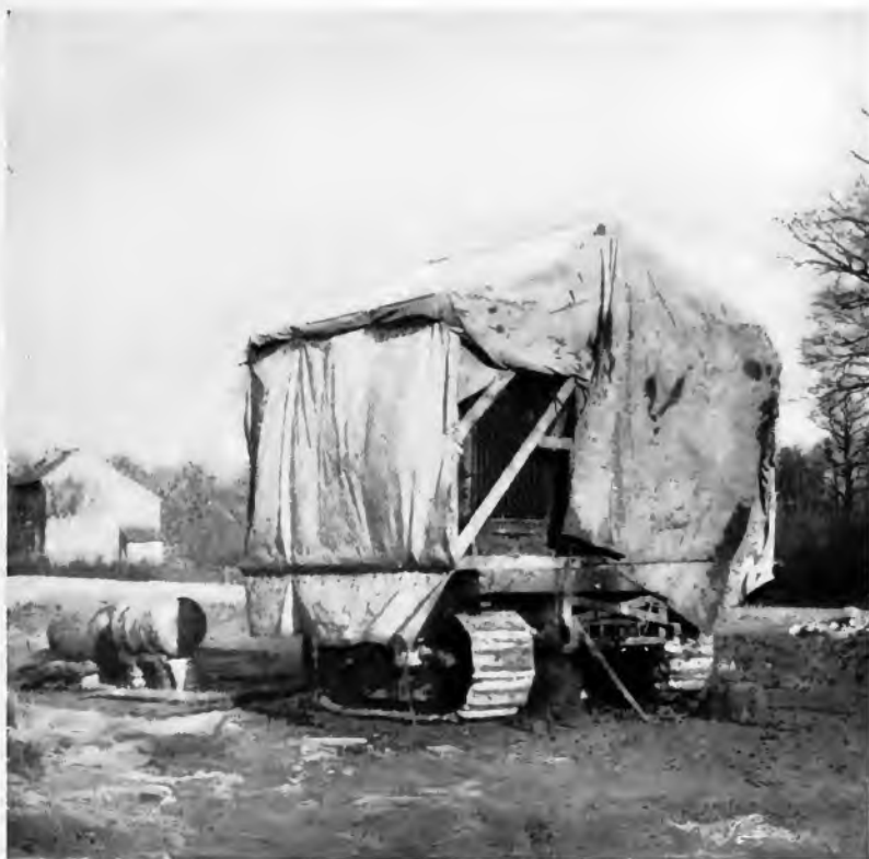
A 25-kw. General Electric Gasoline-Electric Generating Set on Caterpillar Trailer Lighting Part of Camp Leonval, France. This set had been moved up near the front in preparation for the great drive that was being planned at the time of the armistice
