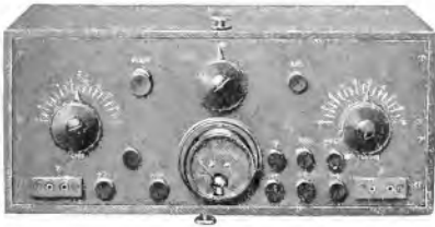
Fig. 9. Ship-airplane Radio Telephone Transmitter and Receiver Used on Smallest Type of Naval Aircraft for communication between seaplanes and ship up to 30 miles; weight 12 pounds; supplied with energy from a wind-driven generator
