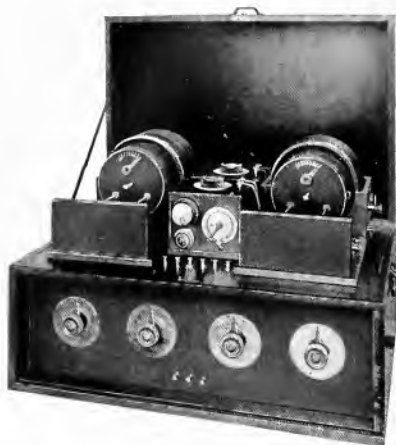
Fig. 15. Combination of Radio Receiver and Barrage Device. The upper portion comprises the receiver and the lower portion the Barrage Section. The Latter Device Screens out all disturbing static "noises" and thus permits the clear reception of the signals emanating from any selected transmitting station
