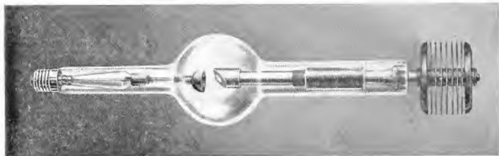
Fig. 2. Special Self rectifying, Radiator-type X-ray Tube Developed by the Schenectady Research Laboratory for the Army Medical Service. Many thousands were made by the Company during the war and they were used extensively by the Army
