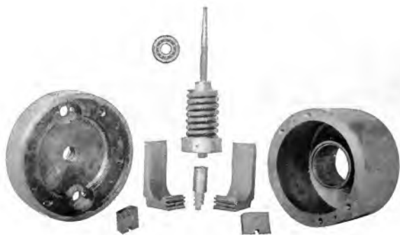
Fig. 19. Dismantled Turbine Governor
