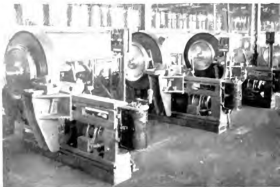
Fig. 10. Insertion of Wheel Buckets
