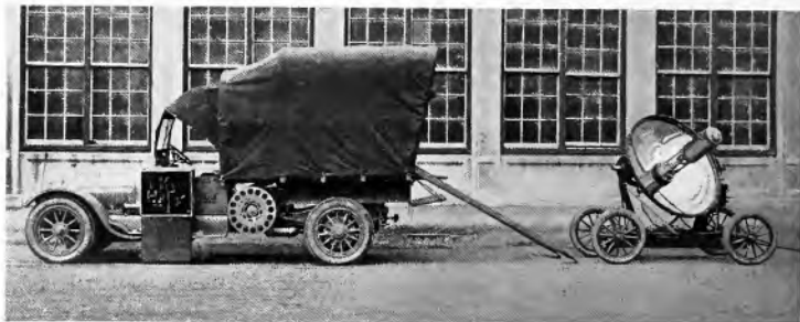
Fig. 1. General Electric-Cadillac, 20-kw Mobile Searchlight Power Unit showing Searchlight in Position for Action, Engineer Corps U. S. Army
