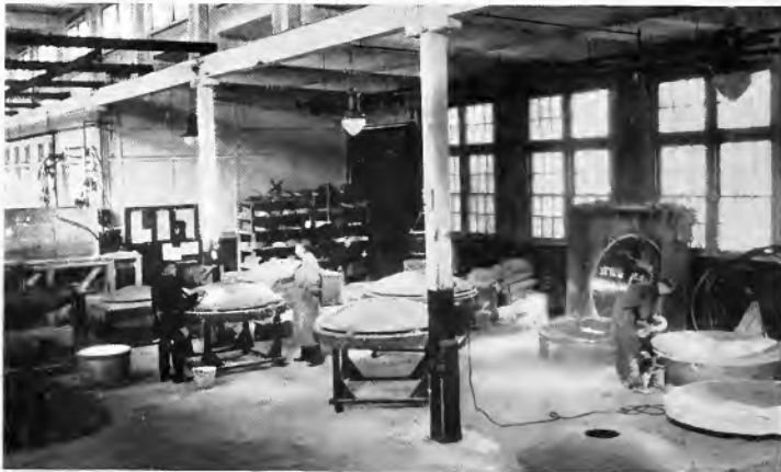
Fig. 1. Applying the Cement Backing to 60-in. Metal Mirrors at the Lynn Works of the General Electric Company
