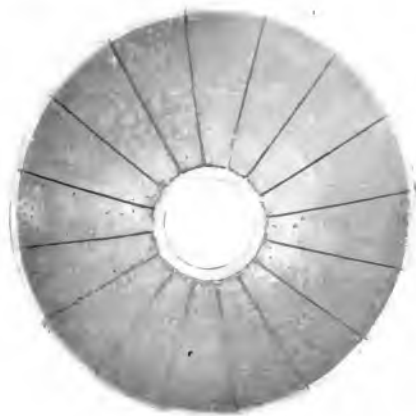
Fig. 3. A 60-in. Metal Mirror with Ribbed Sheet Steel Reinforced Cement Backing. Note the cement "rivet heads"
