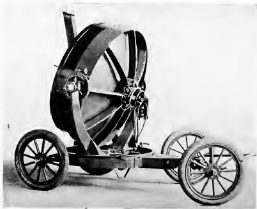
Fig. 15. High Intensity Lamp Mechanism in Place on Lynn No. 4-A Design showing Lamp Mechanism and Controls
