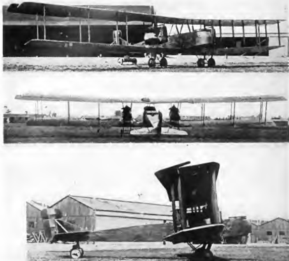
Fig. 1. Gotha Type of German Bombing Airplane
