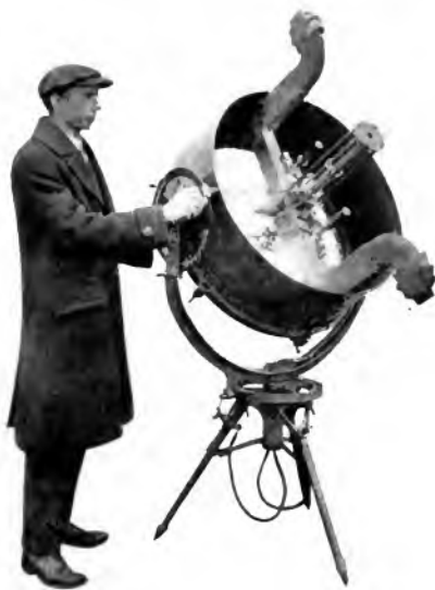
Fig. 3. 30 in. Open Type Projector Showing Method of Feeding and Rotating Carbons
