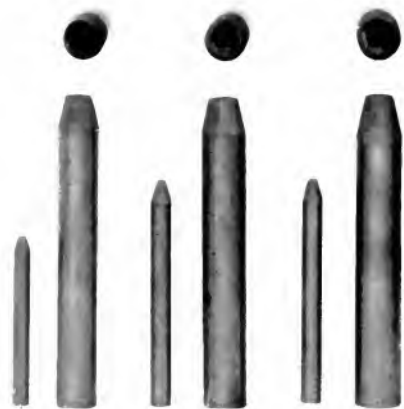
Fig. 7. 500 Ampere Medium Intensity Electrodes
