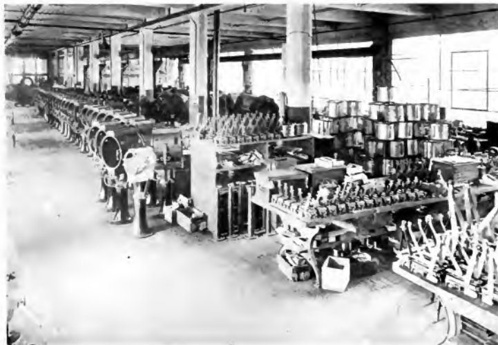
View in One of the Departments Manufacturing Some of the Smaller Searchlights
