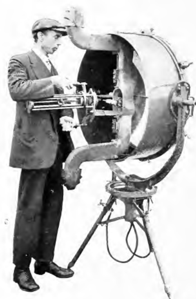
Fig. 4. Removing Lamp from 30-in. Open Type Projector
