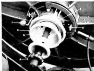
Fig. 16. Medium Intensity Lamp Controls and Breech Details of Lynn No. 4-A Design
