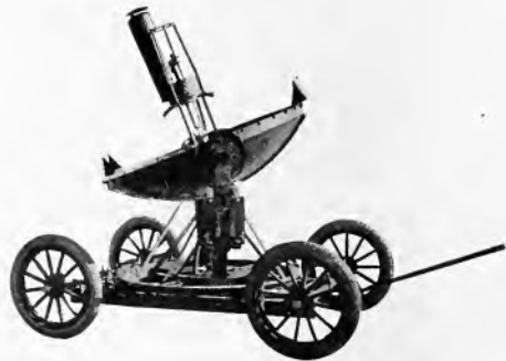
Fig. 4. 60-inch Open type Searchlight
