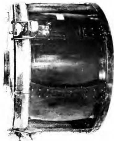
Top section of furnace showing cover as used for putting liners in large gams
