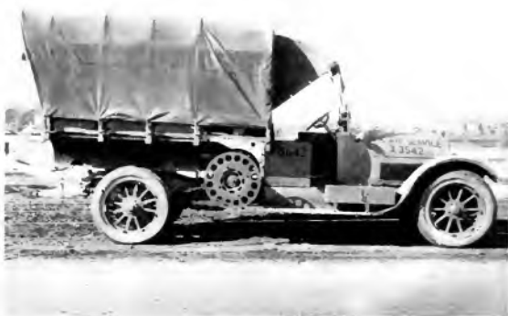
Fig. 6. General Electric-Cadillac 20-kw. Mobile Power Unit Equipped for Flood-lighting Landing Fields, Bureau of Aircraft Production, U. S. Army
