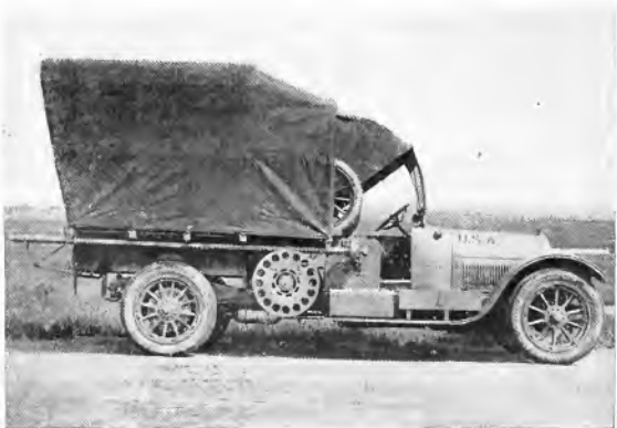
Fig. 4. General Electric-Cadillac 20-kw. Mobile Searchlight Power Unit, Engineer Corps, U. S. Army
