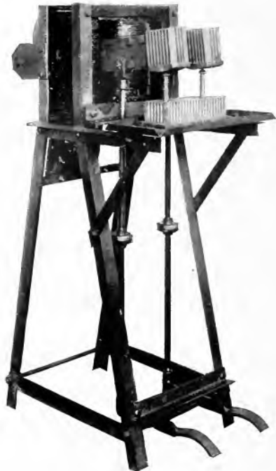
A Simple Form of Induction Device for Heating Rivets
