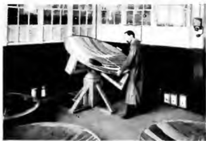
Fig. 2. The Lacquering Operation in the Manufacture of 60-in. Metal Mirrors
