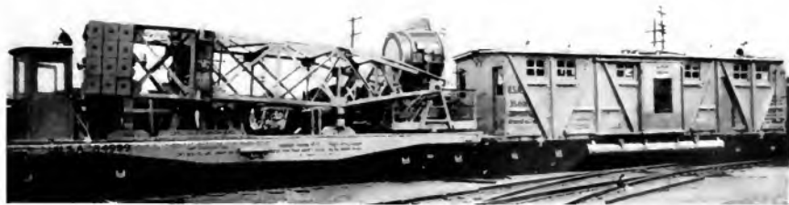
Fig. 4. 60-in. Seacoast Railway Type Searchlight. Box and Flat Car coupled together
