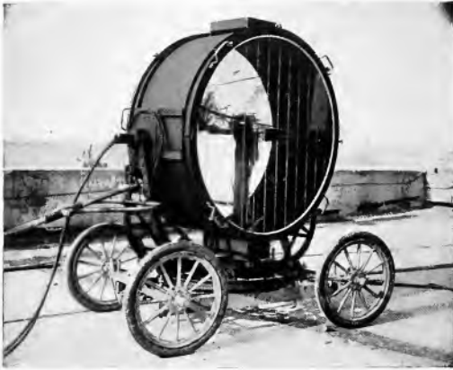
Fig. 3. Light Weight 60-inch Searchlight
