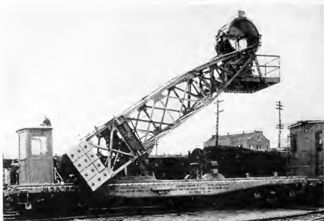
Fig. 5. 60-inch Seacoast Railway Tower Type Searchlight. Side View of Flat Car with Tower in 45-degree Position
