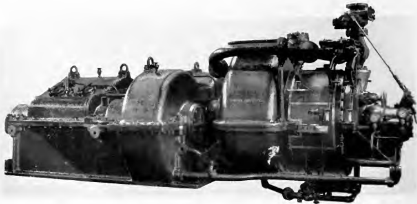
View of Complete 2500-horsepower Marine-gear Turbine Unit
