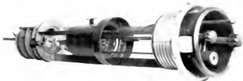
Fig. 2. View of High Intensity Arc Lamp Removed from Its Mounting
