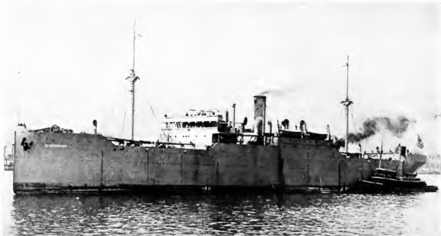
The S.S. Schenectady , one of the fabricated ships built by Hog Island. This ship was equipped with one of the 2500-horsepower ship propulsion units shown in other views
