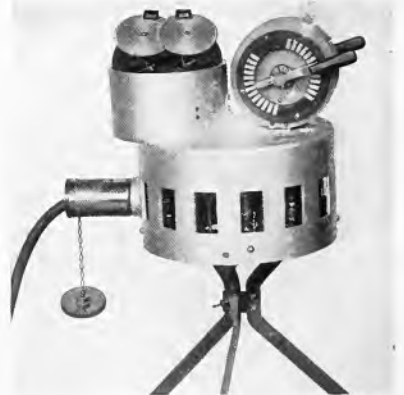
Fig. 4. Photograph showing Controller Mounted on Tripod with Transmitter and Indicator (cover removed)
