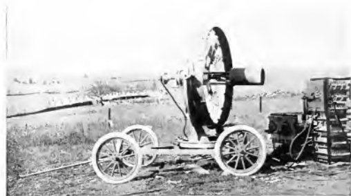
Fig. 4. An early model of the 60-in. Type Medium Intensity Searchlight adopted for army use
