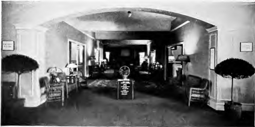
Fig. 1. View of Entrance and Foyer, Lighting Exhibit, N.E.L.A. Convention, showing General Arrangement of Rooms and Motion Picture Screen in the Background. The lighting of this area was accomplished by means of portable lamps of the direct and indirect types
