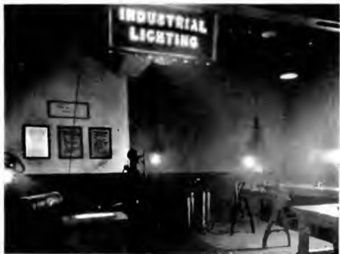
Fig. 2. View of the Industrial Lighting Exhibit, showing the Condemned or Poor Lighting. Such illumination represents a type of practice far too common which causes direct glare, sharp shadows, reflected glare and low intensity at the work. No one would be comfortable working in a room lighted in this manner.
