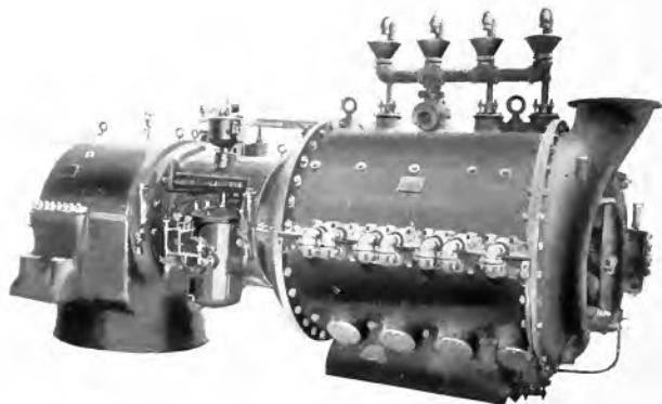
Fig. 1. Mixed Pressure Curtis Turbine-driven Centrifugal Compressor
