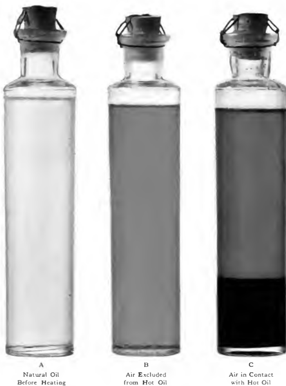
Fig. 5. Effect of Air on Hot Oil
