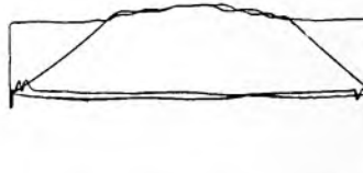
Fig. 6. Indicator Diagram Taken on Smaller Ingersoll-Sargeant Compressor After Installation of Turbo Compressor
