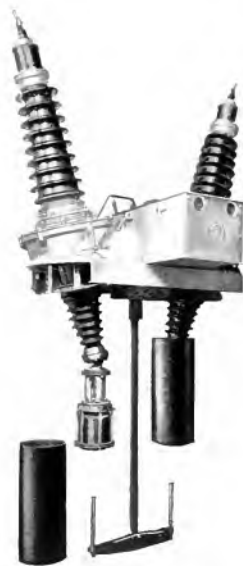
Fig. 10. Single Pole of High Capacity Oil Circuit Breaker of the FK Type, showing Insulating Shield and Explosion Chamber
