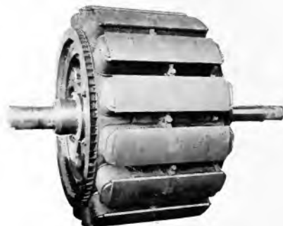
Fig. 3. Rotor of Waterwheel-driven Generator shown in Fig. 1
