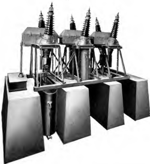
Fig. 9. 115,000-volt High Capacity Oil Circuit Breaker of the FK Type. Mounted on Structural Steel Girders which Rest on Concrete Foundation Pillars between which a Pit is Built to Allow Removal of the Oil Tanks
