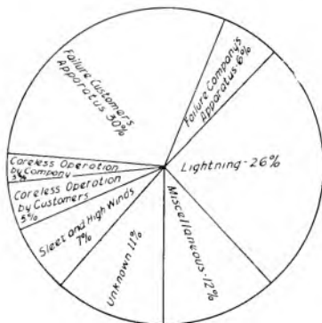
Fig. 2. Diagram Classifying and Evaluating the Disturbances on the Lines of the New England Power Co.
