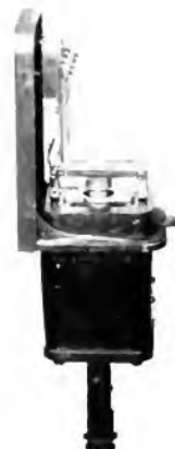
Fig. 19. Relay Used for Differential Protection of Alternators (Cover Removed)
