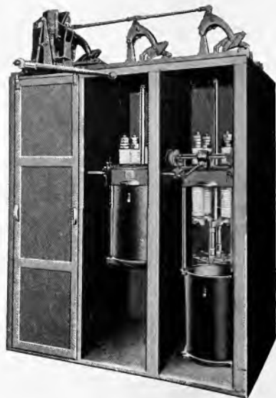
Fig. 7. Moderately High Capacity Oil Circuit Breaker of the FK Type, with Four Contacts in Each Oil Tank
