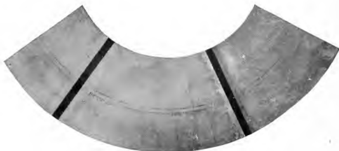
Fig. 5. Babbitted Surface of Spring Thrust Bearing After First Ten Hours Operation, showing fine radial lines not visible before the run and presumably due to machining at the factory
