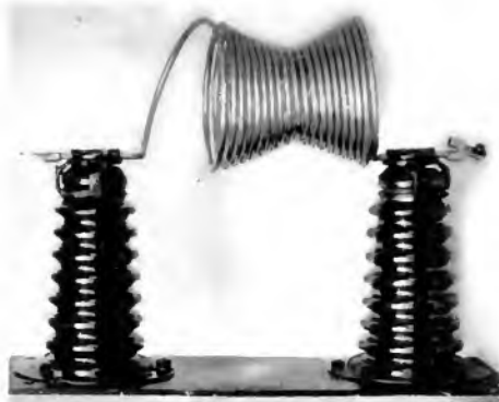
Fig. 9. Unbraced Choke Coil Deformed by Short-circuit Current. The vibration of the coil in a vertical position tends to force it downward, resulting in a pronounced distortion.
