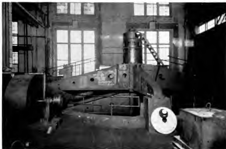
Fig. 4. Equipment for High Speed Test on Generator shown in Fig. 1
