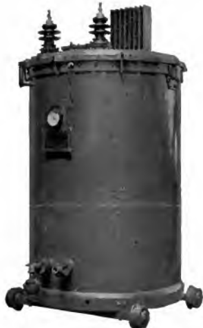
Fig. 4. Water-cooled Furnace Transformer. Due to recent largely augmented demand, the design of such transformers has been given special consideration. The transformer must deliver very heavy currents without excessive stay loss and be reliable in a class of service where short-circuits are common.
