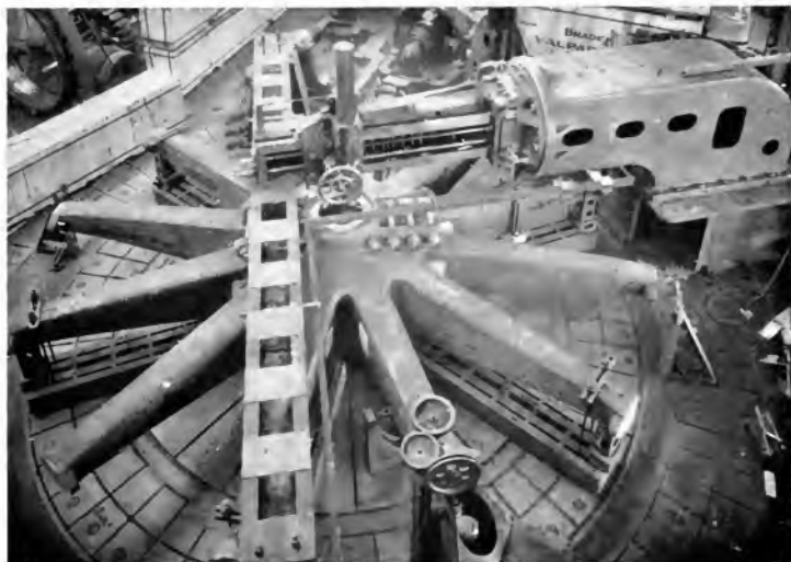
Fig 11 Rotor Spider of 10,000-kv-a. Waterwheel-driven Generator Ready for Boring and Turning Operation
