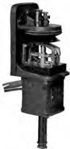
Fig. 27. Notching Relay (Cover Removed)
