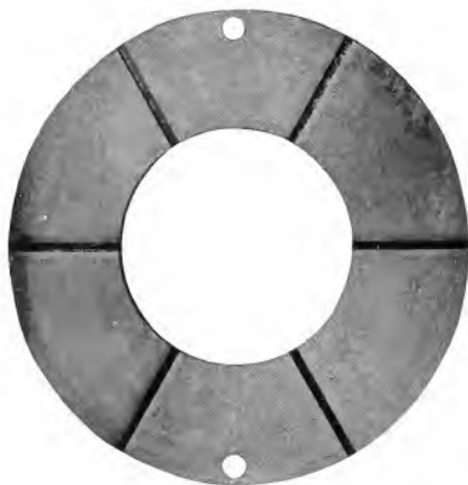
Fig. 4 Babbitted Surface of Spring Thrust Bearing After Initial Run, Cedars Rapids Power Station
