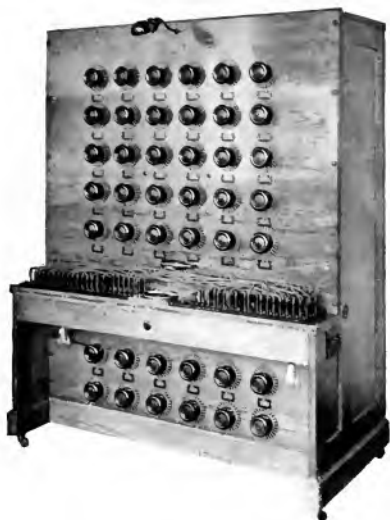
Fig. 11. Front View of Calculating Table Built for and Used by the Alabama Power Co. for the Calculation of Its Short-circuit Problems
