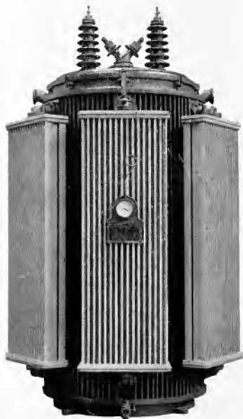
Fig. 3. 50,000-volt Moderate Capacity Power Transformer. Use of the all-welded steel radiators on transformer tanks has made practical the building of self-cooled units in any desired capacity. The installation of such transformers out of doors has eliminated the difficulty often experienced with large self-cooled units when installed indoors, of keeping the ambient temperature at a conservative value.
