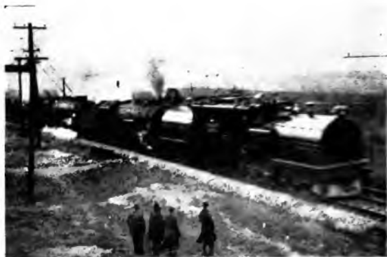
Electric Locomotive Connected for Regenerative Braking and Pushed by Two Steam Locomotives to Simulate the Effect of a Heavy Train Down grade. At times as much as 2000 kw. was returned to the trolley circuit.
