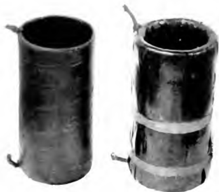
Fig. 3. Lightly Insulated Coil, on left, and Heavily Insulated Coil, on right, used in determining the effect of coil insulation on cooling after shut-down. The cooling curves are given in Figs. 8 and 9
