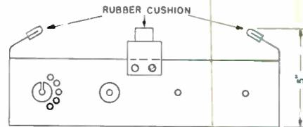
**Fig. 2B.** Showing the vertical side portion of the chassis which was bent to provide support for the 16KP4-A picture tube.
