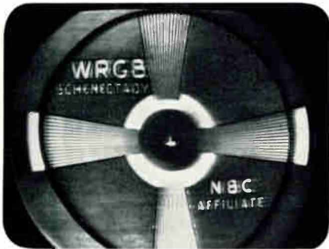
**Tele-Clue No. H-77**—This photograph and the one shown in Tele-Clue No. 78 illustrate the effect of low emission in a picture tube. The picture with the brightness and contrast controls adjusted for correct balance between the blacks and whites was very dull and had a washed-out appearance similar to Tele-Clue No. H-60. When the contrast control was advanced the color gradation between black and white practically disappeared as shown above.
