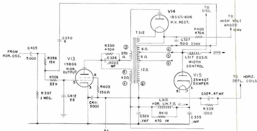
**Fig. 4.** Horizontal output circuit of General Electric Model 12C101 after making necessary changes to obtain adequate sweep width and HV for a 16KP4-A picture tube.
