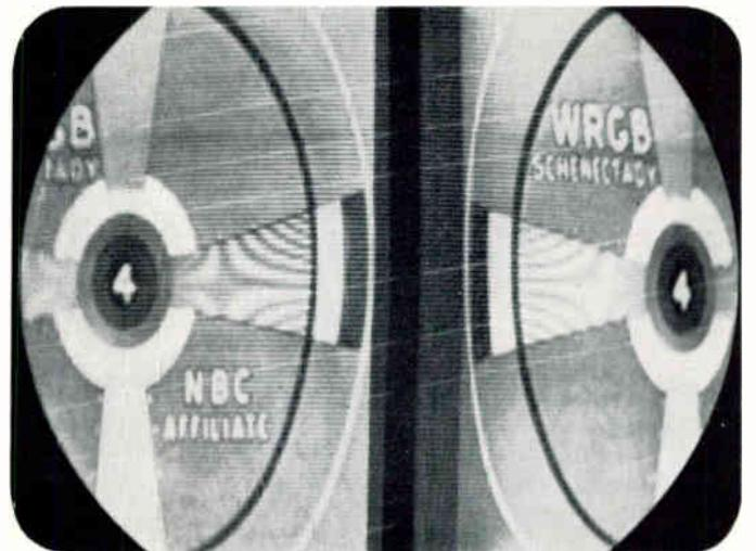
**Tele-Clue No. E-76**—This defect in horizontal synchronization which was the only point where horizontal sync would occur indicates a phase shift in the horizontal oscillator circuit shown in Fig. 1. This circuit is used in the Westinghouse Model H-606K12. A similar circuit, however, is used in a considerable number of TV receivers. This defect was caused by a change in the value of R453 from 220,000 ohms to 8000 ohms.
