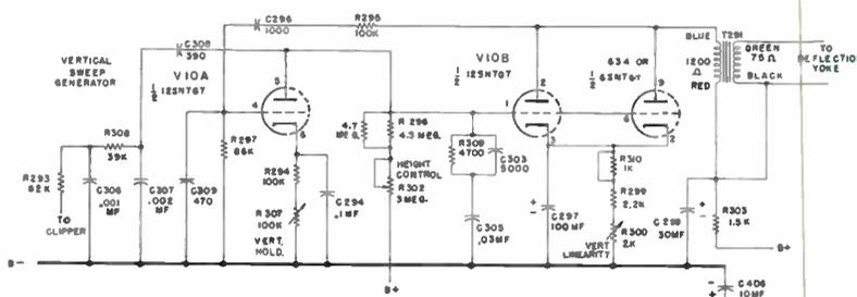
**Fig. 3.** Vertical sweep generator circuit of General Electric Model 12C101 after making necessary changes to obtain sufficient sweep for a 16KP4-A picture tube.
