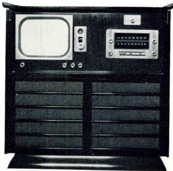
Fig. 6. The same receiver as shown in Fig. 5 after being converted to use a General Electric 14CP4 picture tube.
