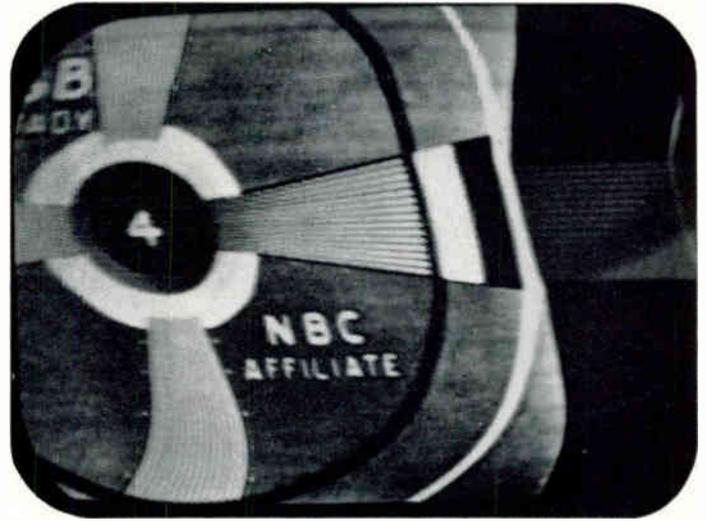
**Tele-Clue No. K-74**—A short between the cathode and heater in the 6SL7-GT Sync Amplifier and clipper tube used in a large number of General Electric chassis will result in a picture similar to either Tele-Clue No. 74 or 75. The contrast control has little or no effect. Horizontal synchronization is extremely critical with a horizontal jitter or weaving present most of the time.
