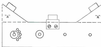
**Fig. 2A.** Front portion of the General Electric Model 12C101 chassis showing the front area which must be removed to accommodate a larger size picture tube.
