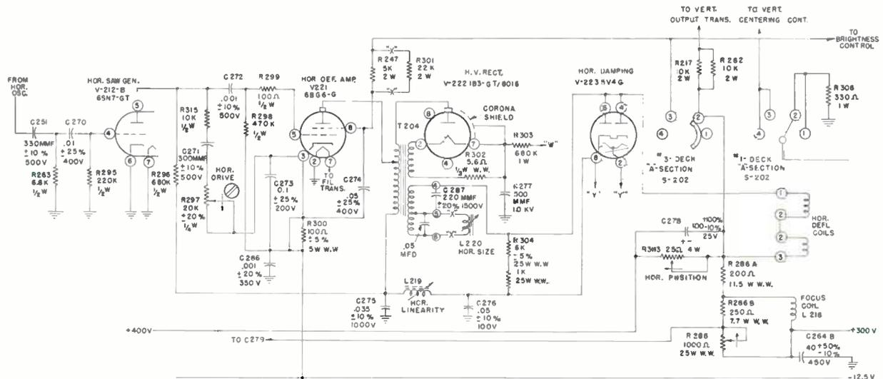
Fig. 7. Horizontal generator and output section of the Stromberg-Carlson Model TV-12 Series 11 after making the necessary changes to obtain adequate sweep width and HV for a 14CP4 picture tube.
