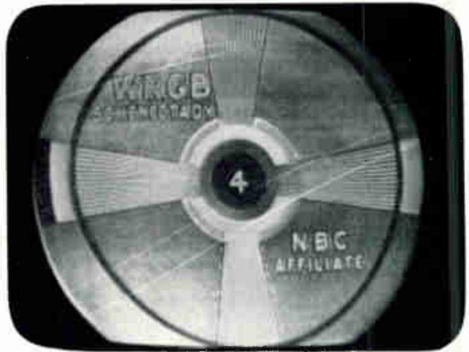
**Tele-Clue No. H-78**—This photograph shows the result of advancing the brightness control on the same tube used in Tele-Clue No. 77. The contrast control was returned to normal. The five shading rings around number 4 should vary in shading from black in the center to white on the outside. In the above photograph the outer ring is darker than the next inner ring. This is just the reverse of the normal shading sequence.
