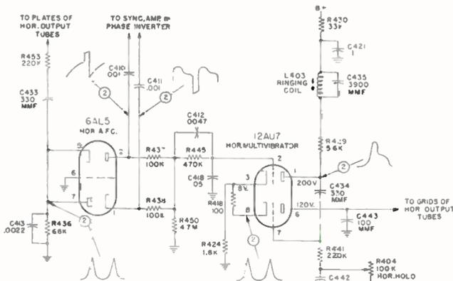
**Fig. 1.** Horizontal A.F.C. and multivibrator circuit used in the Westinghouse Model H-606K12 chassis No. V-2150-111 TV receiver.
