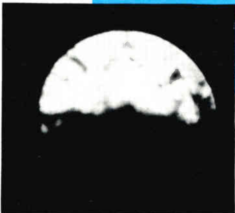
Figs. 7, 8, 9, 10. Cathode images with large areas dead. These tubes had low emission and poor picture quality.
