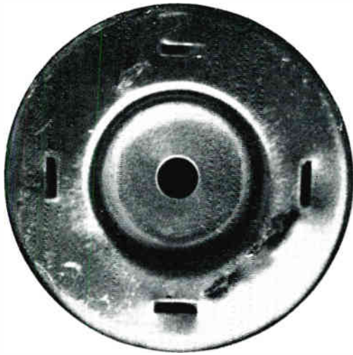
Fig. 11. Normal masking aperture at one end of HV anode cylinder.
