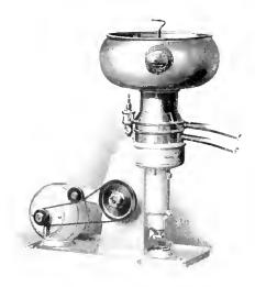
Fig. 6. Motor-Operated DeLaval No. 4 Separator
