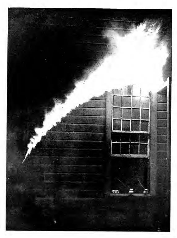
Are Drawn by Air-Break Disconnecting Switch in Rupturing a Current of 800 Amperes at 13,000 Volts
