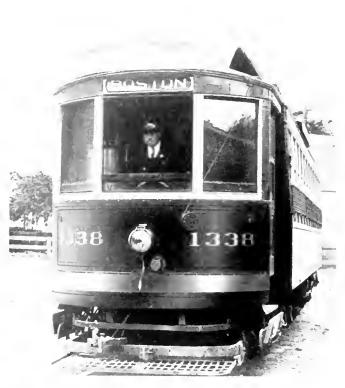
Fig. 7. Two-Ampere Headlight Permanently Attached to Front of Car
