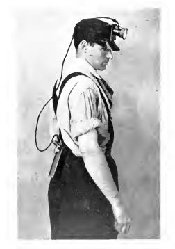
Miniature Tungsten Headlight Deriving Current from Portable Storage Battery
