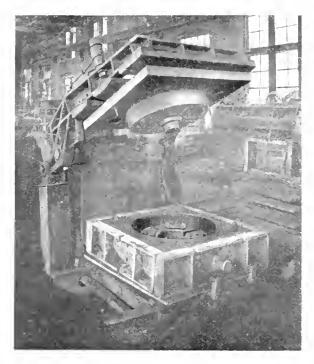
Fig. 1. Gear Moulding Machine
