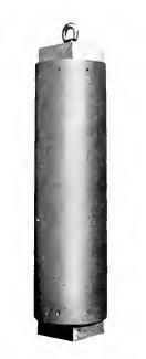
Fig. 2. Concrete Core of Power Limiting Reactance Coil
