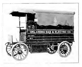
Fig. 7. 2000 Lb. Electrically Propelled Truck
