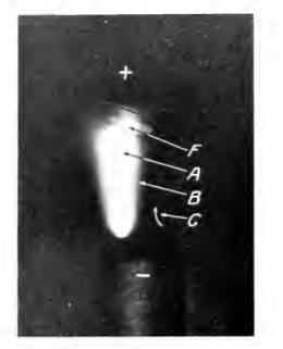
Fig. 5. Luminous Arc with Electrodes Inverted and Polarities Reversed
