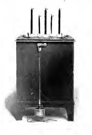
Fig. 5. Tube Tank Equipped with Shaking Magnet
