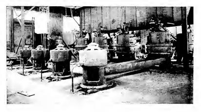
40 H.P., 500 R.P.M. Vertical Induction Motors Belted to Fuller-Lehigh Mills Universal Portland Cement Company, Plant No. 4
