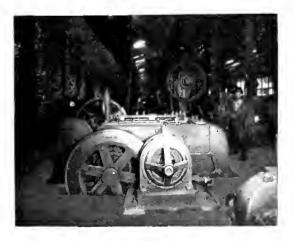
Fig. 4. Upsetting Machine in Forge Shop, Buick Motor Work.
