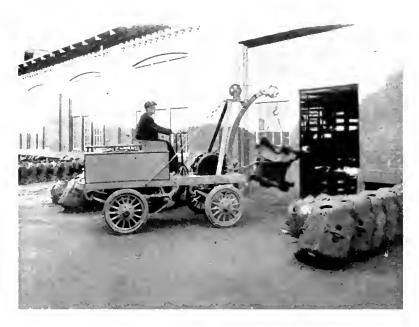
Carrying Railway Motor Castings into Machine Shop
