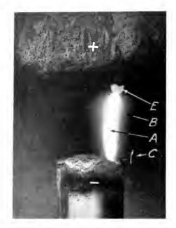
Fig. 6. Luminous Arc Showing Formation of Minute Metallic Drop on Surface of Positive Electrode
