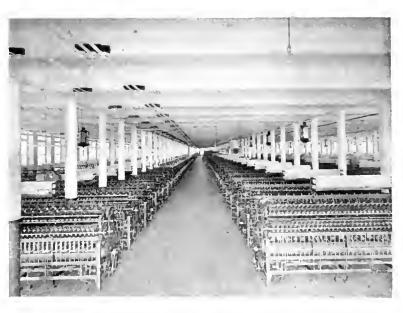
Fig. 5. View in Worsted Spinning Room, Showing Individually-Driven Frames
