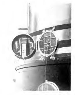
Fig. 6. Rear Compartment of 2-Ampere Headlight
