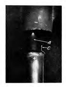
Fig. 4. Luminous Arc with Reversed Polarity of Electrodes
