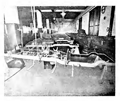
Fig 7 Portable Miller on Assembling Floor, Cadillac Shops
