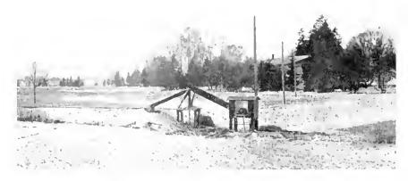
Fig. 16. Motor Driving Pump for Farm Irrigation
