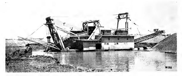
Gold Dredge—Capacity 7<sup>1</sup>, cu. ft.—Electrical Equipment: Three 125 Kw. 60 Cycle 4000 460 Volt Three-Phase Transformers, One 7<sup>1</sup>, Kw. 4000 -115 230 Volt Transformers, Switchboard and the Following 440 Volt Induction Motors: Bucket 200 H.P., Winch 25 H.P., Screen 35 H.P., Stacker 25 H.P., 10 In. High Pressure Pump 75 H.P.
