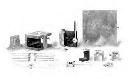
Drilling Jigs Designed and Made by First Year Apprentices. Die Holders Made by Four Months Apprentice. Training Room, Schenectady Works
