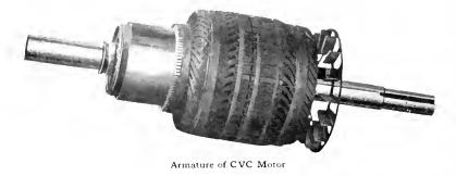
manufacturers, produces a positive circulation of air in a definite direction, resulting in a more economical use of the active iron and copper, and a more uniform temperature throughout the machine.
