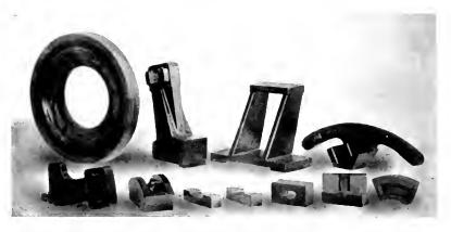
Patterns and Core Boxes for Commutator Turning Tools and Armature Flange, Made by Patternmaker Apprentices Six Months on Course. Training Room, Schenectady Works
