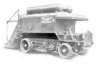
Fig. 3. Gasolene Electric Street Sweeper. Made by the Emerson Contracting Co. New Brunswick, N. J.
