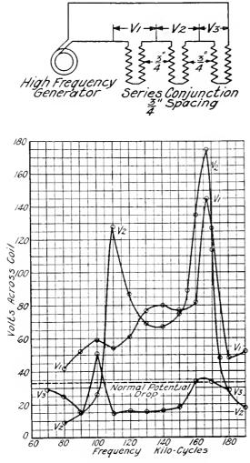
Fig. 13. Curve Showing the Two Peaks of Resonance at Different Frequencies
