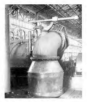
Fig. 16. Constant Volume Governor for Turbine Compressor of Fig. 15
