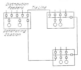
Fig. 2. Simple System, with Tie-Lines Between Generating Stations
