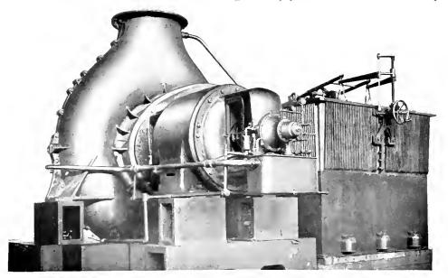
Fig. 27. Compressor Driven by 375 H.P. Curtis Turbine
