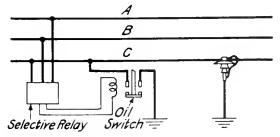
Fig. 3. Simplified Circuit of the Arcing Ground Suppressor
