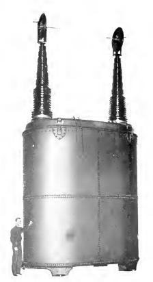
Fig. 6. 750,000 Volt Testing Transformer for Investigating Insulation for High-voltage Oil-break Switches
