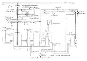
Fig. 5. Connections of Flywheel Motor-Generator Hoisting Equipment with Regulating Motor in Main Line
