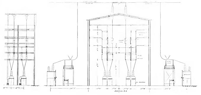
Fig. 6. Section of Indoor Substation for 110,000 45,000 Volt Circuits. Sections taken in direction of arrows shown in Fig. 5
