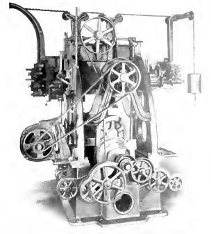
Fig. 5. Induction Motor driving Bullard 42 inch Boring Mill
