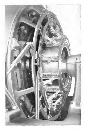
Fig. 8. Brush Raising Mechanism for Synchronous Converter
