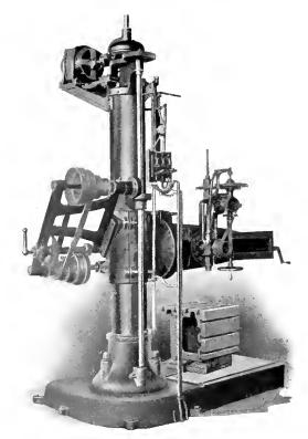
Fig. 4. Induction Motor driving 4 1-2 ft. Universal Radial Drill
