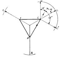
Fig. 1. One Single-phase Regulator on 3-phase System Current Transformer in One Leg of Phase
