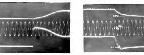
Fig. 9. Load Thrown On Oscillograms of Commutating Pole Converter, with Commutating Poles shunted by an Inductive Resistance. Upper curve, current in shunts; Lower curve, current in commutating pole; Middle curve, volts per bar
