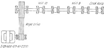
Fig. 12. Plan of 30 in, Four-Stand Sheet Mill
