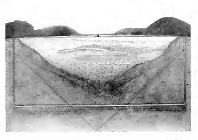
Fig. 8. Section of Hudson River at Storm King, showing Pressure Tunnel and Borings
