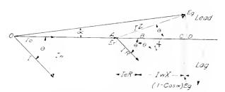
Vector Diagram of a Transmission Line Illustrating the Relation Between Generator and Receiving Voltage for Different Loads and Power factors Fig. 7
