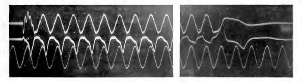
Fig. 5. Switching Line on and off with High Tension Switch. Upper curve, high tension voltage at receiver end of line; middle curve, high tension current at receiver end of line; lower curve, low tension voltage at generator end of line.
