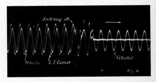
Fig. 9. Switching off 150 miles of 100,000 volt transmission line by high-tension switches. Waves of low-tension current and potential
