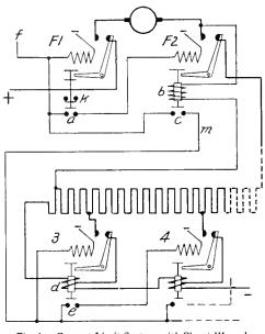
Fig. 1. Current Limit System with Shunt Wound Contactors for Direct Current Motors
