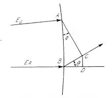
Fig. 21. Vector Diagram Showing the Condition of Constant Line Power-factor When the Voltage Drop is Maintained at Zero.
