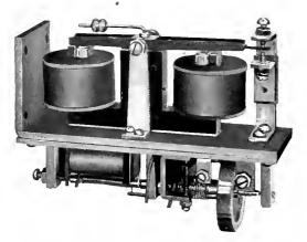
Fig. 5. Relay of the Localizer of Faulty Feeders
