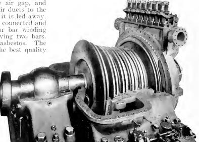
Fig. 3. Turbine with Top Half of Casing Removed
