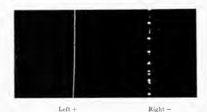
Fig. 4. Corona on Parallel Wires Iron—first polished and then run at 120,000 volts for two hours to develop "spots." Diam. 0.168 cm. Spacing 12.7 cm. Photographs taken through stroboscope at 80,000 volts.
