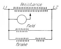
Fig. 2. Connection Diagram for Ammunition Hoist Motor
