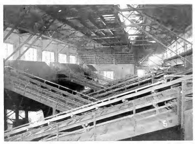
Fig. 1. Conveyors Between Breakers and Hammer Mills
