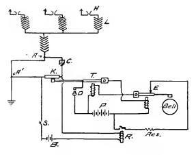
Fig. 7. Circuit Connections of the Discharge Alarm
