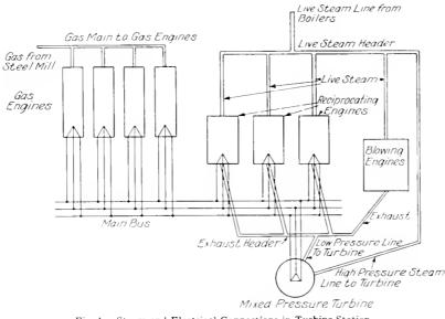
Fig. 1. Steam and Electrical Connections in Turbine Station
