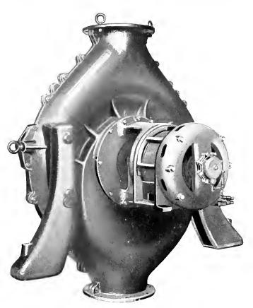
Fig. 12. Centrifugal Compressor Driven by 50 H.P. Induction Motor Front to Back, 5 Ft. 2 In.; Width, 7 Ft. 3 In.; Height, 7 Ft. 8 In.
