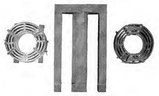
Fig. 1. Core and Coils of Constant Current Transformer
