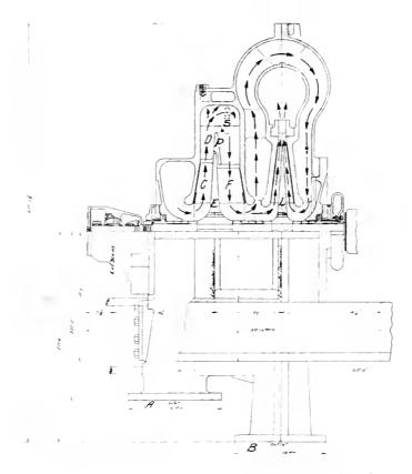
Fig. 28. Centrifugal Compressor Arranged for Cleaning Producer Gas
