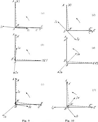
Vector Diagrams of 2-phase 3-wire Systems, showing Unbalancing of Voltages
