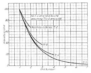
Fig. 5. Calculated Voltage Across Different Insulators in a String of n Units
