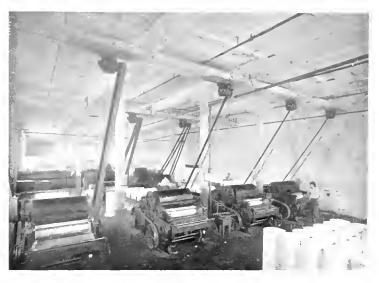
Fig. 5. Pickers Driven by Individual Motors
