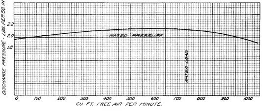
Fig. 25. Characteristic Curve of Single Stage Compressor
