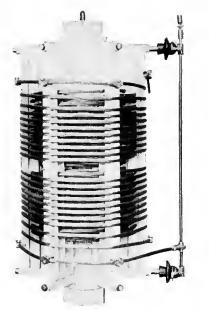
Fig. 8. Special Provision for Carrying Lower Lead to Overhead Bus
