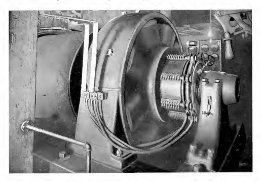
225 H.P., 250 Volt, 65 R.P.M. Direct Current Motor Driving 6 Ft. Single Drum Underground Hoist Serving Red Jacket Shaft
