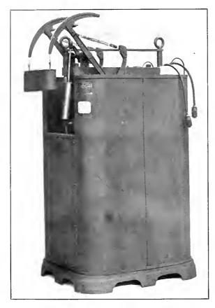
Fig. 4. Constant Current Transformer for Use with Mercury Arc Rectifier
