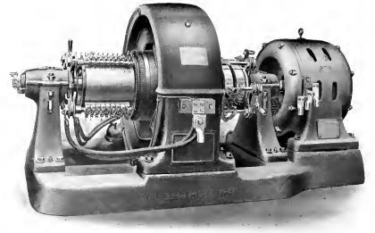
Fig. 3. Converter and Series A-C. Booster Set
