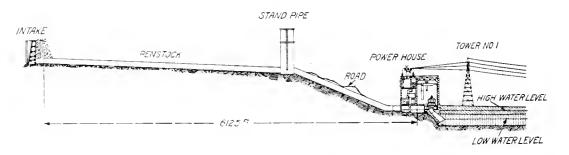
Fig. 4. Elevation of Development Showing Course of the Water from Intake to Tail Race
