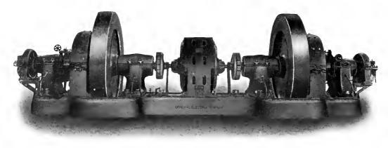
Fig. 6. Two 170 Kw., 575 Volt Shunt Wound Generators Direct Connected to 450 H.P. 2080 Volt Induction Motor, Winona Mines
