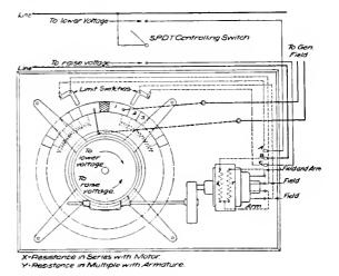
Fig. 7. Connection Diagram for Motor-operated Rheostat
