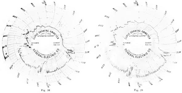
These curves illustrate the ability of a synchronous condenser to compensate for unbalanced load conditions. Simultaneous charts were taken of the voltage on the different phases which showed balanced voltages. In effecting this compensation it is necessary for the synchronous condenser to carry the unbalanced current. This data was taken from the 1500 kv-a. two-phase synchronous condenser
