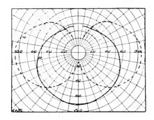
Fig. 4. Illumination Curves of Lighting Unit
