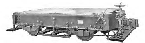
Fig. 14. Storage Battery Industrial Car. Made by General Electric Company
