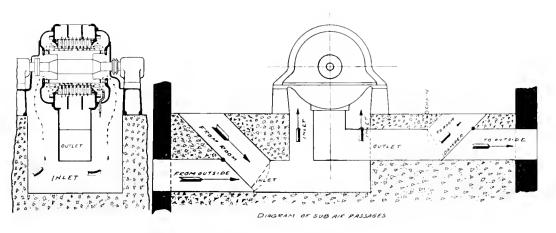
Fig. 2. Diagram Showing Air Passage and Direction of Air Flow
