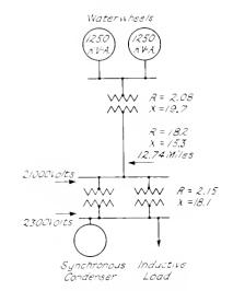
Fig. 9. One Line Diagram of a System Where Two Stations are in Parallel Connected Together by a Transmission Line
