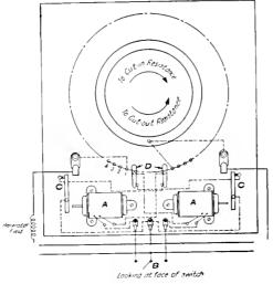
Fig. 6. Connection Diagram for Solenoid-operated Rheostat
