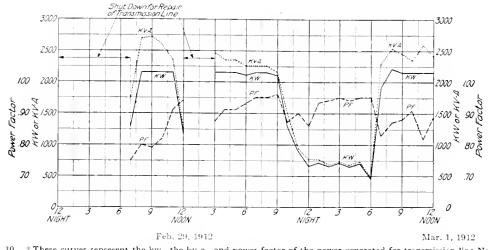
Fig. 30. \*These curves represent the kw., the kv-a., and power-factor of the power generated for transmission line No. 1. The data is plotted from readings on station instruments at Trenton Falls
