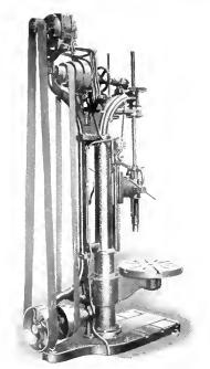
Fig. 3. Induction Motor driving Prentice 24 inch Drill
