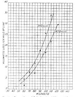
Fig. 2. Comparison of Calculated and Measured Losses The x and • are measured values. The drawn curve is cal-culated from corona formula (6). Diam. of wire 0.064 in. Spacing 48 in. Single-phase. Tests made on short line for Stanley G-I Electric Company by Mr. A. B. Hendricks, 1903-1904. This shows check at two frequencies.
