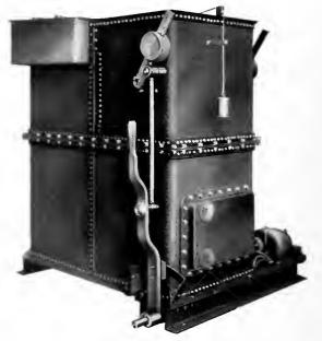
Fig. 2. Liquid Rheostat for Mine Hoist Induction Motor
