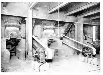
25 H.P., 600 R.P.M., 60 Cycle, 440 Volt, Induction Motors Driving No. 5 Gyratory Crushers. Knickerbocker Portland Cement Company, Hudson, N. Y.
