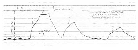
Fig. 15. Wattmeter Record of Power Supplied to Two Mills
