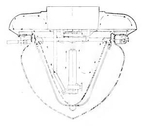
Fig. 1. Diagram of Enclosed Flame Arc Lamp, Showing Circulation of Air and Gases
