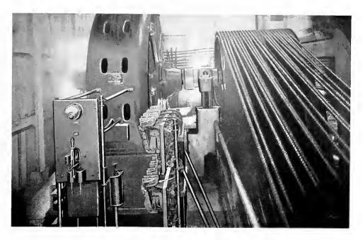
700 H.P., 440 Volt, 150 R.P.M. Motor, Rope Driving 64 Ft. Sand Wheel
