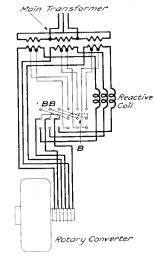
Fig. 1. Connections of Starting Switches and Reactive Coils for Six-Phase Converters
