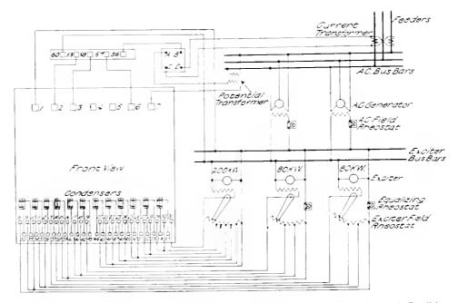
Fig. 2. Connections of Automatic Voltage Regulator with One Arrangement of Three Exciters in Parallel
