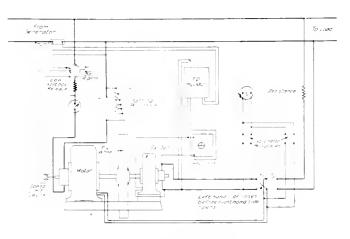
Fig. 10. Connections of Flywheel Equalizer Set with Automatic Voltage Regulator
