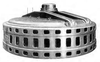
Fig. 6. 2300 kw., 97 r.p.m. three-phase generator, showing the appearance of a slow speed machine with the top bracket provided with a bearing for supporting the weight of the revolving part of the generator and the waterwheel runner
