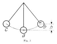
it accelerates, the potential energy decreases, but the kinetic energy increases, until in the middle position, *a*, all the energy is kinetic
