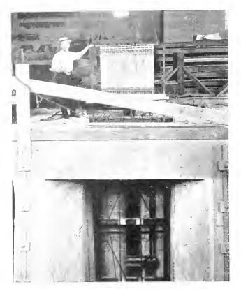
Fig. 5. Upper Portion of Moveable Framework, with Glass Reading Tubes Backed by Graduated Board
