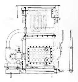
Fig. 3. Internal Construction of Liquid Rheostat
