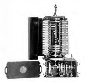
Fig. 13. Drum Controller for 300 H.P. Hoist Motor, Showing Mounting of Mechanical Acceleration and Retardation Limit Device
