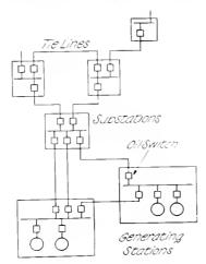
Fig. 1. Complicated System, with Substations in Series and Tie-Lines Between Substations
