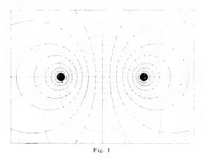
circles in Fig. 1. There further exists a condition of stress in the space surrounding the conductor, which is called the electrostatic or *dielectric field*, and is represented by lines of dielectric force, shown dotted in Fig. 1. This figure is the cross section of the two fields, the magnetic field and the dielectric field, of conductor and return conductor.
