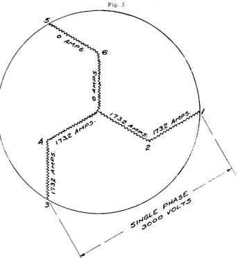
Diagrams for Connecting Three-Phase Generator to Single-Phase (519.6 Kv-a.)
