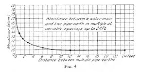
by 50 per cent. Half the total resistance of the pipe-earth, therefore, lies within 6 inches of the pipe.
