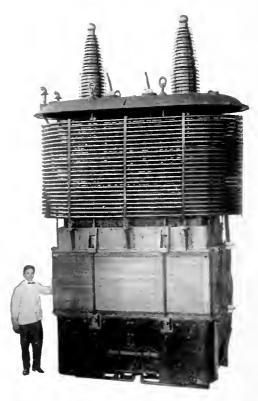
Fig. 3. 3000 Kv-a. 140,000 Volt Water-Cooled Transformer Without Case
