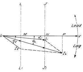
Fig. 4. Vector Diagram of Two Generators in Parallel
