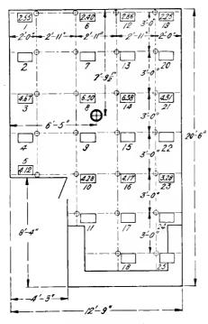
Fig. 6. Layout and Intensities for Indirect Illumination
