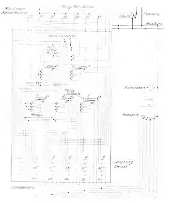
Fig. 3. Connections for Large Slow Speed Generators
