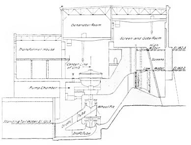
Fig. 3. Cross-section Through Turbine Room and Gate Room
