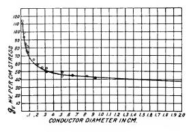
Fig. 10. Visual Critical Voltage Gradient, Two Parallel Wires
