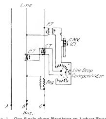
Fig. 3. One Single-phase Regulator on 3-phase System with Line Drop Compensator. Current Transformer in each Leg of Phase
