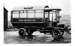
Fig. 9. Passenger Omnibus Fitted on Chassis of Fig. 8
