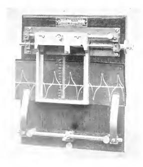
Fig. 1. Micrometer for Measuring Oscillograph Records
