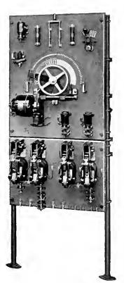
Fig. 7. Control Panel Used with Direct Current Full Automatic Single Motor Printing Press Drive
