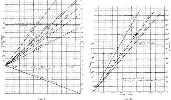
Fig. 17 represents a theoretical calculation of the condition where zero voltage drop is maintained while Fig. 18 represents an actual case, the readings being taken with station meters and instruments. The constant voltage at the receiving end of the line was accomplished by means of a 1000 kv-a. synchronous condenser, the regulation being within 2 per cent. It is interesting to note that the power-factor maintained constant from no load to full load
