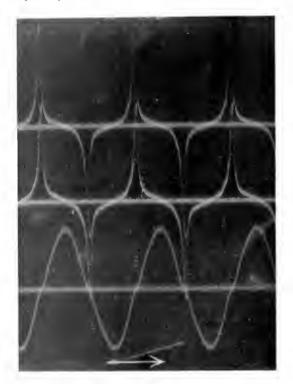
Fig. 4. Saturated Iron Reactance, Sine Wave Magnetizing Current. Upper Curve, Secondary Voltage; Middle Curve, Primary Voltage; Lower Curve, Current
