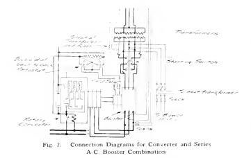
voltage by the required amount, depending on the direction and amount of field excitation. This combination of synchronous booster, direct-connected to the converter, has the advantage over the induction regulator of greater simplicity and reduced amount of station wiring. The connection diagram for this combination is shown in Fig. 2; while the appearance of the set is shown in Fig. 3.
