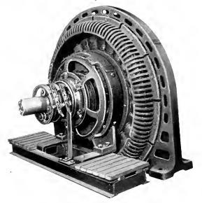
Fig. 2. Engine-driven Generator with Direct-connected Exciter
