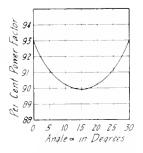
Fig. 4. Power-factor of Three-phase to Two-phase Transformers Fluxes 120° Apart
