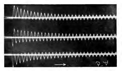
Fig. 8. Three-Phase Short-Circuit of 25 Cycle Turbo-Alternator at One-quarter Voltage. Currents in the Three Lines
