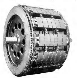
Fig. 5. Revolving Field of 10,000 kw., 514 r.p.m. threephase generator, showing spider made of plates of rolled steel
