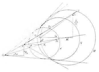
Fig. 16. Circle Diagram for Circuit A, Based upon Principle of Inversion
