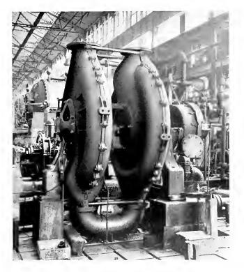
Fig. 26. Centrifugal Compressor Driven by 80 H P. Curtis Turbine
