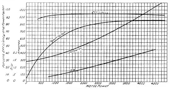
Fig. 6. Characteristic Curves of Induction Motors
