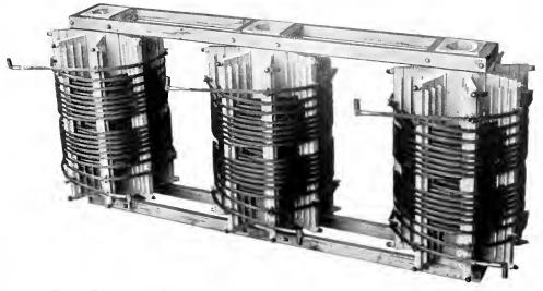
Fig. 7. Bank of 6 Per Cent Reactances for Three-Phase, 50 Cycle, 15,000 Kv-a., 11,000 Volt, Turbo-Generator. Showing Method of Mounting and Bracing
