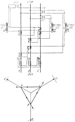
Fig. 7. Three Single-phase Regulators on 3-phase System, giving Independent Regulation of each phase
