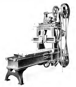
Fig. 2. Individual Drive. Induction Motor driving Pratt and Whitney 24 inch Planer
