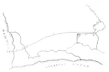
Fig. 1. Map of Cia Docas de Santos Hydro-electric System. A, intake; B, flume, C, forebay; D, pen stocks; E, power house; F, narrow gauge railway; G, general store; H, point of debarkation; 1, transmission line; J, dead ends; K, substation.
