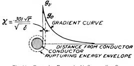
Fig. 11. Rupturing Energy in Air Surrounding One of Two Parallel Conductors
