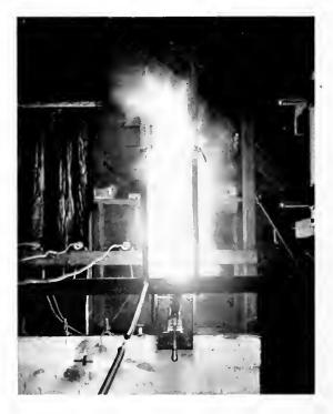
Fig. 3. Transient Electric Arc in Air, Showing the Necessity of Oil-break Switch When Large Amounts of Power are to be Opened
