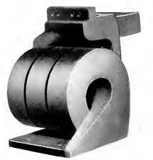
Fig. 6. Blow-out Coil Cast in One Piece by the Use of Boron Suboxide. Turns Squeezed Together After Casting
