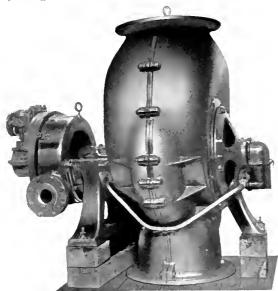
Fig. 22. Centrifugal Compressor Driven by 75 H.P. Curtis Turbine
