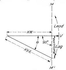
Fig. 2. Relation of Wattless Ky-a, to Power-factor and Actual Kv-a., Assuming the Kilcwatt Output and Voltage Constant
