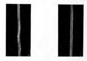
Fig. 3. Corona on Polished Parallel Wires without Stroboscope
