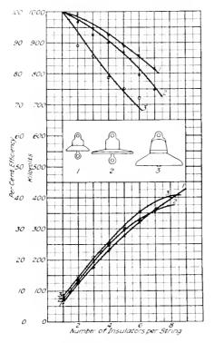
Fig. 3. Test Arc-Over and Efficiency Curves for Different Sizes and Types of Insulators
