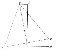
Fig. 21. Reactance Drop in T Connected Transformers, 3-Phase Primary. Perfect interlacing and equal per cent. reactance in main and teazer.
