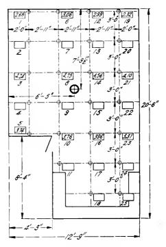
Fig. 7. Layout and Intensities for Direct Illumination
