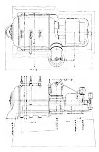
Curtis Turbine Driven Centrifugal Compressor Disconnected Compound Steam Engine Driven Blower
