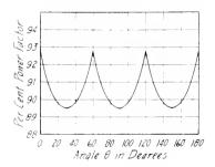
Fig. 2. Power-factor of Three-phase to Two-phase Transformers, Fluxes  $90^{\circ}$  Apart
