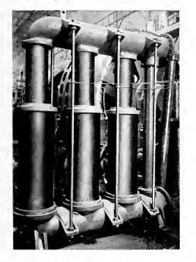
Fig. 3. Water-cooled Resistance for One Induction Motor
