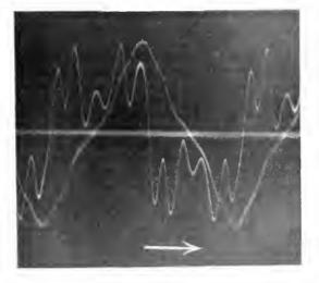
Fig. 7. Wave of Current Charging an Aluminum Electrolytic Condenser, and of Voltage on the Condenser
