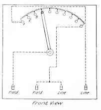
Fig. 10. Connections of Series Shunt Rheostat for Direct Current Generator
