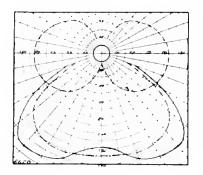
Fig. 7. Characteristic Distribution of Reflectors Shown in Fig. 6
