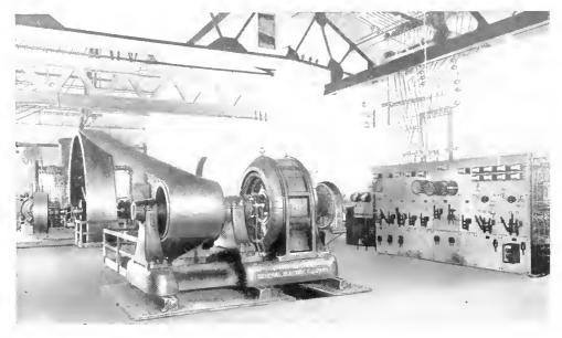
Fig. 9. 400 H.P., 3300 Volt, 500 R.P.M. Synchronous Motor Driving 2500 Cu. Ft. Compressor in A and B Compressor House
