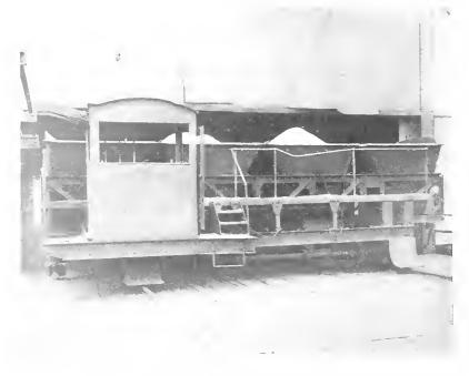
Fig. 3. Larry Car Receiving Crushed Coal Overhead from Storage Bins, and Delivering Into Coke Ovens Through Charging Holes in Roof of Latter
