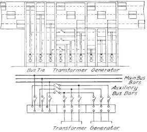
Fig. 5. Design for Locating Switching Equipment on Gallery Forming Roof of Transformer Room
