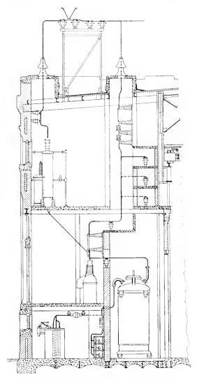
Fig. 8. Cross-Section of Power Station Showing the Relative Location of Transformers, Switches, Wiring, Etc.
