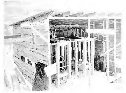
Fig, 4. Oil-break Switches Under Test Conditions Made to Represent Actual Operation
