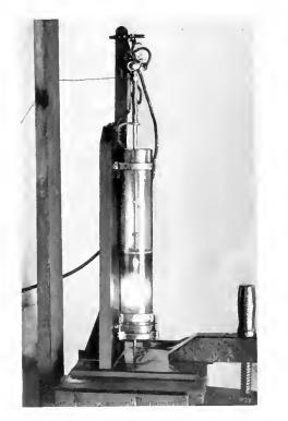
Fig. 2. Miniature Oil-break Switch Used for Experimental Study of Arc-squelching Schemes
