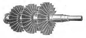
Fig. 17. Rotating Element of Three-Stage Blast Furnace Compressor
