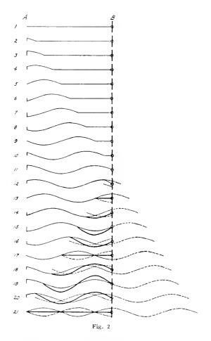
towards A, superimposes on the original wave coming from A to B, and both combined are shown in curves (12) to (21) in heavy drawn lines. As seen, this resultant wave does not travel, but its maxima and its zeros are always at the same points; and it therefore is a stationary or standing wave, which spreads from B towards A, and is formed by the combination of the traveling wave and its reflected wave.
