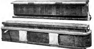
Fig. 3. Field Pole and coil of 10,000 kw. 400 r.p.m. 11,000 volt vertical three-phase generator, showing field pole, form of dovetail and dovetail reinforcement on pole piece
