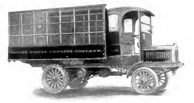
Fig. 7. Gasolene-Electric Express Truck. Made by The Tate Gas-Electric Motor Vehicle Company, New York City
