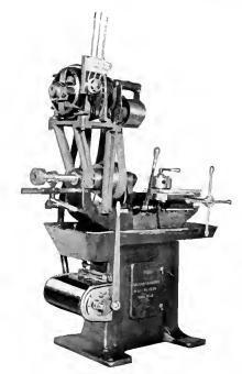
Fig. 6. 1 H.P. 4-Speed Induction Motor operating Bardons and Oliver Screw Machine
