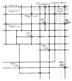
Fig. 1. Edison 3-wire System of Distribution
