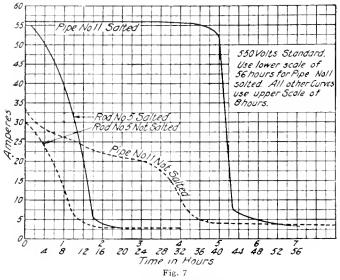
of the value of the use of salt water. In Fig. 7 is given also the ampere-hour capacity of a rod one-half inch in diameter. The rod is much inferior in capacity to the pipe under both conditions of test. Before salting, it had a capacity of about 15 ampere-hours with a constantly decreasing current, and, after salting, of about 90 ampere-hours with a constantly decreasing current.
