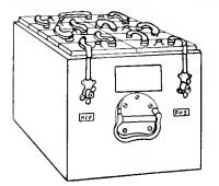
Fig. 2. Lead Battery for Electric Vehicle in Tray
