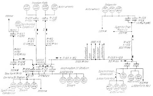
Fig. 22. One-line \* Diagram Showing the Generators, Synchronous Condensers, Transmission Lines, etc., of the System of the Utica Gas & Electric Company
