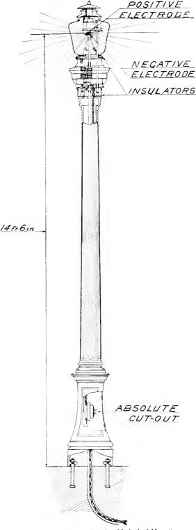
Fig. 11. Diagram Showing Method of Mounting Ornamental Luminous Arc Lamp
