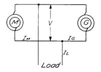
Fig. 5. An Alternator and Motor in Parallel
