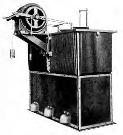
Fig. 4. Automatic Slip Regulating Rheostat
