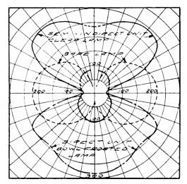
Photometric Curves for 250 Watt Units, giving average apparent candle-power in a vertical plane
