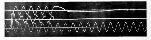
Fig. 2. Switching Line on and off with High Tension Switch. Upper curve, high tension voltage at generator end of line; middle curve, high tension current at generator end of line; lower curve, low tension voltage at generator end of line.
