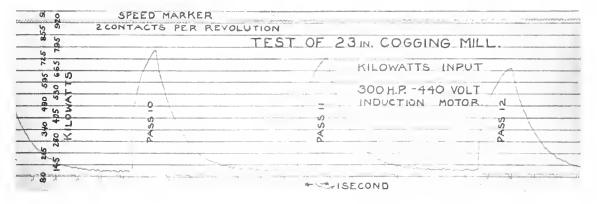
Fig. 16. Example of Insufficient Flywheel Effect
