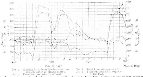
Fig. 24. Curve 4 shows total wattless kv-a. required at different periods of the day: Curve 1 is the amount automatically supplied by the synchronous condensers, while the remaining amount is furnished by the other synchronous machines, their fields being hand regulated
