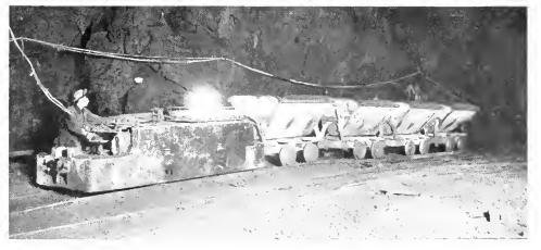
Fig. 11. 10 Ton Electric Mine Locomotive The United Engineering and Contracting Co., Pennsylvania Railroad Crosstown Tunnels, New York City
