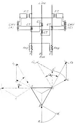
Fig. 5. Two Single-phase Regulators on 3-phase System. Connections similar to those of Fig. 2
