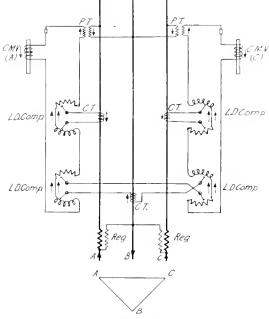
Fig. 11. Two Single-phase Regulators on Two-phase 3-wire System
