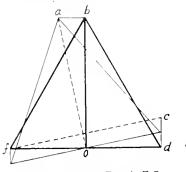
Fig. 18. Reactance Drop in T Connected Transformers, 2:Phase Primary. Perfect interlacing and equal per cent reactance in main and teazer.
