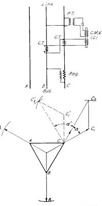
Fig. 2. One Single-phase Regulator on 3-phase System. Current Transformer in each Leg of Phase
