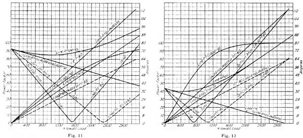
The curves illustrate the relation of the kilowatt load to the line current, power-factor, and line wattless current, when the voltage drop is maintained constant. Two conditions of load are assumed, one at 0.60 p-f. and the other at 0.80 p-f., and the two corresponding curves of wattless current are given, these being designated "syn. con. amps."
