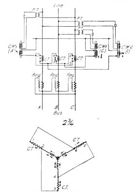
Fig. 8. Three Single-phase Regulators on 3-phase System, employing three current transformers instead of six as shown in Fig. 7
