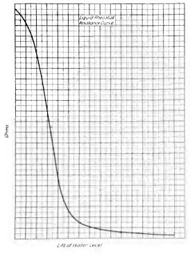
Fig. 4. Liquid Rheostat Resistance Curve
