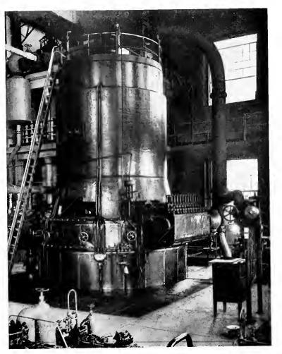
Fig. 2. 9722 Kv-a. Mixed-Pressure Curtis Turbine
