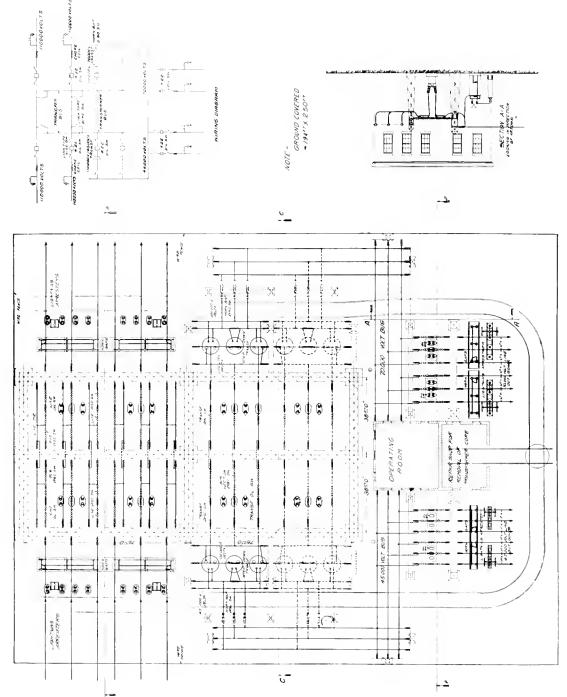
Fig. 1. Plan of Outdoor Substation for 110,000/45,000 Volt Circuits
