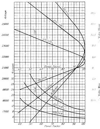
Fig. 10. The Above Curves Illustrate the Effect of Powerfactor on the Generating Voltage at Different Loads for an Equivalent High Tension Receiving Voltage of 21,000 Volts. In the Lower Part of the Figure, Power-factor is Plotted Against the Per Cent of Energy Losses. Fig. 9 is the System for Which These Values Obtain
