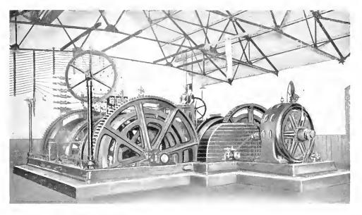
Fig. 10. 300 H P., 440 Volt, 250 R P.M. Motor Driving Four-Drum Hoist For A and B Shafts, Harmony Mine
