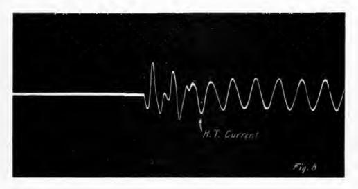
Fig. 8. Switching on 150 miles of 100,000 volt transmission line by high-tension switches. Wave of high-tension current
