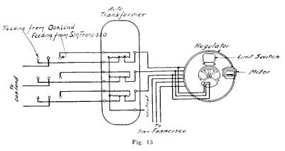
Fulsom station. Ordinarily, the outgoing voltage from the regulator was 11,500, this being the normal operating voltage of the Fulsom station. The regulator was set to automatically maintain the desired voltage at San Francisco.
