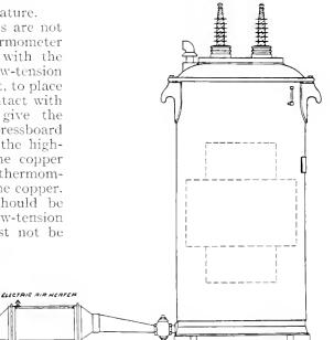
Fig. 3. Hot Air Drying Outfit for Drying Transformers
