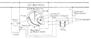
Fig. 5. Regulator for Controlling Speed of Shunt Wound Motors
