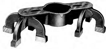
Fig. 7. Crosshead for 3000 Ampere Oil Switch Cast from Pure Deoxidized Copper
