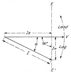
Fig. 1. Relation of Wattless Current to Power-factor and Actual Current Assuming Kilowatt Output and Voltage Constant
