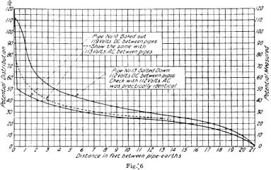
applied. These curves illustrate the value of salt water around the pipe-earths.
