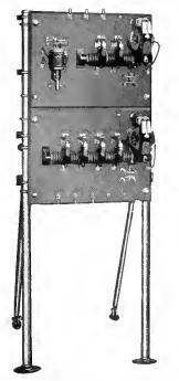
Fig. 3. Automatic Compensator Panel for Squirrel Cage Induction Motors
