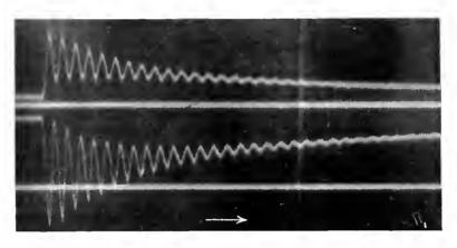
Fig. 9 (With Fig. 8) Upper Curve, Field Current; Lower Curve, Field Voltage
