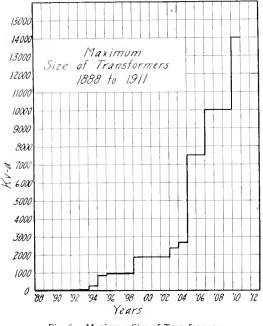
Fig. 6. Maximum Size of Transformers
