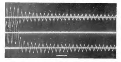
Fig. 10. Single-Phase Short-Circuit (on Phase B-C) on 25 Cycle Turbo-Alternator. Upper Curve, Voltage of Phase A to Neutral; Middle Curve, Voltage of Phase B to Neutral; Lower Curve, Current
