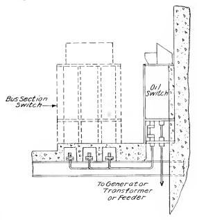
Fig. 4. Compartment Design for Small Substations or Power Houses
