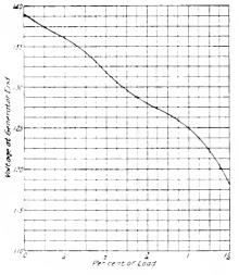
Fig. 7. Voltage Characteristic of Battery Charging Motor-Generator Set
