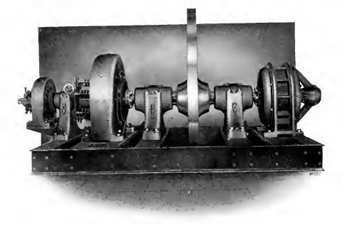
Fig. 7. 90 Kw., 500 Volt Generator Direct Connected to 75 H.P. 440 Volt Induction Motor, Kendall Gold Mines
