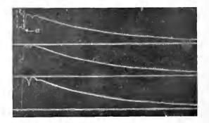
Fig. 7 Impulse Traveling Over Line. Receiver End Short Circuited. Upper curve, current at generator end of line; middle curve, current at middle of line; lower curve, current at receiver end of line.
