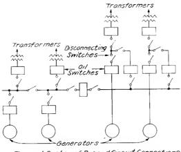
Typical System of Busand Circuit Connections
