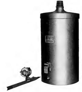
Fig. 2. Ammeter, Stick and Jack for Measuring the Charging Current in an Aluminum Arrester
