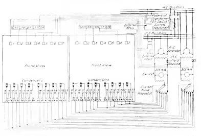
Fig. 4. Connections of Two Automatic Voltage Regulators Operating in Parallel with One Arrangement of Two Exciters not in Parallel
