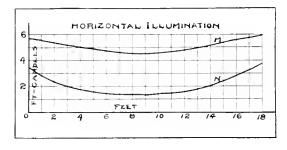
Fig. 3. Illumination Curves. N, Old Installation; M, 400 Watt Mazda Installation
