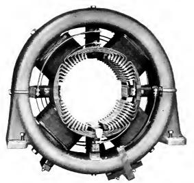
Fig. 7. 500 Kw. Field Frame Showing Compensated Windings
