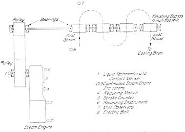
Fig. 3. Arrangement of Four Finishing Stands of 11 in. Rod Mill
