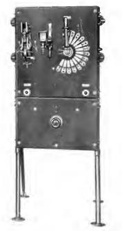
Fig. 1. Hand-operated Dial Controller used [with direct current single motor semi-automatic printing press equipments. Push button jog; push button stop; no-voltage release; overload release; dynamic brake; slow speed; armature and shunt field regulation are provided.
