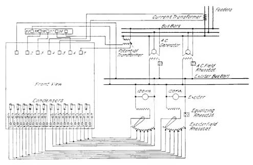
Fig. 1. Connections of Automatic Voltage Regulator with One Arrangement of Two Exciters in Parallel
