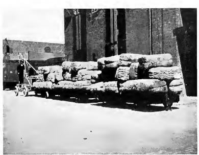
Fig. 8. Battery Truck Crane and Trailers Trafficking Between Piers, Bulkhead and Warehouses
