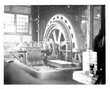
Fig. 9. 1000 H.P. Induction Motor Driving 20 in. Bar Mill
