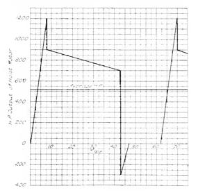
Fig. 2. Load Curve of Mine Hoist
