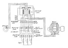
Fig. 2. Wiring Connection for Compensator Shown in Fig. 1
