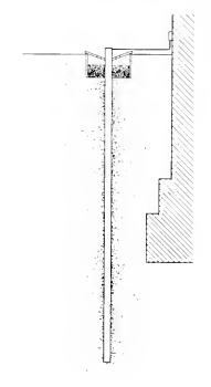
Fig 1. Illustration of a Single Pipe-Earth, containing all the essential features of a good earth connection. To avoid voltaic action the copper connecting wire at the top is not brought to the wall underground through the salt solution
