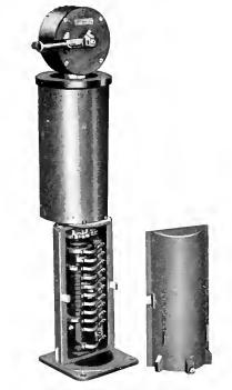
Fig. 3. Master Controller for Ammunition Hoist Motor
