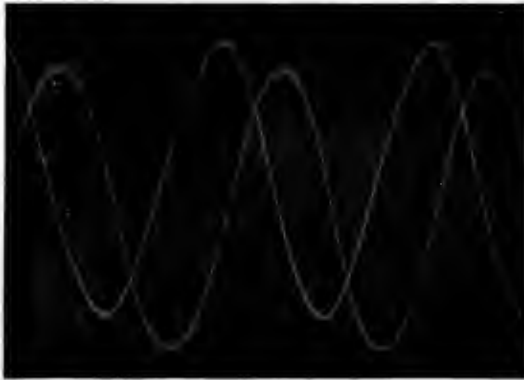
Fig. 14. Upper Curve: Potential of Phase 3 Power Line to Ground. Lower Curve: Induced Potential on Telephone Circuit 5600 volts
