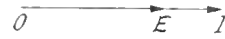
Fig. 4. Vector Diagram showing the current drawn by an induction motor adjusted by a phase advancer to be in phase with the line voltage, i.e., motor operating on unity power-factor
