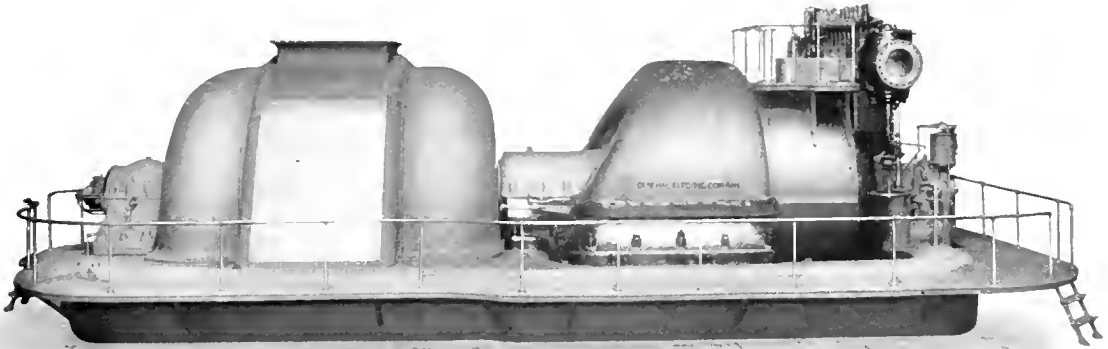
Fig. 4. 12,500 Kw. Horizontal Curtis Steam Turbine
