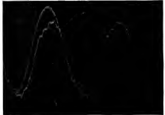
Fig. 11. Upper Curve: Line Potential Phase 2. Lower Curve: Current in Ground Connection of Drainage Coil
