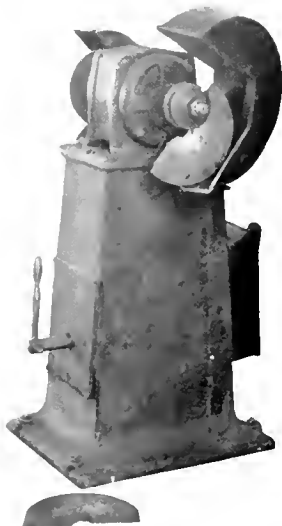
Fig. 7. Broken Emery Wheel. The workman was protected by the guard when the wheel exploded
