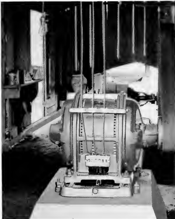
Fig. 13. 35 H.P. 1200 R.P.M. Constant Speed Motor Driving the Power-head for Pumping 23 Jack-wells in the Kern Field, Bakersfield, Cal.
