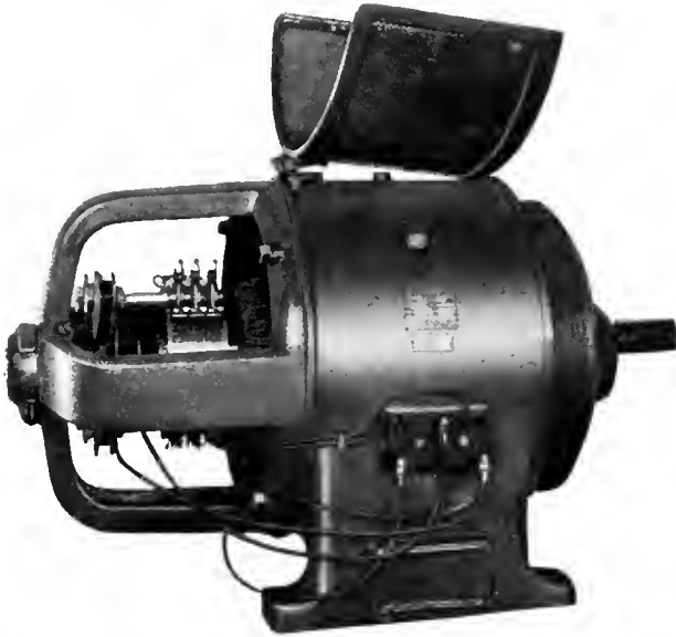
Fig. 3. Standard Type of Planer Motor. Rated 35 h.p., 250/1000 r.p.m., 230 volts. The planer is one of the more recent to which the adjustable speed motor has found application
