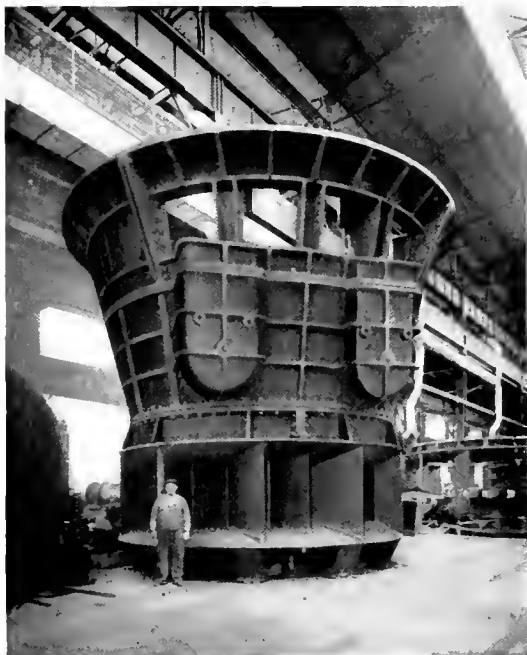
Fig. 3. One of the Four 17,500 h.p. Turbines Designed and Built by the I. P. Morris Company for the Alabama Power Company
