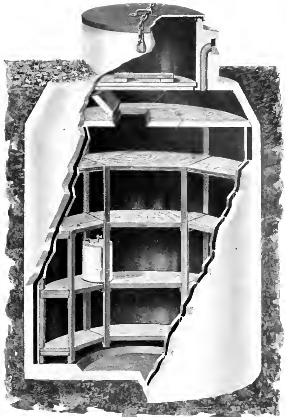
Fig. 4. Concrete Battery Wall
