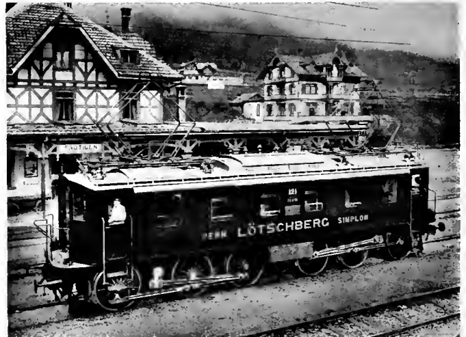
Fig. 14. Loetschberg Tunnel. Experimental locomotive. Motors geared to jack shafts with side rod drive
