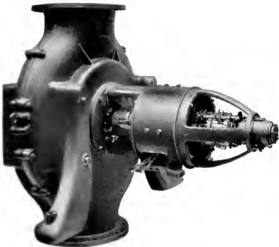
Fig. 4. A Centrifugal Compressor Driven by a Direct-Connected 30 H.P., 230-Volt Direct-Current Motor
