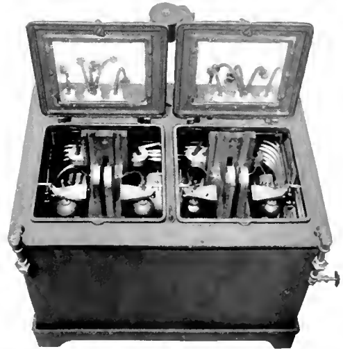
Fig. 9. Tube Tank for Duplicate Two-Tubes-in-Series Mercury-Arc Rectifier, Showing Internal Construction of Tank. No Oil
