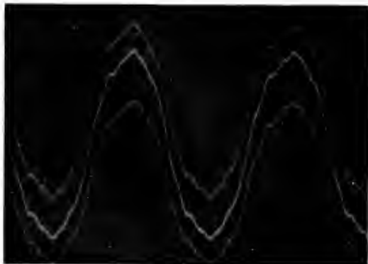
Fig. 10. Upper Curve: Current in One Wire of Telephone Line 0.8 amp. Middle Curve: Current in Other Wire of Telephone Line 0.8 amp. Lower Curve: Current in Ground Connection of Drainage Coil 1.6 amp. Record taken while Lightning Arresters were being charged
