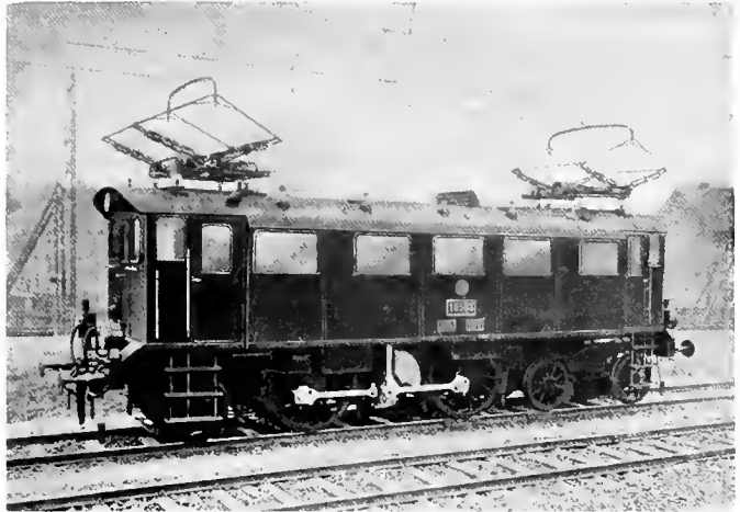
Fig. 1. Dessau-Bitterfeld Experimental Line. High speed passenger locomotive. Side rod drive with vertical connecting rods
