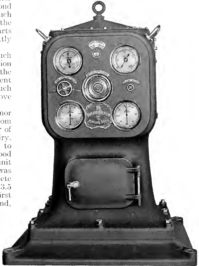
Fig. 8. The Type of Turbine Governor used in the Mississippi River Power Company's station at Keokuk
