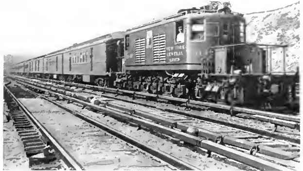
Fig. 11. New York Central Locomotive, 600 Volts, Hauling 12-Car Train
