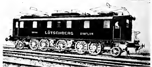
Fig. 15. Loetschberg Tunnel. Accepted type of locomotive. Motors geared to jack shafts coupled with Scotch yoke and side rods
