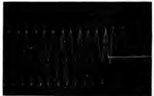
Fig. 8. An Oscillogram made at the time of interrupting a 1720 kv-a. charging current by an Oil Switch
