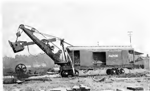
Fig. 3. A Sixty-Five-Ton Electric Shovel equipped with four 550-volt direct current series motors
