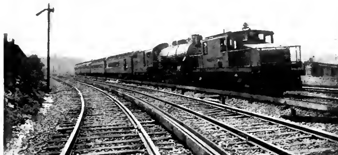
Fig. 6. One 100-ton Freight and Passenger Locomotive, Type OE-1 and OE-2, equipped with four GE-209 Motors hauling passenger train
