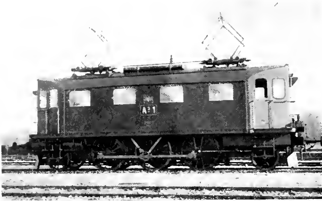
Fig. 8. Baden State Railways. Later type of express locomotive with "double rod" drive without jack shafts
