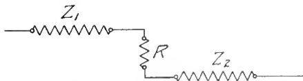
Fig. 22. Resistance, R , connected between circuits of impedance, Z_1 , and circuit of impedance, Z_2 :
