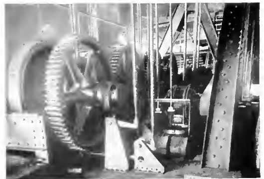
Fig. 5. Eight-Drum Swing Winch
