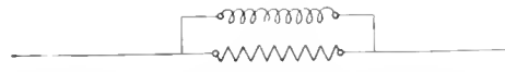
Fig. 24. Series resistance shunted by choke coil to afford low impedance to currents of low frequency, and high impedance to currents of high frequency
