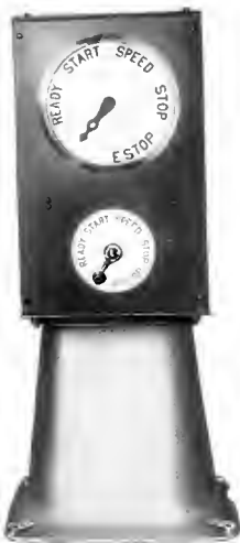
Fig. 24. Pedestal Containing Transmitter and Receiver, Located near Generator
