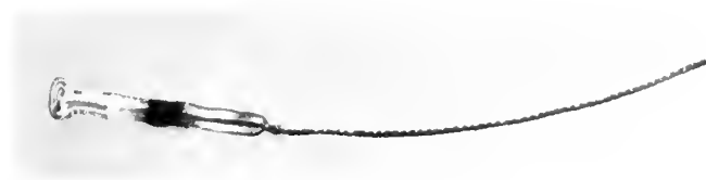
Fig. 3. Graded Glass Seals with Tungsten Leading-in Wire
