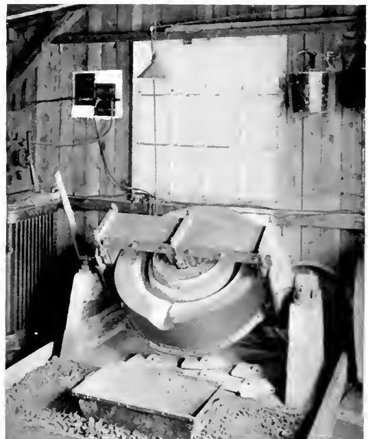
Fig. 7-A. Induction Furnace assembled complete with crucible. Cover plates shown beneath furnace
