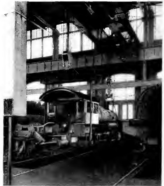
Fig. 6. A 120-Ton Electric Crane in Use in a Locomotive Shop
