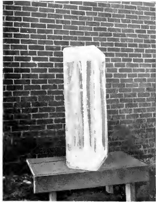
Fig. 4. Another illustration of the cake of ice shown in Fig. 3. The central core which here appears to have considerable width would be only of line width in an edge-on view.
