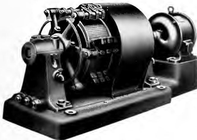
Fig. 7. A Rotary Phase Advancer designed for raising the power-factor of a 400 h.p. induction motor
