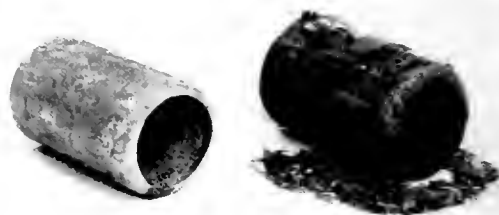
Fig. 2. Effect of 800° C. in a Gas Furnace for 100 Hours on a Section of Calorized and of Uncalorized Sheet Iron Tubes
