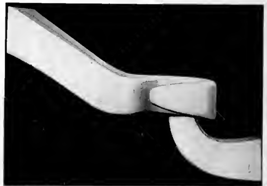
Fig. 3. Photograph of the Model of Water Column of a 20,000 h.p. Water Turbine
