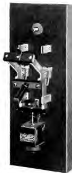
Fig. 1. An Interlocking Lever Switch for Automatically Connecting a Reserve Source of Current to the Mains on failure of the Normal Supply
