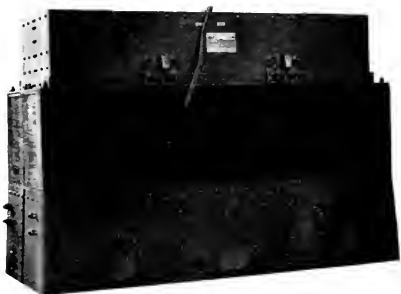
Fig. 8. A 20,000-kv-a., 8100. 14000-4050 7000-volt Shell Type Air Blast Auto-Transformer
