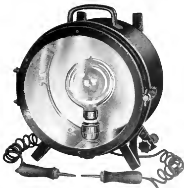
Fig. 14. A Portable Interurban Type Headlight Having the Same Casing as that Shown in Fig. 12 but Having a Shallow Parabolic Glass Mirror Reflector
