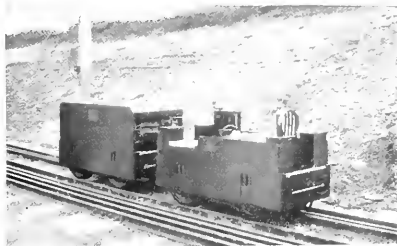
Fig. 12. Four-ton Storage Battery Locomotive with Storage Battery Trailer Truck
