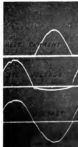
Fig. 13. Rectifier Containing an Active Purifying Agent. Voltage Across Arc Gap 29.6 Amperes Direct-Current Flowing
