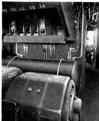
Fig. 10. Interior View of the Locomotive Illustrated in Fig. 7, Showing the Dynamotor Blower Set, Contactor Bank, and Rheostat Compartment all in the Apparatus Compartment
