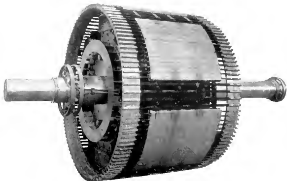
Fig. 4. Rotor with unusually heavy squirrel-cage winding, continuous between poles. Well adapted for operating on unbalanced system, 7000-h.p., three-phase, 25-cycle, 13200-volt, with peripheral speed of 10100 ft. per min.
