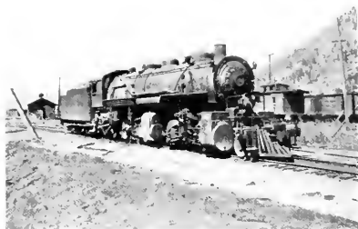
Fig. 7. Type of Mallet Locomotive Used for Freight Service
