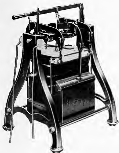
Fig. 8. Regulating Apparatus Used in Conjunction with the Transformers Shown in Figs. 9 and 10
