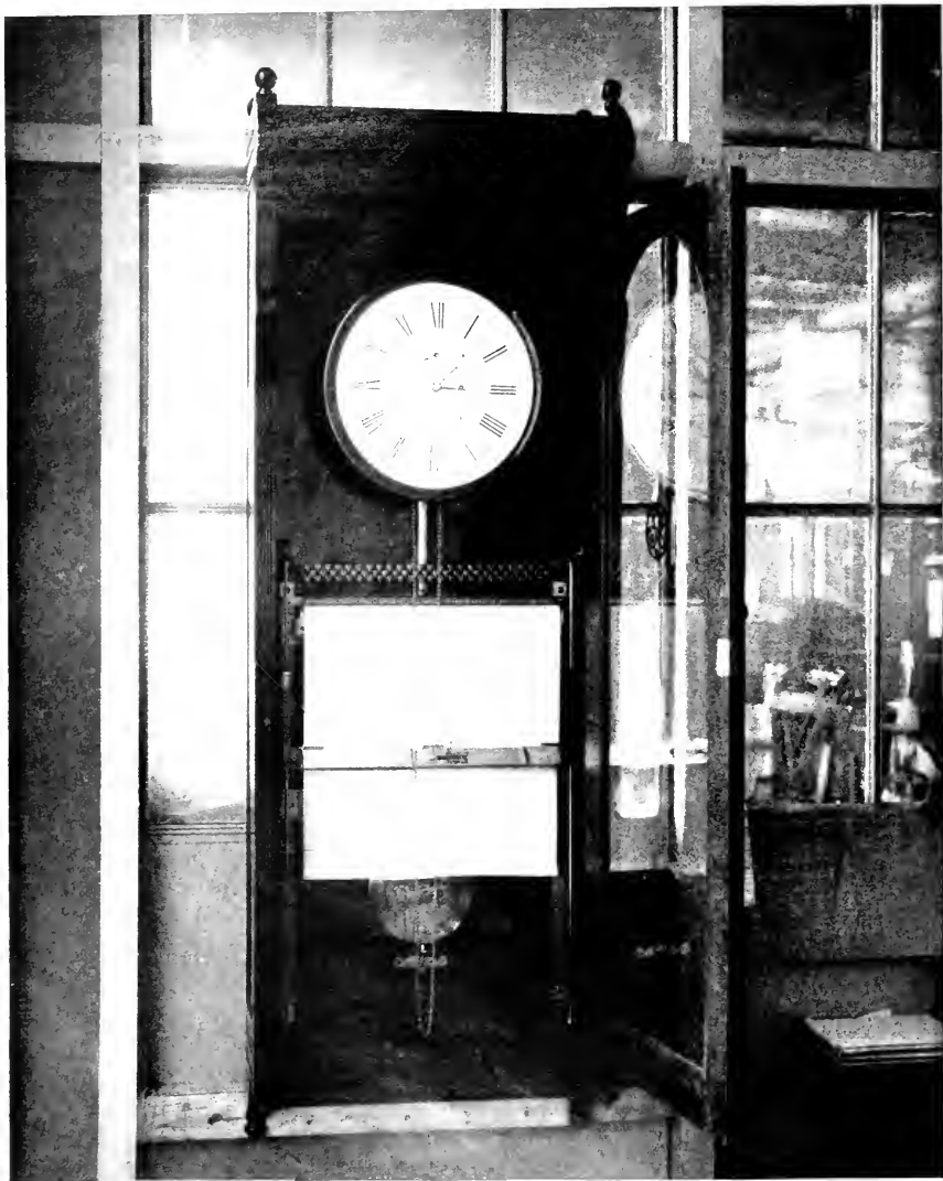
INDUSTRIAL MULTIPLE RECORDER
