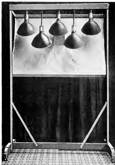
Fig. 7. Rear View of Mazda Lamp Artificial "Skylight"
