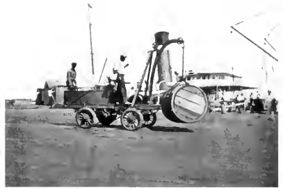
Fig. 4. Moving 1800 lb. Tobacco Casks 1000 ft. Cars to Ship's Side
