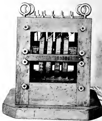
Fig. 3. Amplifier Coil Used for Tests
