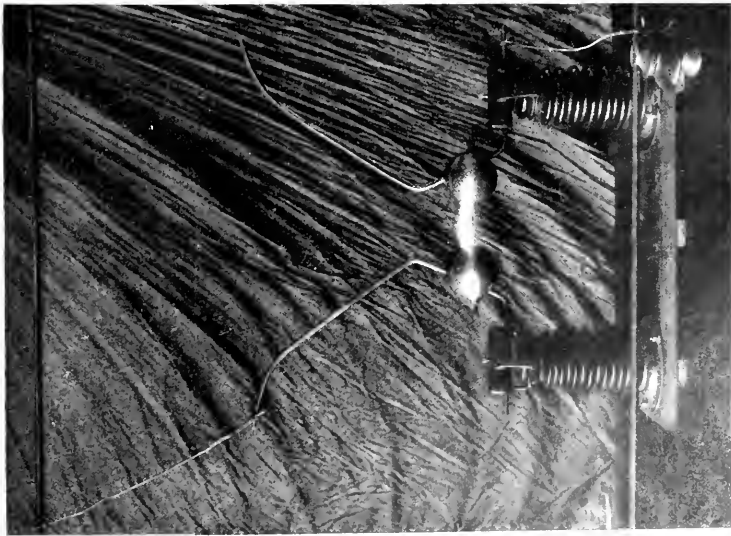
Fig. 18. Sphere and Horn Gaps having a Steep Wave front Voltage Applied
