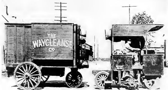
Fig. 5. Tractor and Trailer Uncoupled
