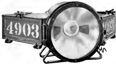
Fig. 19. The Type of Electric Headlight Used on the Canadian Northern Railroad
