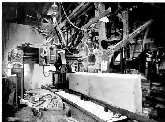
Fig. 9. 440-volt, 3-phase, 60-cycle Induction Motor geared to a Carborundum Attachment on a Single Circular Planer
