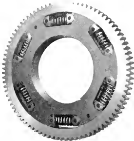
Fig. 15. Spring Gear used on Chicago, Milwaukee & St. Paul Locomotive
