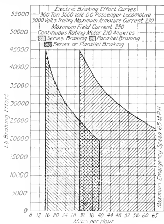
Fig. 8 Electric Braking Effort Curves of 3000-volt D-c. Passenger Locomotive Showing Wide Range in Braking Speeds
