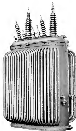
Fig. 14. Transformer designed for operation as either a self-cooled or a water-cooled unit for outdoor installation. Where heavy overloads for extended periods are expected such designs are invaluable for increasing flexibility of large central stations.
