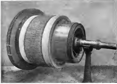
Fig. 7. Generator Armature of Set Shown in Fig. 1 Showing Double Section of Fan
