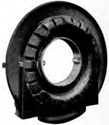
Fig. 8. Air Distributing Chamber Showing Nozzles for Forcing Streams of Air Over Surface of Armature
