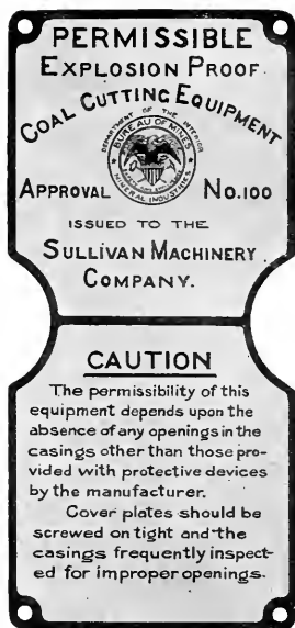
Fig. 1. The Permissibility Plate that is Attached to Explosion-proof Coal Cutting Equipment
