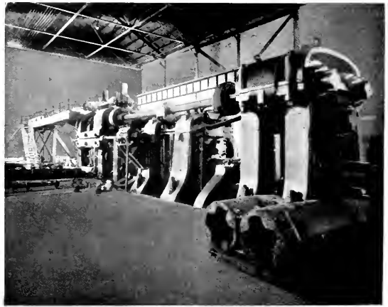
Fig. 8. Main Rolls of Universal Plate Mill Driven by Induction Motor shown in Fig. 7
