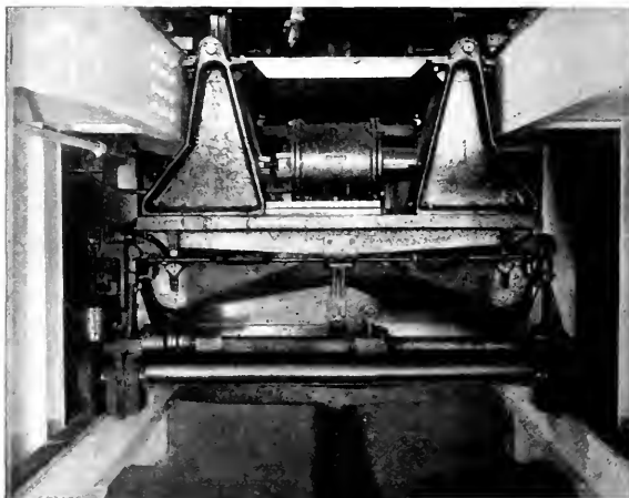
Fig. 4. End View showing Scale and Lifting Mechanism
