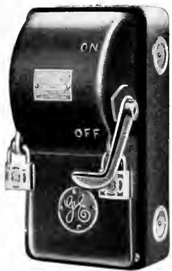
Fig. 1. 250-volt, 60-ampere, Double and Triple-pole Single-throw Safety First Enclosed Lever Switches. Double-Pole Switch Locked "Off" and Fuse Cover Locked Closed; Triple-pole Switch in "Off" Position and Fuse Cover Open
