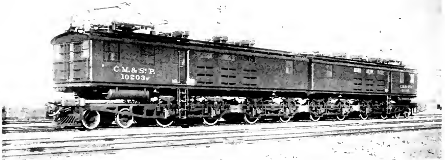
Fig. 14. Transcontinental Type 3000-volt Direct-current Electric Locomotive for Chicago, Milwaukee & St. Paul Railway
