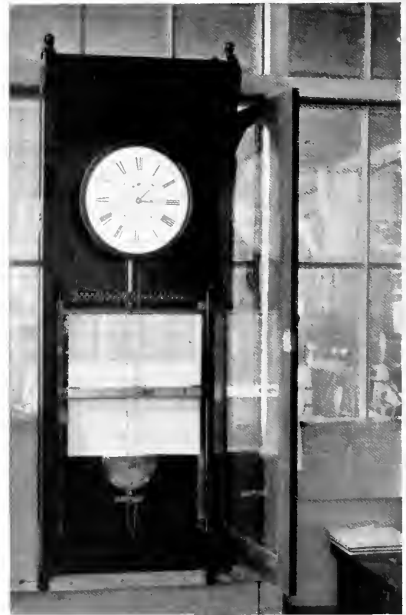
Industrial Multiple Recorder
