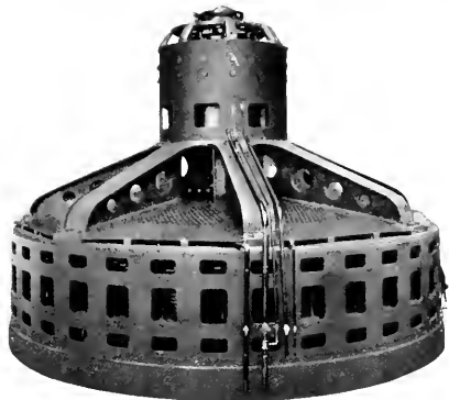
Fig. 6. 72-Pole, 3750-Kw., Three-Phase, 60-Cycle, 6600-Volt, 100-R.P.M. Generator with Self-Contained Exciter
