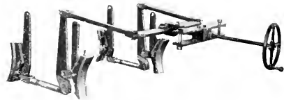
Fig. 8. Horizontal Screw Type Brake Rigging for Inside Frame Type of Locomotive
