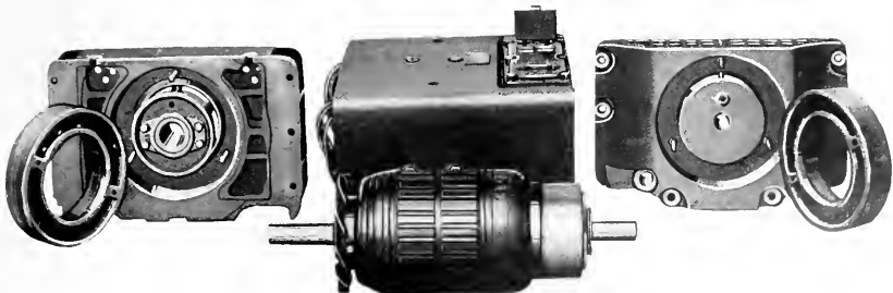
Fig. 4. The Motor shown in Figs. 2 and 3 Disassembled, showing Mufflers
