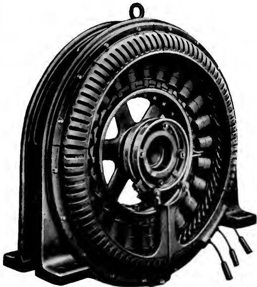
Fig. 3. 24-pole, 50-kw., 2300-volt Revolving Field Alternator
