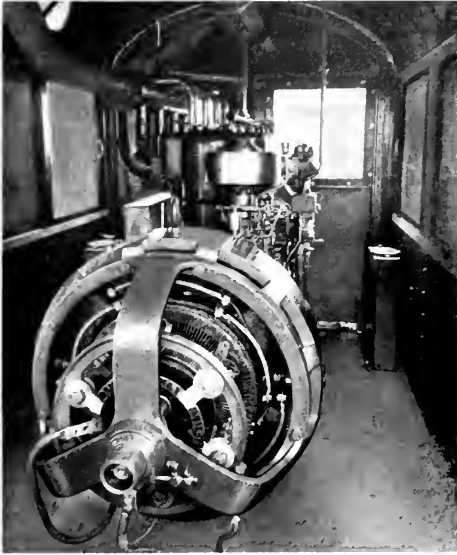
Fig. 18. View in Cab of Gasolene-electric Locomotive Showing Self-contained Power Plant from Generator End
