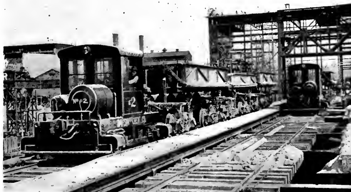
Fig. 16. Two 20-ton Locomotives Hauling Trips, Showing the Over-running Third Rail and Current Collectors
