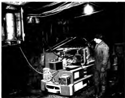
Fig. 19. 4-ton Storage Battery Locomotive Shown in Fig. 18 Receiving a Charge During Noon Hour
