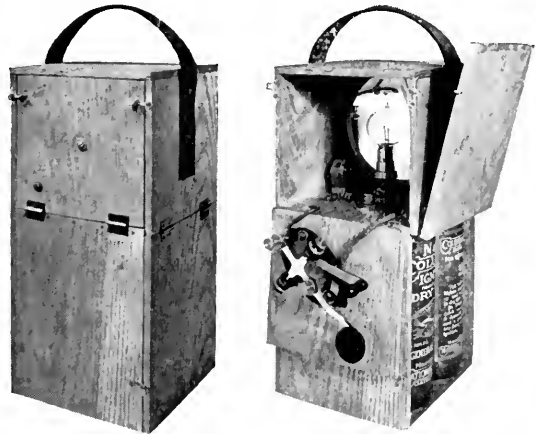
Fig. 12. Simple Signal Projector having a Range of 25 Miles. Fitted with 5-in. Mangin Mirror, 6-volt 12-c.p. Mazda C Lamp
