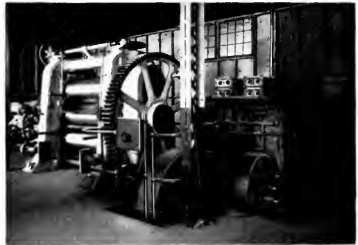
Fig. 31. Motor-driven Rubber Calender Equipped with Automatic Push Button Control
