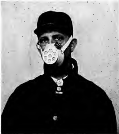
Operator wearing respirator which is used in places where ventilating or exhausting systems can not successfully remove injurious dust
