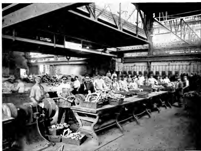
Safety Work at the Erie Plant. The grinding machines are fitted with guards and the men are impressed with the need for wearing Goggles to shield the eyes from flying particles
