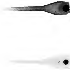
Fig. 9. Lower, Roentgenogram of Hooded Target; Upper, Roentgenogram of Target of Standard Tube
