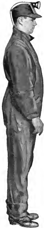
Fig. 3. General Electric Miners' Lamp Properly Worn by Miner (Battery Box Under Jumper)
