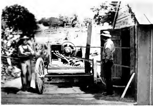
Fig. 10. 20-h.p. portable motor equipment for pulling oil wells of the Badger Oil Co., Hosston, La.
