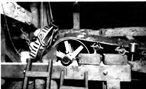
Fig. 11. 36-inch Electromagnet for Extracting Pieces of Steel from Ore before it Enters the Crushers
