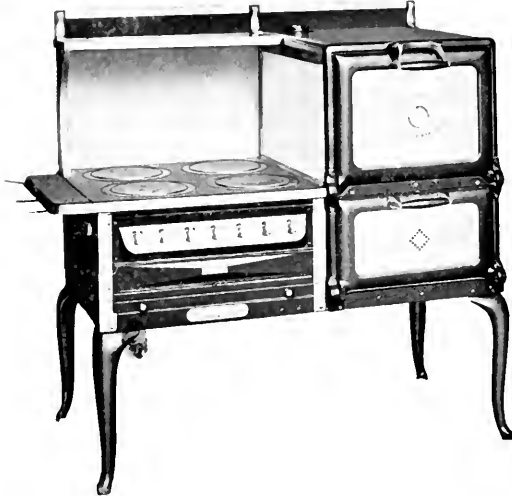
Fig. 3. Electric Range with Four Eight-inch Three-heat Hot Plates, Two Three-heat Oven Units, and a Three-heat Broiling Closet
