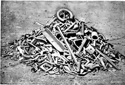
Fig. 7. Iron Caught by a 12-inch Magnet (Placed in Chute Back of Coal Dryer), between November 20, 1913, and July 16, 1914. The quantity was about one barrel
