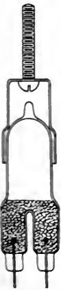
Fig. 7. Coherer which forms a part of Discharge Alarm and High-frequency Alarm Devices
