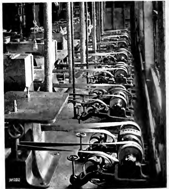
Fig. 12. Individual Drive. Note floor space and extra mechanical parts
