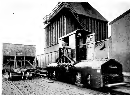
Fig. 14. Side View of "Pusher" Locomotive Showing Construction of Pneumatically Operated Pusher Arm
