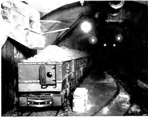
Fig. 15. Loading Ore Cars in Mine. Tail Lamp Consists of Edison A4 Cell and Incandescent Lamp Mounted in Iron Box
