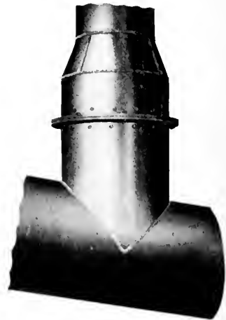
Fig. 16. Section of a Smoke Stack. Seams Welded by Electric Arc Welding Process. Metal \frac{1}{4} in. Boiler Plate
