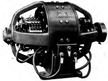
Fig. 26. 100-kw. 1200-r.p.m. 250-volt Three-wire Synchronous Converter
