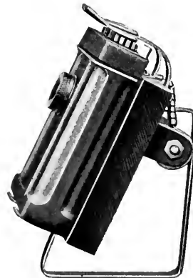
Fig. 10. Battery under Contacts, Charging (Note Position of Contacts)
