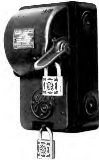
Fig. 32. Enclosed "Safety First" Lever Switch, 2-pole, 30-amp. 250-volt, Switch Locked Open, Fuse Compartment Locked Closed
