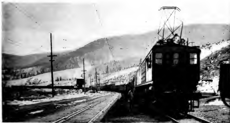
Freight train without helper on two per cent grade at Donald (Continental Divide)
