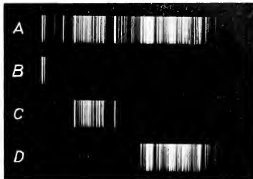
Fig. 1. (A) Spectrum of Iron Spark (B) Spectrum through Ruby Glass (C) Spectrum through Green Glass (D) Spectrum through Blue Glass
