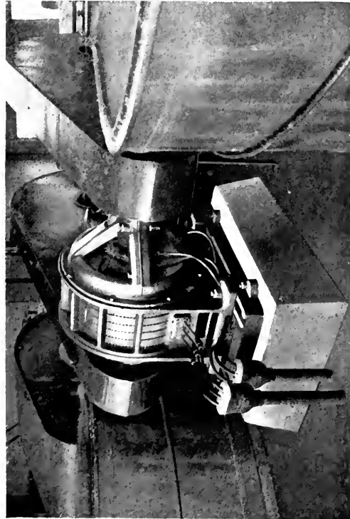
Fig. 9. 100-h.p., 480-r.p.m., 550-volt Slip Ring Induction Motor Driving Two Jones Beaters. Fenimore Mill, Union Bag and Paper Corporation, Hudson Falls, N. Y.
