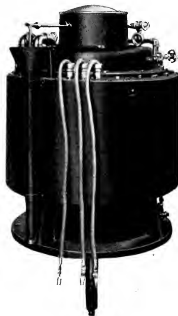
Fig. 7. 150-h.p., 1845-r.p.m., 440-volt Squirrel Cage Totally Enclosed Water-cooled Motor for Driving Unwatering Pump. Iron & Silver Mining Co., Leadville, Colo.
