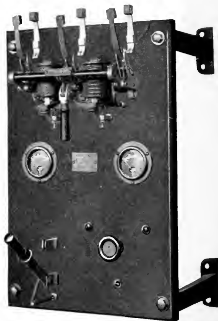
Fig. 15. Individual Vehicle Charging Panel with Automatic Protection for use when ampere-hour meter is installed on the vehicle
