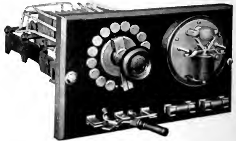
Fig. 11. Series-rheostat Section with Automatic Protection Device
