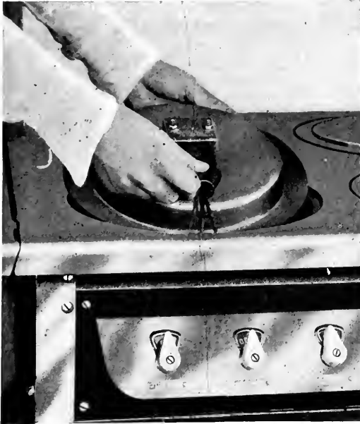
Fig. 6. Method of Attaching Plug to Hot Plate
