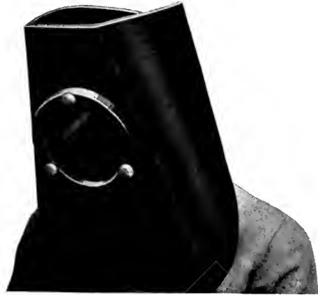
Helmet used by arc welders, provided with windows of special glass which shield the operator not only from injurious light rays but also from the heat rays
