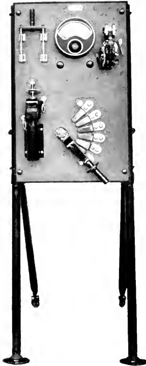
Fig. 22. Auxiliary Arc Welding Panel
