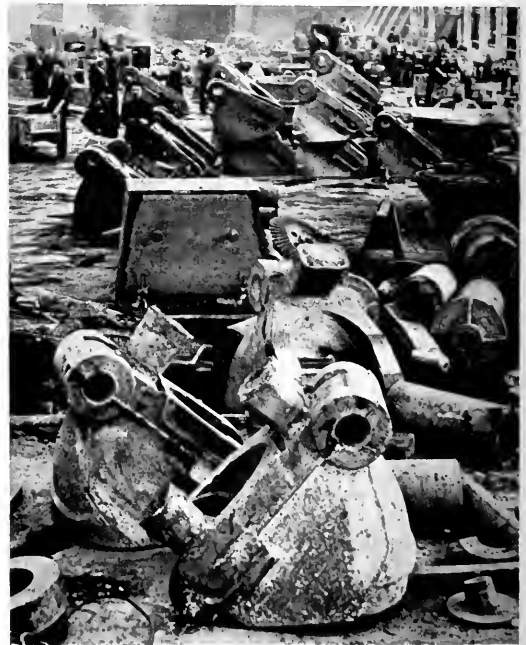
Fig. 8. Castings in Shops Showing Heavy Risers Cut by Electric Arc
