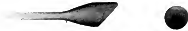
Fig. 17. Right, Roentgenogram of Target of Tube shown in Fig. 16; Left, Broadside View of Target for Comparison
