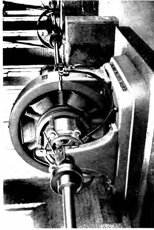
Fig. 21. One 100 225-h.p., 275 500-r.p.m., 220-volt Variable Speed Direct Current Motor direct-connected at both ends to line shafting driving variable speed end of paper machine. Consolidated Water Power and Paper Company, Grand Rapids, Wis.
