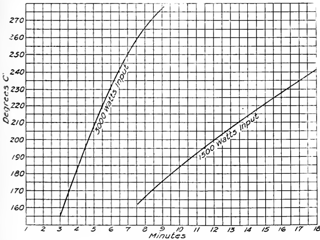
Fig. 12. Time to Preheat a Standard Oven 18 Inches by 18 Inches by 14 Inches
