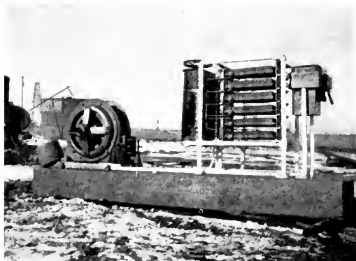
Fig. 7. A two-speed oil well motor equipment in Kansas, mounted on skids and completely wired ready for final location at a well near El Dorado
