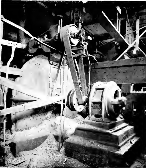
Fig. 5. 15-h.p., 750-r.p.m., 440-volt Form K Induction Motor driving 5-ft. barker. Kimberly-Clark Company, Kimberly, Wis.
