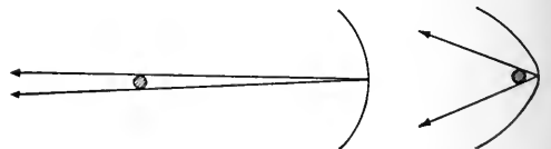
Fig. 4. Illustrating the Effect of Focal Length of Projector on Spread of Beam
