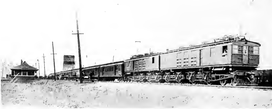
Fig. 3. Electric Locomotive Coupled to Passenger Train on the C., M. & St. P.
