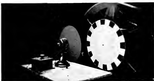
Fig. 3. Photographs Showing Arrangement of Apparatus for Measuring Angular Deviation
