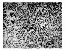
At weld, showing ferrite mass with irregular bands of carlade. Structure in transition stage, 150 diameters.
