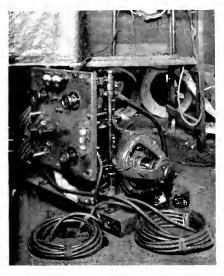
Fig. 6. Direct-current Portable Balancer Equipment
