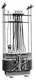
Fig. 6. Core-type 60-cycle, 750 kv-a., 24,000 2400-volt Trans former Showing Method of Bringing out Leads from Resistance Unit Embedded in Low-voltage Coit (Third from top)
