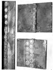
Fig. 2. Samples of: A 3-inch Angle Iron Spot Welded to a Halfinch Thick Plate; two 12 by 18 by 1-3-inch Thick Plates Welded in a Double Row Using Buttons (Thin Steel Disks) under the Electrode; and Similar Plates Welded in a Single Row Using Elongated Electrodes which make a Practically Continuous Weld.
