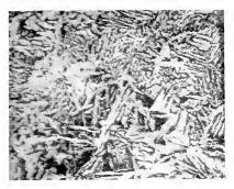
At weld, showing mass of ferrite with numerous plates of carbide. Structure in transition stage = 150 diameters.
