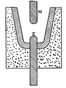
Fig. 37. Furnace with Metallic Hearth Electrode
