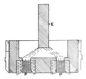
Fig. 39. Girod Furnace with Metallic Poles Embedded in Refractory Masonry
