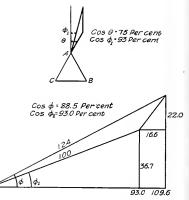
Figs. 16 and 17. Vector Diagram of Three-phase Feeder.
