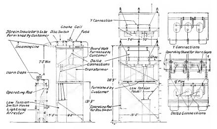
Fig. 4. Standard Outdoor Substation, steel structure mounted. three-phase, 45,000 volts maximum high tension, 2300 volts maximum low tension, 150 kv-a. maximum
