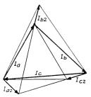
Fig. 13. Current Diagram of Three-phase Feeder
