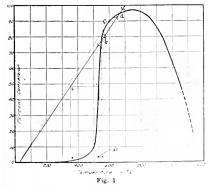
words, the shape of the "conversion curve" will change from convex to concave, and at a certain temperature which the writer understands is somewhere around 750 deg. C. the conversion will reach a maximum of nearly 100 per cent. Thereafter, the conversion will
