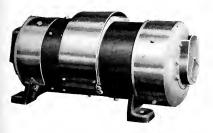
Fig. 2. Motor-generator Set for Interurban Car Lighting
