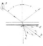
Fig. 11. Reflection and Transmission by Etched Glass
