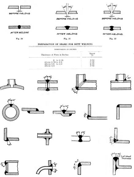
Fig. 33. Method of Making Various Types of Welds
