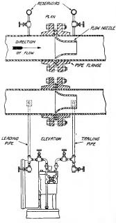
Fig. 3. Arrangement Diagram Showing the Method of Connecting the Flow Meter to the Flow Nozzle shown in Fig 2
