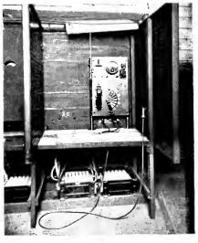
Fig. 3. Direct-current Resistance Welding Equipment
