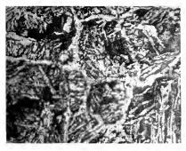
Close to weld, showing sorbitic grains with territe boundaries. 150 diameters.
