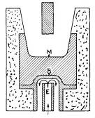
Fig. 38. Furnace with Metallic Hearth Electrode and Water Circulation
