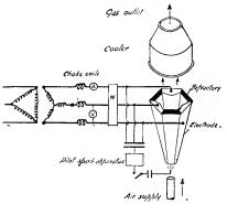
Fig. 7. Diagram of Kilburn Scott Three-phase Furnace
