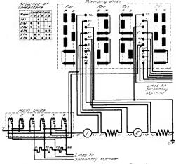
Fig. 4. Simplified Connections of Four-motor Controller
