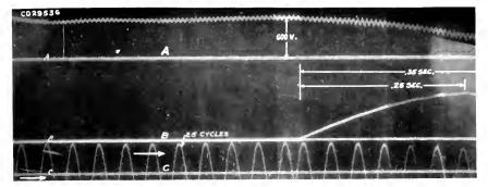
Fig. 14 Short Circuit on 300 kw , 600 volt, 25 evide Synchronical Converter Protected by A and the Re-Direct-current Circuit and Standard Circuit Breaker. Curve A voltage across and the Curve B, line current. Curve C collector ring voltage.
