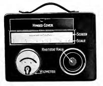
Fig. 86. Foot-candle Meter-Front View
