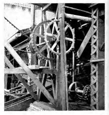
10-h.p. Back-geared Motor Driving an Excess Bagasse Conveyor. Central Santa Rosa
