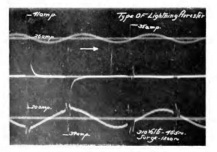
Fig. 2. Surge Discharge through Arrester Cell T-p vibrator -60-y-le timing wave Middle vibrator—courtent through arrester Bottom vibrator—voltage arross arrester
