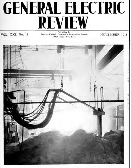
ELECTRIC FURNACES PRODUCING ARTIFICIAL ABRASIVES These electrochemical abrasives are much more effective than the emery formally imported from Turkey
