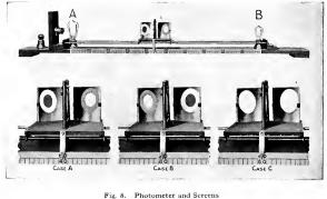
Case A—Screen at Left of Balance Point Case B—Screen at Right of Balance Point Case C—Screen at Balance Point
