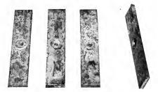
Fig. 4. Sample Plates with Hores Plugged by Spot-welding. At the right is shown a plate with plug in place previous to welding
