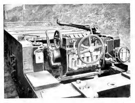
Fig. 6. Installation of Controller on Locomotive. Covers Removed
