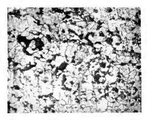
Close to weld, showing ferrite grains with normal pearlite areas. 150 diameters.
