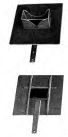
Fig. 3. Front and Back Views of Welder's Hand Shield
