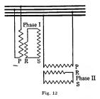
former having a primary winding P, a regulating winding R, and a secondary winding S. The windings P and R are fitted in between each other, so as to have only a small leakage between the two. Rand S are connected together. Let P and Shave the same number of turns, and the ratio of turns of R and S be c. Assuming as
