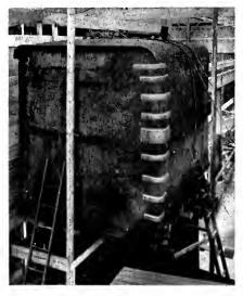
Fig. 25. Box Repaired and Under 15 lb. Hydrostatic Pressur All repairs were made with welding. Bolt holes shown are filled with welded in metal.
