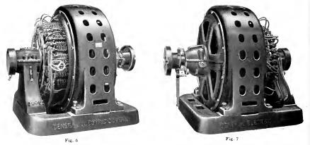
Two Views of a Single-phase, 25-cycle, 20-pole, 700-h.p., 300 r.p.m. Series Starting Motor having 30,000 ft-lb. starting torque
