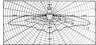
Fig. 2-a. Pendent Type Novalux Unit with Stippled Globe and Dome Refractor
