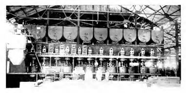
Twelve Induction Motor Direct Driven 40 In. by 24 In. Centrifugals. Central Violeta, Cuba. Some of the control panels are shown mounted between the motors. The master control switch is combined with the brake lever
