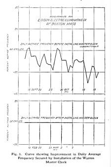
motors, and consequently the output of the mills, varies directly with the frequency. One half of 1 per cent would mean fifty dollars per day to a mill with a daily output of ten thousand dollars.
