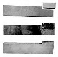
Fig. 6. Electrically Butt-welding High Speed Cutting Face to Machine Tool Shank
