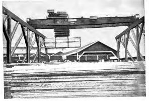
Overhead Crane used in Conveying Lumber from Transfer Cars to Tables in Front of the Planing Machines. Weyerhaeuser Timber Company.
