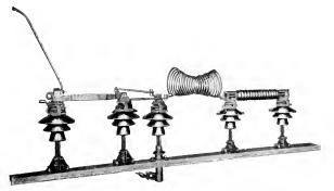
Fig. 10. Single-pole Combined Disconnecting Switch, hourglass choke coil and fuse, 45,000 volts maximum, 50 amperes maximum
