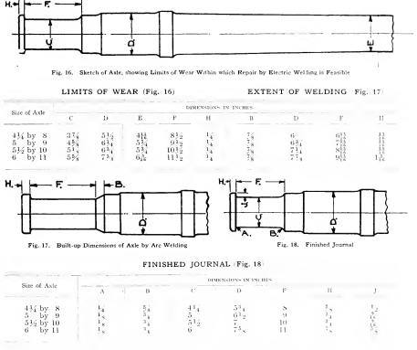
may be enough metal to allow the axles to be finished to conform to Fig. 18.
