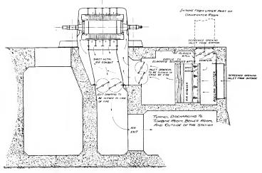
Fig. 3. Diagram of a Ventilation System for Turbo-alternator
