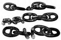
Fig. 9. Results of Static Tests on 2<sup>1</sup>4-in. Naco Electric Steel Links
