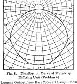
Lumens Output from Bare 200-watt Lamp—2920 Lumens Output from 200-watt Unit 1750
