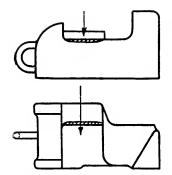
Fig. 20. Reclaimed Major Knuckle Locks by Electric Weld
