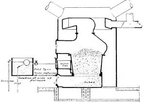
Fig. 1. Diagram showing Convenient Method of Keeping Water-pan Filled, also Conditon of Ashes which Should Not Exist
