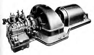
Fig. 2. 30,000-kw. 1800-r.p.m., 60-cycle Curtis Steam Turbo-generator
