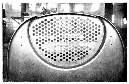
Fig. 10 Back Tube Sheet Welded to Head
