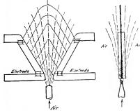
Fig. 5. Arc Flow in Relation to the Furnace of a Pauling Arc
