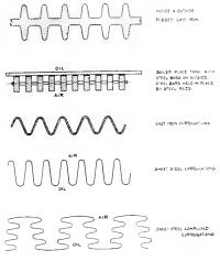
Fig. 1. Various Methods of Increasing Tank Surface
