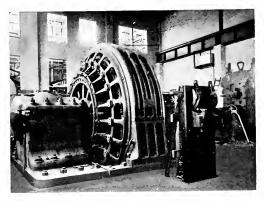
Fig. 32. 2500-h.p., 40 120-r.p.m. Motor-driving 36-inch Reversing Blooming Mill, Ashland Iron Mining Company, Ashland, Ky.
