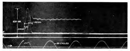
Fig 12 Short Circuit on 200 kw , 600 volt, 25-cycle Synchronous Converter Protected by Oil-cooled, High-speed Fuse Curve A, voltage across fuse, Curve B, line current, Curve C, collector-ring voltage
