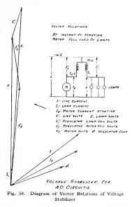
spondingly low voltage drop; Second, by inserting an air gap in the iron core the apparatus is made highly reactive and most of the drop over the motor coil is in quadrature with the line voltage, except for copper and core loss. These losses can and must be kept low in order to make the apparatus efficient.
