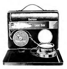
Fig. 87. Foot-candle Meter-Rear View
