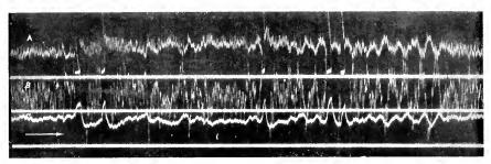
Fig. 4. Constant Potential System with Automatic Current Regulator and Variable Series Resistor Curve A Voltage across welding arc Curve B –Voltage across control magnet. Curve C–Current in Arc
