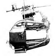
Fig. 2. Portable Electric Spot Welder with 27-in. Reach
