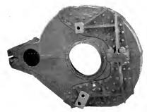
Fig. 9. Gear Housing on Which the Seams are Electrically Welded
