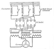
Fig. 20. Connection [Diagram for 3-phase Stassano Furnace. Provision is made to use high-voltage at starting, at which time a reactance can be connected in circuit
