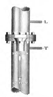
Fig. 2. Phantom View of Flow Nozzle Designed Primarily for Use with Flow Meters Measuring Dirty or Impure Water or Steam
