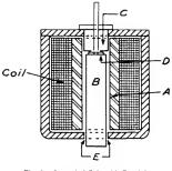
Fig. 2. Iron-clad Solenoid, Special Retarding Construction
