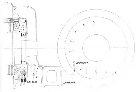
Fig. 3. Diagram showing Suggested Arrangements of Steam Jets
