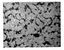
At weld, showing mass of ferrite grains with nearly normal pearlite areas. 150 diameters.
