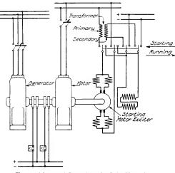
Fig. 10. Diagram of Connections of a Series Motor showing switch to make the machine function as a direct-current exciter when up to speed
