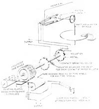
Fig. 6. Diagrammatic Sketch of Recording and Printing Demand Meter Type c
