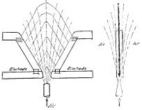
Fig. 12. Sketch showing Principle of Pauling Furnace
