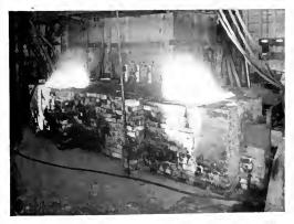
Fig. 3. Resistance Furnace in Operation. Making Special Carbides The flames show gases burning above contact area between electrodes and charge
