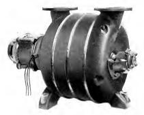
Small Three-stage Centrifugal Air Compressor with capacity of 250 to 350 cubic feet per minute at  $1^{1}_{2}$  lb. per square inch. This type of machine can supply the primary air to pulverized coal burners at any pressure from one-half lb. to 3/1 ib. per square inch, by varying the number of stages from 1 to 6. The power required is from 2 to 8.5 h.p.
