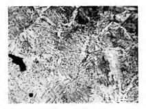
Fig. 13. Edge of Weld Made with Covered Electrode showing Coarsening of Grain in Plate Stock by Overheating (unannealed)
