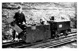
Fig. 18. 2-ton, 20-inch Gauge Storage Battery Locomotive with Battery Carrying Trailer
