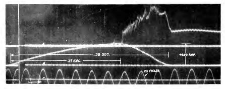
Fig 13 Short Circuit on 200 kw., 600 volt, 25 cycle Synchronous Converter Protected by Air-core Reactor in Direct current Circuit and Standard Circuit Breaker. Curve A: voltage across circuit breaker. Curve B, Inte current, Curve C, collector-ring voltage
