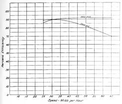
Fig. 4. Efficiency Curves of Present Geared and New Gearless Chicago, Milwaukee & St. Paul Locomotive
