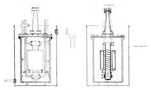
Fig. I. Small Vertical Vacuum Furnace
