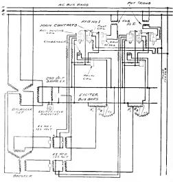
Fig. 5 Connections of Phase-balancer Regulator
