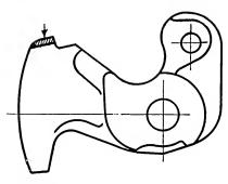
Fig. 19. Reclaimed Major Knuckle by Electric Weld
