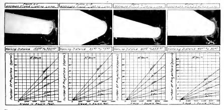
Fig. 1. General data on floodlighting projectors for high-intensity illumination. Working distances are given for convenience in , selecting the proper floodlighting projector. Local conditions may necessitate a change in some cases
