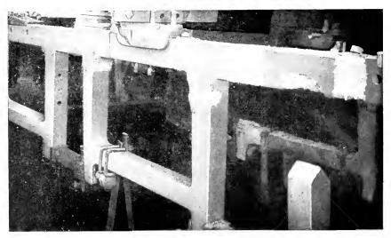
Fig. 4 Left Side Frame of Locomotive; Break Partially Prepared for Welding; Rubbed Spots Built up and Cracks Chipped out and Welded; Electric Arc Process Used
