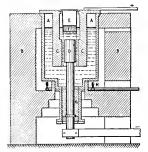
Fig. 1. Castner Sodium Furnace A, Cast-iron pot set in brickwork B; C, Nickel anode; D, Cathode; E, Metal cylinder receptacle for sodium; F, Liberated sodium.
