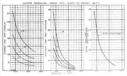
Fig. 2-c. Calculated Illumination Values on Street Surface along Center Line of Street
