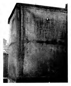
Fig. 24. Break in Corner of Box at 43 lb per Square Inch Pressure. The corner angle was bent considerably before the joint gave was. It is difficult to calculate the strain in the joint at rupture on account of the composite nature of the stress, but it was probably in the neighborhood of 50,000 lb, per square inch.
