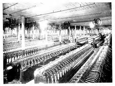
Fig. 3. Slubbers and Roving Frames Well Illuminated by a General Lighting System 500 watt Mazda C lamps in dome shaped enameled steel reflectors are placed close to the 18 ft ceiling on centers 24 by 33 ft. One can work efficiently in any part of the room
