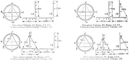
Fig. 7. Connections of Synchronous Converter with Core-type, Two-phase, or Three-phase Transformers
