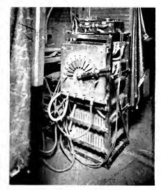
Fig. 4. Alternating-current Welding Transformer Booths and Various Types of Welding Equipment in use at the Emergency Fleet Corporation Welding School at Schenectady, N. Y.
