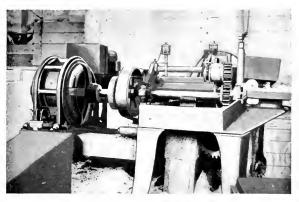
5-Saw Lath Mechine Driven by a 35-h.p., 3600 r.p.m., 550-volt Direct-connected Induction Motor. Weyerhaeuser Timber Company
