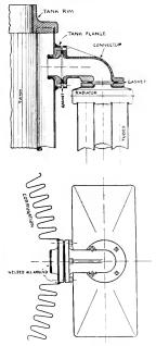
Fig. 3. Method of Attaching Radiator to Corrugated Tank
