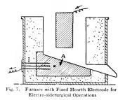
trodes are prismatic, M, a certain number being provided in close proximity to each other. They are placed upon a heavy iron plate f, which is in turn connected with an electric cable. The upper part of M forms the hearth level, carbon e being packed tightly around in order to properly close the joints. This arrangement has been adopted in various aluminum smelters.
