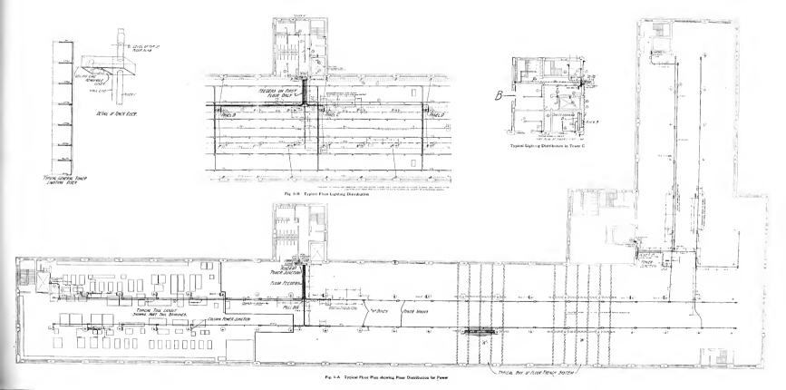
copper is No. 4/0, all riser copper 300,000 c.m. The necessary average amount is ordered and installed where required. Over some dead areas no copper will be necessary —over manufacturing areas the average watts per sq. foot may rise to 4.5 or even more.
