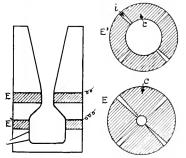
Figs. 11 and 12. Conley Furnace with Circular Electrodes (Vertical Cut and Cross-section of Electrodes)
