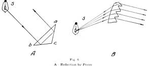
A Reflection by Prism B Refraction by Prisms
