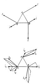
Figs. 14 and 15. Current Diagram of Three-phase Feeder
