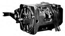
Light Weight, 25-h.p. Motor Designed for the Light-weight Safety Car
