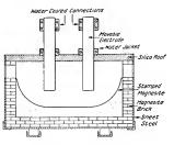
Fig. 6. Cross Section of Single-phase Furnace. Current arcs from one electrode to bath and up to other electrode
