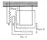
ning above synchronous speed, the ampereturns of the primary winding arc equal to the sum of the ampere-turns of both the regulating and the secondary winding, hence in order not to have the primary winding overheat when running above synchronous speed, it is better to make the cross-section of the regulating winding. As  $AU = (1 - e^2 E_t,$ the reactance  $(x_0 + x_1)$  is found by an impedance test applying  $E_t$  to the slip rings
