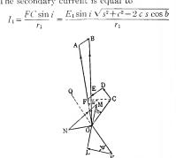
Fig. 17. Running as Motor below Synchronous Speed-Brush Shift Opposite to Direction of Rotation
