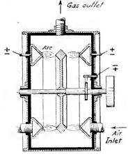
Fig. 1 The Island Furnace with Mechanically Rotated Arc
