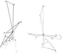
Fig. 20. Running as Motor Above Synchronous Speed Brush Shift in the Direction of Rotation
