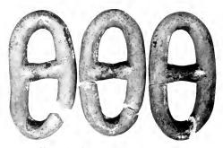
Fig. 10. Two-inch Electric Cast-steel Links Made at Schenectady and Tested at the Charleston Navy Yard
