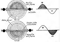
Fig. 3. Alternating Arc Flame of Birkeland-Eyde Furnace
