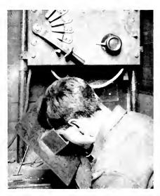
Fig. 8. Proper Distance at which to Hold the Electrode from the Work Electrode from the Work Booths and Various Types of Welding Equipment in use at the Emergency Fleet Corporation Welding School at Schenectady, N. Y.
