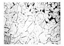
Fig. 4. Electrolytic Iron. Nitrogenized by annealing in  $NH_3$  I2 hrs. 750 deg. C., but subsequently annealed in vacuum for 2 hrs. at 1000 deg. C. Areas smaller and lines diminished in number
