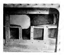
Fig. 2. Another View of Main Engine Casting shown in Fig. 1. The hole in the cylinder wall was cut through to facilitate welding the steam port wall.
