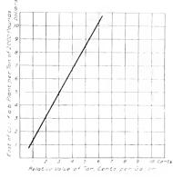
Fig. 12. Curve Showing Approximately the Heating Value of Tar as a Boiler Fuel
