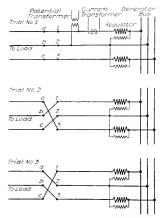
Fig. 21. Connections of Two Single-phase Automatic Induction Regulators on a Three-phase Three-wire System
