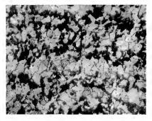
At weld, showing ferrite grain, with form  $\epsilon \rightarrow 0.3$   $^{++}$   $150~{\rm diameters}$
