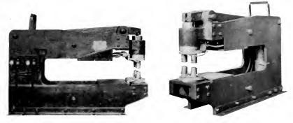
Figs. 6 and 7. Views of Duplex Electric Welder having a Reach of 6 ft. Welds two spots at a time
