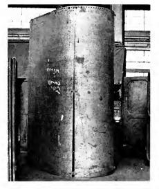
Fig. 1. Appearance of a Long Seam Ready for Welding. Note the bevel of the plate edges, the V shape of the seam, and the method of clamping
