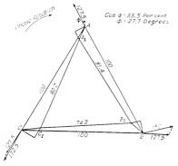
Fig. 19. Vector Diagram Three-phase Feeder, Clockwisephase Rotation
