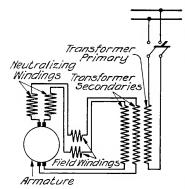
Fig. 1. Diagram of a Two-circuit Series Motor connected to a transformer having two secondary coils,
