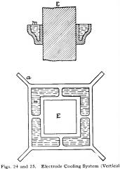
Figs. 24 and 25. Electrode Cooling System (Vertical and Horizontal Cut)
