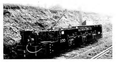
Fig. 15. 30-ton, 48-inch Gauge Mine Haulage Locomotive
