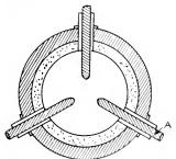
Fig. 5. Cylindrical Electrodes of Small Diameter (80 mm.) (3.15 in.) Used in a Three-phase Stassano Furnace
