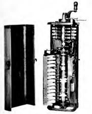
Series-parallel Controller for Use on the Light-weight Car
