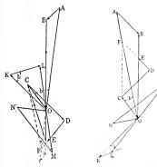
Fig. 18. Driven as Generator Above Synchronous Speed —Brush Shift Opposite to Direction of Rotation Fig. 19. Running as Motor Below Synchronous Speed — Brush Shift in the Direction of Rotation
