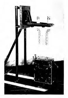
Fig. 8. High-speed, Oil-cooled Fuse Holder Used in Test
