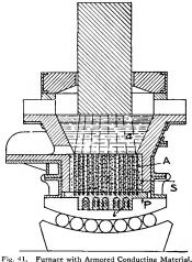
Fig. 41. Furnace with Armored Conducting Material, Keller System
