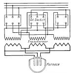
Fig. 9. Connection Diagram of 3-phase Furnace Arranged for Variable Voltage Operation by Means of Changing Highvoltage Connections. The high metting voltage is obtained by connecting high-voltage windings delta and the low refining voltage by connecting them Y
