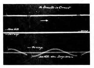
Fig. 1. Oscillogram of a Surge Discharge as in Fig. 2 with no Arrester in Circuit Top vol-rator—current through transformer Bottom vibrator—curcuit voltage
