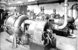
Fig. 6, a and b General Electric Turbine driven Centrifugal Exhausters These units are used to draw the gas through the primary coolers and force it through the ammonia and crude benzol scrubbers
