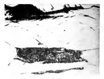
Fig. 5a. Nitride Areas in Electrolytic Iron Treated as in Fig. 3
