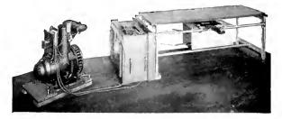
Fig. 4. Complete Portable Roentgen-ray Outfit
