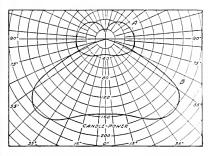
Fig. 12. The Area of a Distribution Curve is not a Criterion for Judging Light Output. These Two Curves Represent Equal Light Outputs
