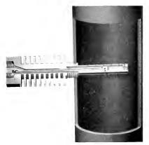
Fig. 1. Sectional View of Nozzle Plug Installed in Pipe
