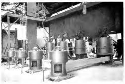
The Pulverizers, which are grinding to the rock in this instal a tion, are of a type most commonly used for pulverizing coal
