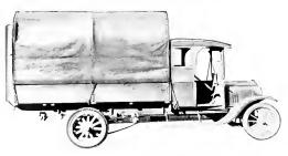
Fig. 2. Automobile Electric Kitchen with Regulation Army Type Canvas Covering in Position
