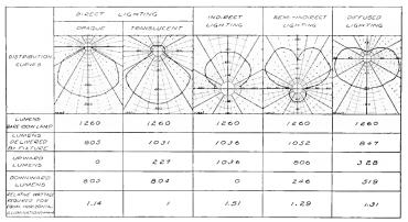
Fig. 2. Characteristics of Lighting Systems
