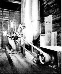
Lead-covered Sulphur Gas Fan Driven by Electric Motor, which has operated without stopping for the last five years at a New England Chemical Company
