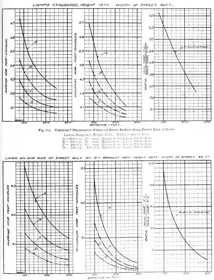
Fig. 3-d. Same as Fig. 3-2, except timps are arranged parallel instead of staggered
