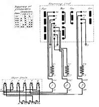
Fig. 7. Simplified Connections of Three-motor Controller
