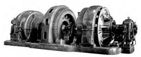
Fig. 9. 2000-kw., 3000-volt, Direct-current Synchronous Motor-generator Set Before Assembly of Flash Barriers
