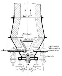
Fig. 6. Modification of Pauling Design Due to Pfachler and Heckenbleckner
