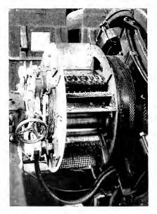
Fig. 19. Final Development of Flash Barriers on 300 kw., 25 cycle, 600-volt Synchronous Converter
