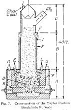
A, Hearth; B, Shaft; C, Head; D, Charge of charo-d; E, Opening for feeding broken carlom to serve as conductor; F, Sulphur; H, Opening for conducting off carbon bisulphide gas; J, Annular space fibed with sulphur; K, Carbon electrodes.
