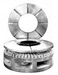
Fig. 1. Spring Thrust Bearing for Vertical Waterwheel Driven Generator to carry a load of 300,000 lb. at 100 (r.p.m. showing rubbing surface of rotating ring. Stationary ring is raised to show the arrangement of springs.
