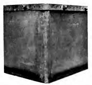
Fig. 6. Note Corner Seam of Tank that was Welded Inside and Outside. The rnised portion of the outside weld was ground off to make a smooth corner as the tank was after ward to be nickel-plated
