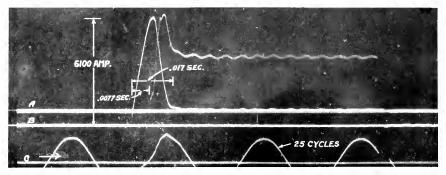
Fig 11. Short Circuit on 300-kw, 600-volt, 25-cycle Synchronous Converter Protected by Air-cooled, High-speed Fuse Curve A, voltage across fuse, Curve B, line current, Curve C, collector-ring voltage
