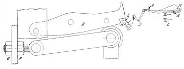
Fig. 3. Sketch showing Tripping Mechanism of High-speed Circuit Breaker
