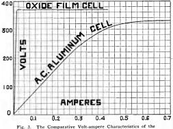
Fig. 3. The Comparative Volt-ampere Characteristics of the Oxide Film Cell and the A-c. Aluminum Arrester Cell. The oxide film has only a few milliamperes of leakage current up to the critical film voltage when the film gives way more suddenly than the film in the aluminum cell. The critical voltage of the oxide film can be made approximately as low as the hydroxide film on the aluminum cell.
