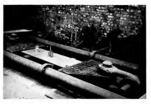
Fig. 1a. Method Employed to Measure Modulus of Elasticity
