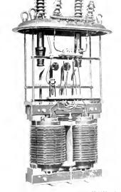
Fig 7. 60-cycle, 1350 kv-a., 36,000 62,400 Y 2400-volt Cylindrical-lisk Type Transformer Showing Method of Bringing Out Leads from Resistance Unit Embedded in Low-voltage Col
