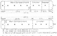
Fig. 5. Installation of Lighting Units on Interurban Cars
