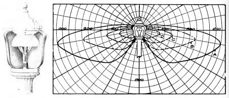
Fig. 3-b. Initial Distribution of Candle-power in a Vertical Plane of the Unit shown in Fig. 3-a Curves A, B, C, and D correspond to the lamps named in Figs. 3-c and 3-d
