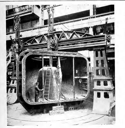
EXHAUST SHELL OF A 45,000-KW. CURTIS TURBINE ON A 40 FT BORING MILL. THE FUEL SITUATION DIRECTS ATTENTION TO THE EFFICIENCY OF THE MODERN TURBINE WITH HIGH STEAM PRESSURE AND SUPERHEAT. See page 216
