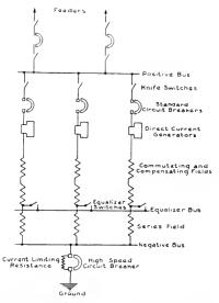
Fig. 10. Diagram of Direct-current Connections for Substation Equipped with Three Motor generator Sets Protected by One High speed Circuit Breaker Connected Across Limiting Resistance
