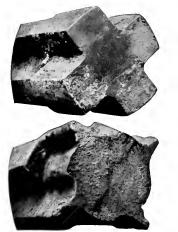
Fig. 2. Worn Steel Roll Wobbler Repaired by Carbon Arc Welding
