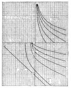
Fig. 5. Speed-torque Curve showing Hoisting and Lowering Control for Cargo Winches
