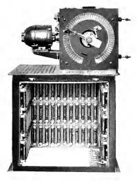
Fig. 4. Motor-operated Rheostat
