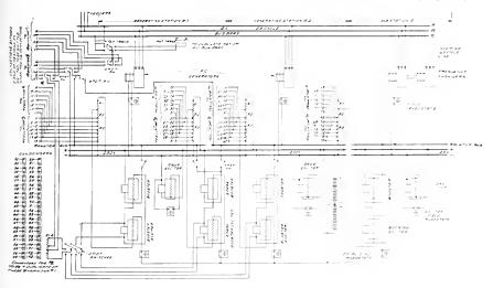
Fig. 3. Complete Wiring Diagram of Regulator System
