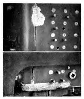
Fig. 5. Worn Outside Sheet of Mud Ring and Reinforcement where Rubbed by Spring Hangers
