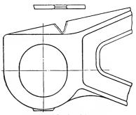
Fig. 13. Cracked Cast Steel Side Truck Frame Prepared for Electric Welding
