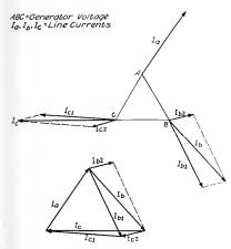
Figs. 11 and 12. Current Diagram of Three-phase Feeder.
