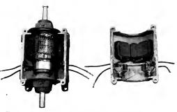
Fig. 4. Motor with Top Half of Frame Removed. Interior of motor easily inspected, two main poles, and one commutating pole in each half of frame
