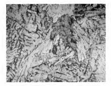
At weld, showing mass of ferrite irregular in shape with a few bands of carbide. 150 diameters.
