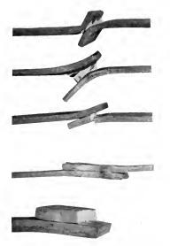
4. Test of Samples 12-inch and 1-inch Thick showing Tear-ing Action when a Single Row of Welded Spots is Used and the Jaws of the Testing Machine are Offset to Accommodate the Displacement. It is, therefore, obvious that, as with rivets, more than one row of spots should be used. Fig. 4.
