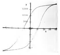
Fig. 3. Photograph of the Normal Hysteresis Loop for Sample Pl
