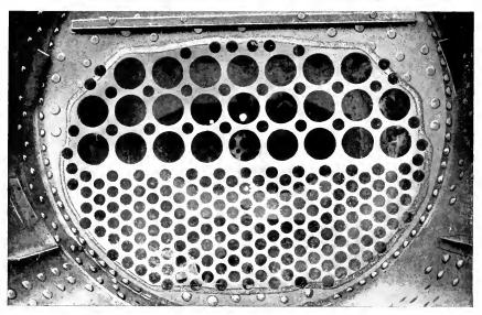
Fig. 2. Front Flue Head Welded in by Arc Process
