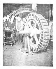
3. Instruction in Testing Rotor of Alternator
