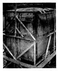
Fig. 23. Electrically Welded Box Constructed for Experimental Purposes for the Electric Welding Committee of the Emergency Flect Corporation. Box Under a Hydrostatic Pressure Test of 40 lb. Per Square Inch. Note bulging of plates
