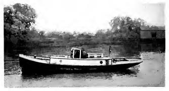
Fig. I. Side View of Electrically Welded Boat
