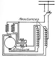
Fig. 2. Diagram of a Two-circuit Series Motor using reactance to limit the flow of current between adjacent brushes
