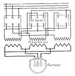
Fig. 28. Connection Diagram of 3-phase Furnace Arranged for Variable Voltage Operation by Means of Changing Highvoltage Connections. The High Melting Voltage is Obtained by Connecting Highvoltage Windings Delta and the Low Refining Voltage by Connecting Idem "Y"
