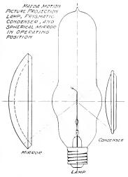
Fig. 83. Diagram of Optical System
