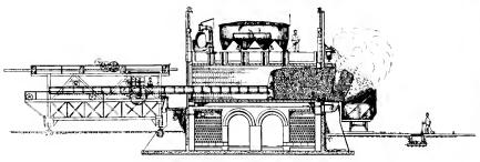
Fig. 3. Conventional Illustration of Coke being Discharged from a By-product Coke Oven This also shows a longitudinal section of a regenerator type of oven
