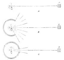
Fig. 2. The Candle-power in the Direction of the Photo.neter is Not Changed by Partially Surrounding the Light Source With a Non-Reflecting Surface
