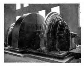
Fig 33. Flywheel Motor-generator Set for Power Supply of Reversing Mill Motor, Shown in Fig. 31, 2000-h.p., 360-r.p.m., 2300-volt Motor. 2000-kw., 360-r.p.m. Generator, 100,000 lb. Flywheel, Ashland Iron Mining Company, Ashland, Ky.
