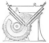
Fig. 3. Continuous Type Calcium Carbide Furnace
