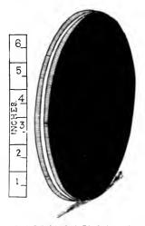
Fig. 1 A Single Cell of the Oxide Film Lightning Arrester consisting of a ning of porcelain with two circular steel disks, one spun on each side of the porcelain and insulated by the porcelain. The inside of the ring of porcelain between the plates is filled with peroxide of lead.
