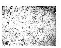
Fig. 8. Section of Weld Made with Pure Electrolytic Iron in Nitrogen Gas
