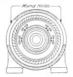
Fig. 9. Mechanical Arrangement of Brush Studs on a two-circuit series motor
