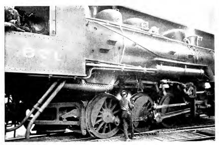
Fig. 9. Filling in Worn Flange on Locomotive Driving Wheel
