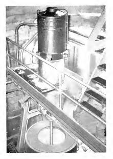
Motor-driven Centrifugal in Bicarbonate of Soda Department, Solvay Process Company, Syracuse, N. Y.
