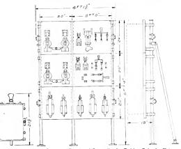
Fig. 38. Outline of Contactor Panel and Controller for Rubber Calender Drive
