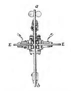
Fig. 3 Girard and Street Type of Furnace Used for the Manufacture of Graphitic Electrodes
