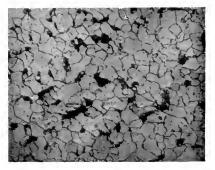
At weld, showing ferrite grains with a few areas of pearly = Carbide absent. 150 diameters.
