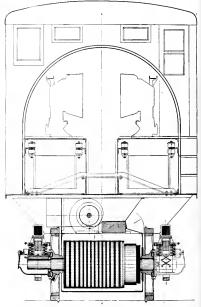
Fig. 2. End Elevation of Chicago, Milwaukee & St. Paul Locomotive Showing Location of Armature and Control Equipment
