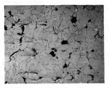
At weld, showing ferrite grains with a few dots of pearlite. Carlide absent. 150 diameters.
