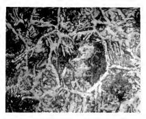
Close to weld, showing sorbitic grains surrounded by irregular bands of territe = 150 diameters.
