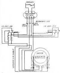
Fig. 8. Diagram of Connections of a Series Motor showing arrangement of current-limiting resistance
