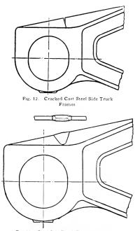
Fig. 14. Steel Side Truck Frame Prepared for Electric Welding
