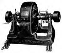
Fig. 3. 4-pole, 10-kw., 1800-r.p.m., 110-volt Shunt-wound Synchronous Converter
