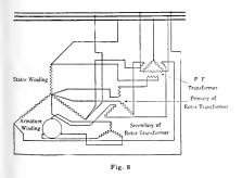
speed is required. For instance, if it is desired to regulate the speed 25 per cent below and 25 per cent above the synchronous speed, the capacity of the transformer is equal to only 25 per cent of the kilovolt amperes flowing through the motor. The characteristics can be improved by adding a small transformer to shift the time-phase of the voltage impressed on the primary of the rotor transformer.
