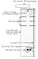
Fig. 1 Diagram showing Arrangement of Measuring Apparatus
