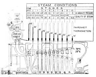
Fig. 2. Section of Ten-stage Turbine, showing Condition of Steam in Each Stage
