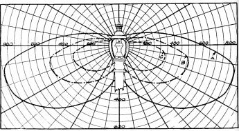
Fig. 4-a Ornamental Novalux Unit with 8-panel Stippled Glass Globe and Dome Refractor
