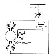
Fig. 3. Diagram of a Two-circuit Series Motor having four neutralizing coils
