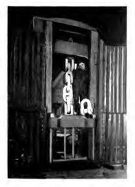
Fig. 7. 3 ,-in Naco Anchor-chain Links in a Static Testing Machine, National Malleable Castings Co-
