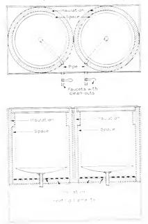
Fig. 3. Plan and Elevation of Fireless C soker Compartment
