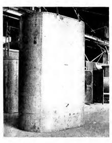
Fig. 3. A Finished Weld of a Long Seam. Note the uniformity in width and appearance of the weld
