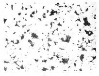
Fig. 10. Section of Weld Made with Pure Electrolytic Iron in CO: Gas
