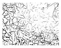
Fig. 3. Electrolytic Iron. Nitrogenized by annealing in NH<sub>3</sub> 12 hrs. 750 deg. C.
