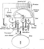
Fig. 4. Diagrammatic Sketch of Alternating-current Demand Meter (Type a)
