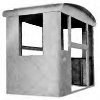
Fig. 1. Electrically Welded Locomotive Cab
