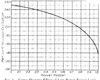
Fig. 5. Curve Showing Effect of Low Power Factor Load on Generator Excitation
