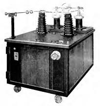
Fig. 45. High-voltage, Portable Direct-current Cable Testing Set
