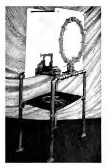
Fig. 7. High-speed, Air-cooled Fuse Holder with Magnetic Blow-out Used in Test
