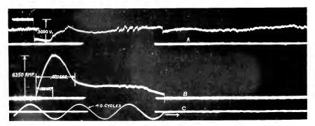
Fig. 6 Direct current Short Circuit on 2000-kw, 2000 volt, Motor-generator Set with High-speed C.rcuit Breaker and Standard 2000-volt Switchboard Type Circuit Breaker
