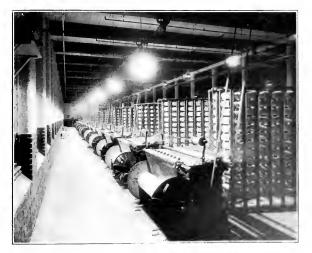
Fig. 1. Night Photograph of a Row of Warpers Well Illuminated by 75-watt Mazda C Lamps in Deep Bowl Steel Reflectors Hung Over the Beam and the Creel. Work under such can be carried on effectively, independent of daylight condutions. With good illuminations, the shop is perforce clean and safe. Employees are contented and production is kept at a maximum
