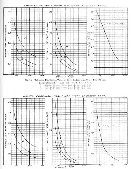
Fig. 4-d. Same as Fig. 4-c, except lamps are arranged parallel instead of staggered
