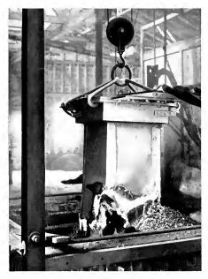
Fig. 4 Photograph taken shortly after 20-inch square carbon electrode had broken on a single-phase Ferro-silcon Furnace
