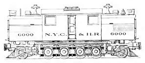
Ft 7. Latest Type New York Central Locomotive Equipped with Eight Bipolar Gearless Motors
