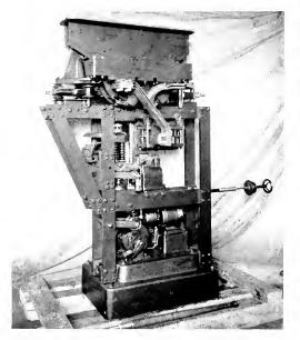
Fig 4 3000-ampere, 3600-volt, Direct-current, High-speed Circuit Breaker
