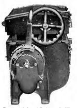
Fig. 17. HC Control Equipment for Mine Locomotive Showing Location of Hand Lever
