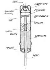
Fig. 9. Construction of Vacuum Tube Lightning Arrester
