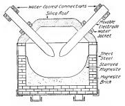
Fig. 19. Cross Section of Single-phase Stassano Furnace. Current arcs between electrodes and bath is heated by radiation
