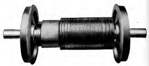
Fig. 6. Wheels and Armature of Bipolar Gearless Motor
