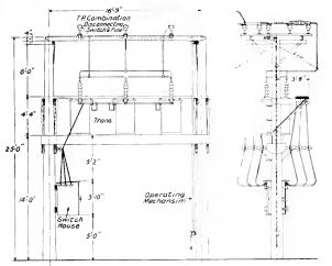
Fig. 2. Standard Outdoor Substation, pole-mounted, three-phase, 45,000 volts maximum high tension, 2300 volts maximum low tension, 150 kv-a. maximum
