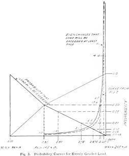
Fig 3. Probability Curves for Evenly Graded Load. Average is 0.3 of Range
