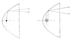
Fig. 5. Increasing Spread of Beam from parabolic reflector due to increasing size of light source
