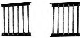
Fig. 1. Front and Back Views of Grating Constructed on Spot Welding Machine
