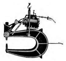
Fig. 1. A Standard Type of Pneumatic Riveter
