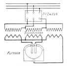
Fig. 25. Connection Diagram of Greaves-Etchells Furnace. Current arcs from two movable electrodes to bath and thence to lower electrode
