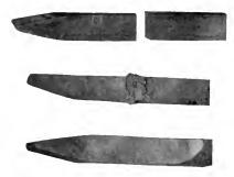
Fig. 7. Electrically Butt-welding High Speed Cutting Face to Machine Tool Shank
