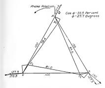
Fig. 18. Vector Diagram of Three-phase Feeder, Counterclockwise Phase Rotation
