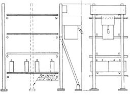
Fig. 6. Method of Mounting Condenser Section
